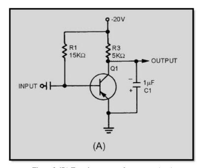
Figure 3-47A Transistor sawtooth generator (pnp)
