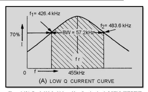
Figure 1-12A. Bandwidth for high- and low-Q series circuit. LOW Q CURRENT CURVE
