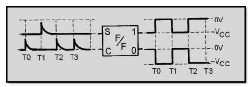
Figure 3-27 Flip-flop with trigger pulse on SET and inputs
