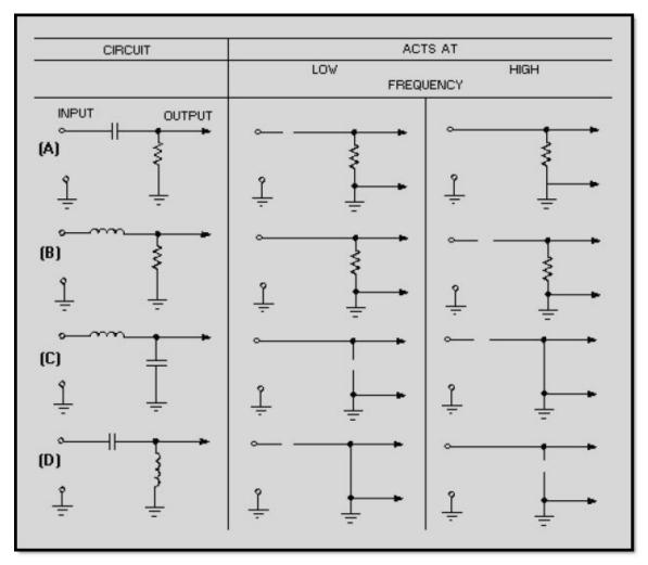
Figure 1-14 Reaction to circuit by change in frequency
