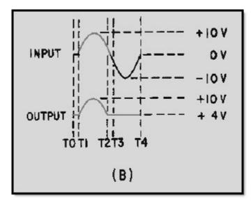
Figure 4-14B.—Parallel-negative limiter with positive bias
