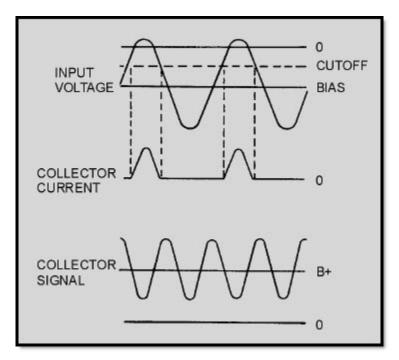
Figure 2-27 Frequency doubler waveforms
