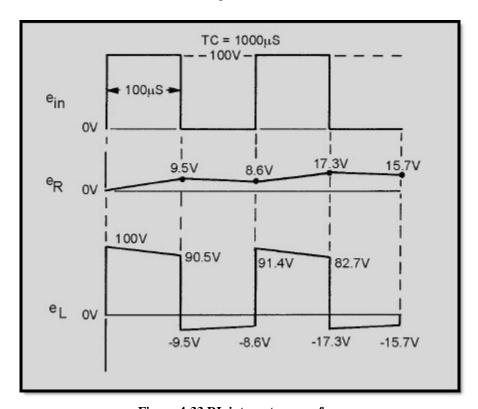
Figure 4-33 RL integrator waveform
