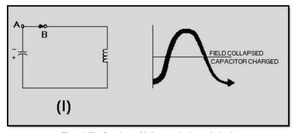
Figure 1-8I.—Capacitor and inductor action in a tank circuit
