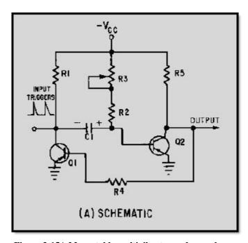
Figure 3-15A Monostable multivibrator and waveshapes. Schematic
