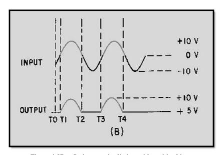
Figure 4-8B.—Series-negative limiter with positive bins
