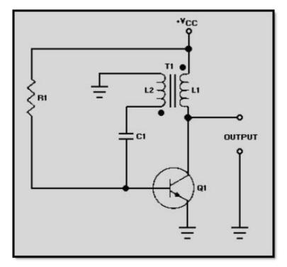
Figure 3-33 Blocking oscillator
