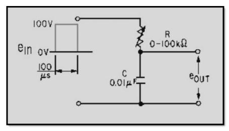
Figure 4-35 RC integrator circuit
