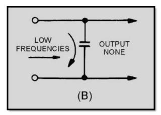
Figure 1-16B.—Components of a simple lowpass filter
