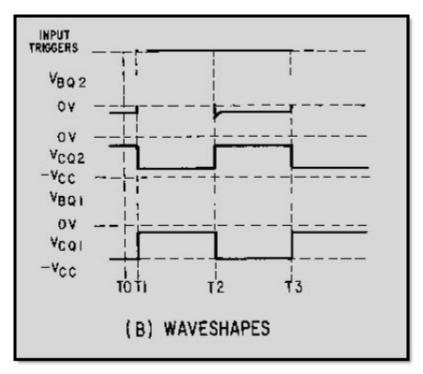
Figure 3-15B.—Monostable multivibrator and waveshapes. Waveshapes
