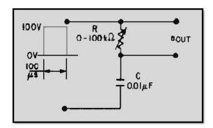
Figure 4-39 RC circuit as a differentiator
