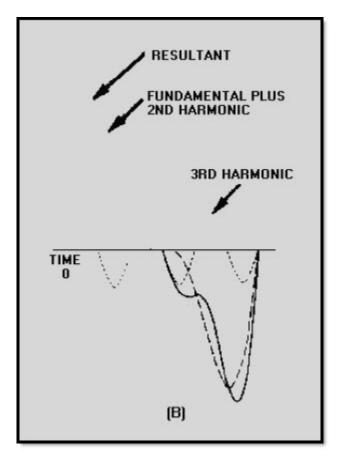
Figure 4-26B.—Composition of a sawtooth wave
