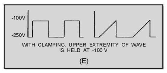
Figure 4-16E.—Clamping waveforms. WITH CLAMPING, UPPER EXTREMITY OF
