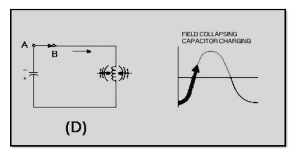
Figure 1-8D.—Capacitor and inductor action in a tank circuit
