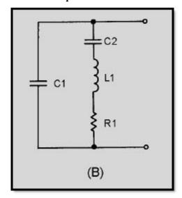
Figure 2-20B.—Quartz crystal and equivalent circuit
