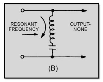
Figure 1-22B.—Components of a simple bandreject filter
