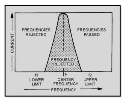
Figure 1-21 Band-reject filter response curve
