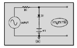
Figure 4-11A Parallel-positive Limiter with positive bias
