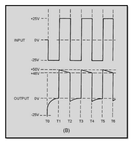
Figure 4-18B.—Positive damper and waveform
