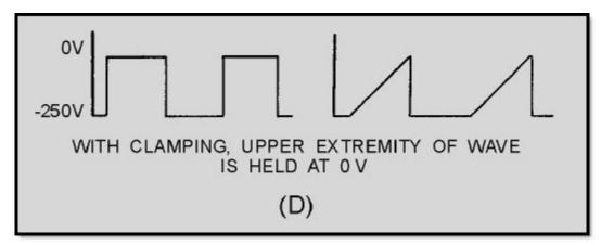
Figure 4-16D.—Clamping waveforms. WITH CLAMPING, UPPER EXTREMITY OF
