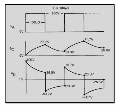
Figure 4-41 Voltage outputs in a medium time-constant differentiator
