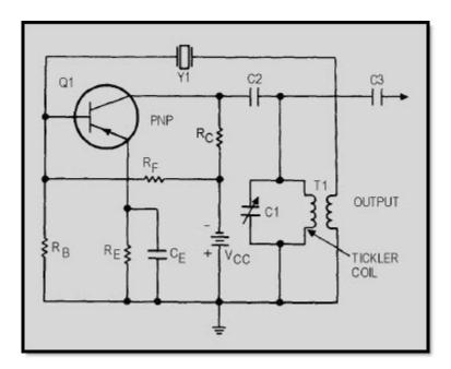
Figure 2-22 Crystal-controlled Armstrong oscillator
