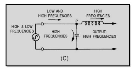
Figure 1-16C.—Components of a simple low-pass filter
