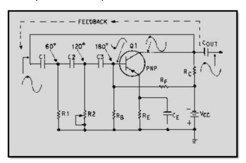
Figure 2-17 Phase-shift oscillator
