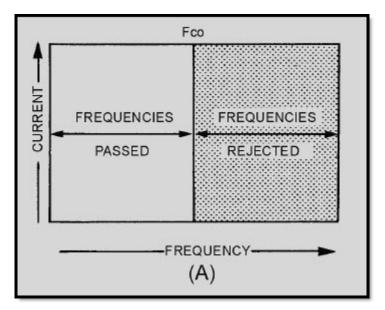
Figure 1-15A. Low-pass filter
