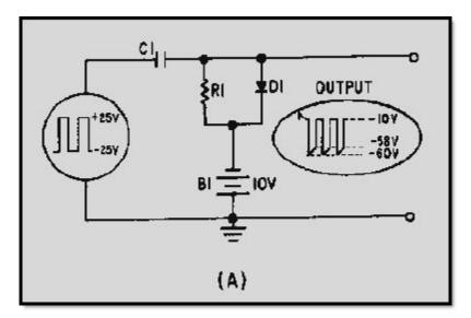
Figure 4-22A Negative damper with negative bias
