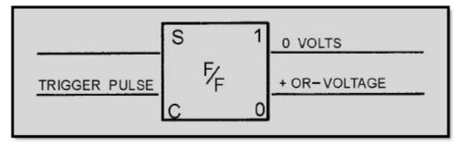
Figure 3-26 Flip-flop (CLEAR state)
