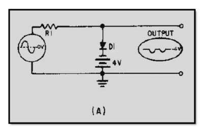
Figure 4-10A Parallel limiter with negative bias
