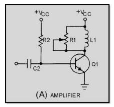
Figure 2-10A Basic Armstrong oscillator circuit. AMPLIFIER
