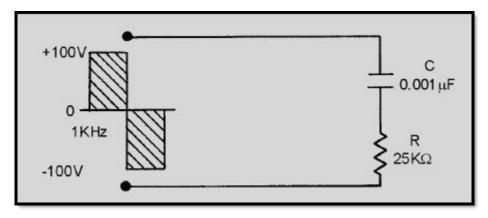
Figure 4-30 Partial integration circuit
