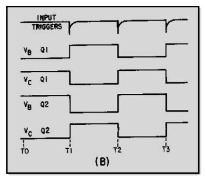
Figure 3-17B.—Bistable multivibrator and waveforms
