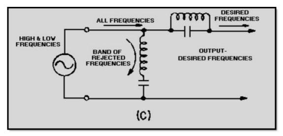
Figure 1-22C.—Components of a simple band-reject filter
