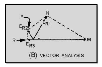
Figure 2-2B.—RC oscillator. VECTOR ANALYSIS
