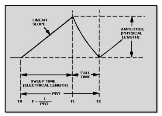
Figure 3-40 Sawtooth waveform
