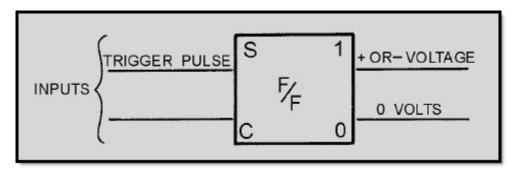
Figure 3-25 Flip-flop (SET state)
