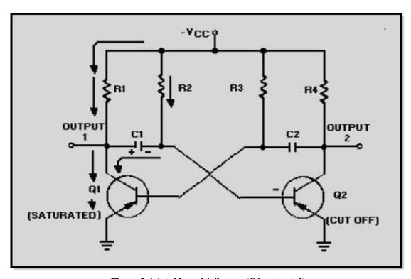
Figure 3-4 Astable multivibrator (Q1 saturated)
