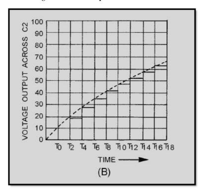
Figure 4-45B.—Basic step counter and waveforms
