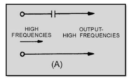
Figure 1-18A. Components of a simple high-pass filter
