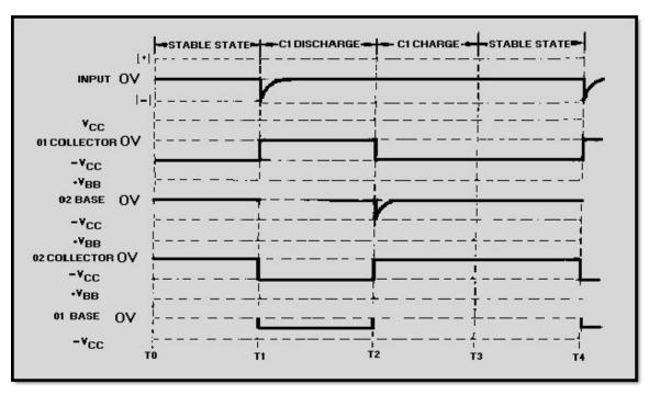
Figure 3-14 Waveforms of a monostable multivibrator (triggered)
