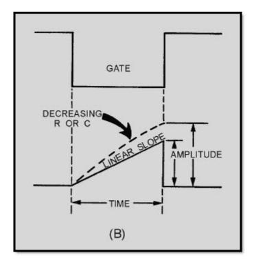
Figure 3-43B.—Relationship of R and C to linearity
