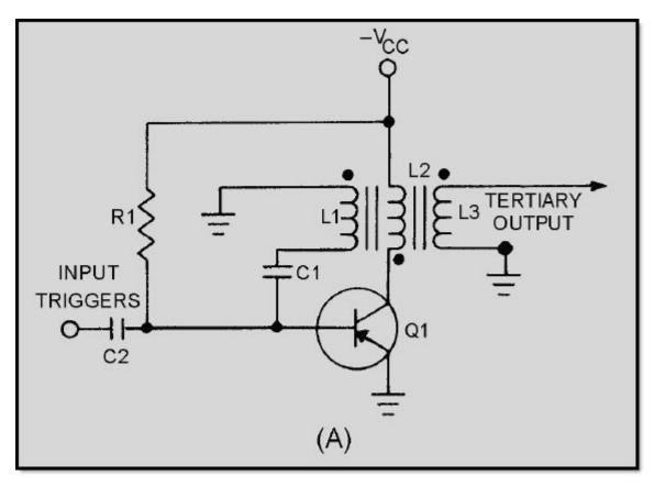
Figure 3-37A Blocking oscillator (synchronized)
