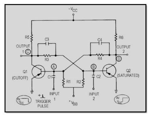
Figure 3-23 Bistable multivibrator (flip-flop)
