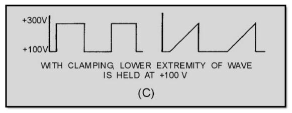
Figure 4-16C.—Clamping waveforms. WITH CLAMPING, LOWER EXTREMITY OF WAVE IS HELD AT  $+100~\mathrm{V}$ .
