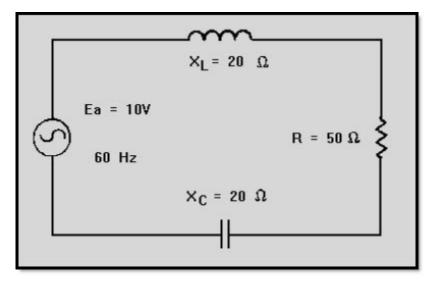
Figure 1-25 Series RLC circuit at resonance
