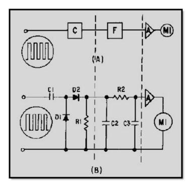
Figure 4-44 Basic frequency counter
