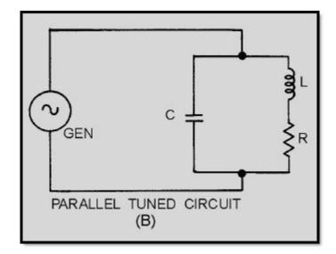
Figure 1-1B.—Basic tuned circuits. PARALLEL TUNED CIRCUIT
