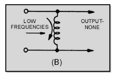
Figure 1-18B.—Components of a simple high-pass filter
