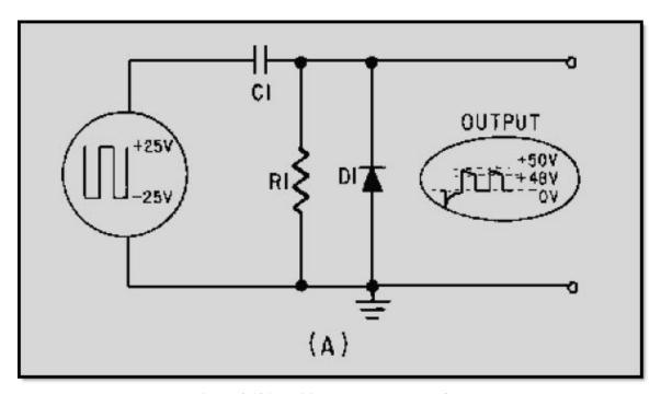
Figure 4-18A Positive damper and waveform
