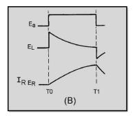
Figure 3-49B.—Series LR circuit
