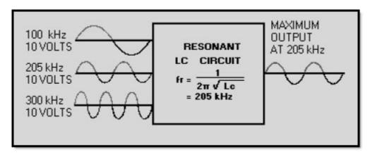
Figure 1-6 Output of the resonant circuit
