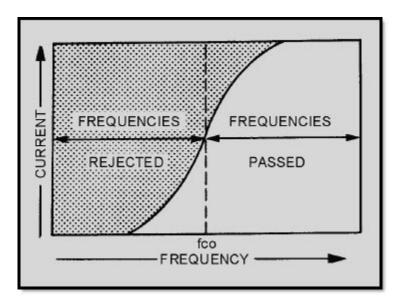
Figure 1-17 High-pass filter response curve
