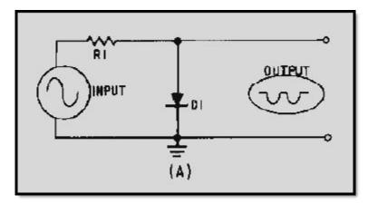
Figure 4-9A Parallel-positive limiter
