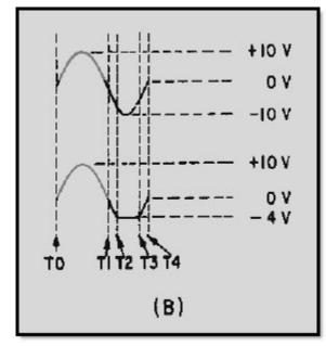
Figure 4-13B.—Parallel-negative limiter with negative bias
