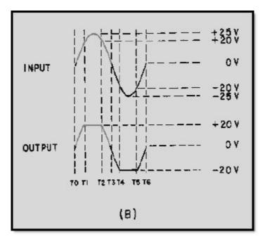
Figure 4-15B.—Dual-diode limiter
