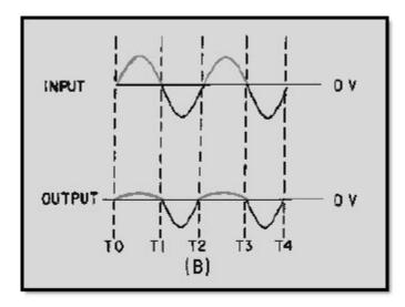
Figure 4-9B.—Parallel-positive limiter
