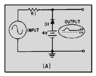
Figure 4-14A Parallel-negative limiter with positive bias
