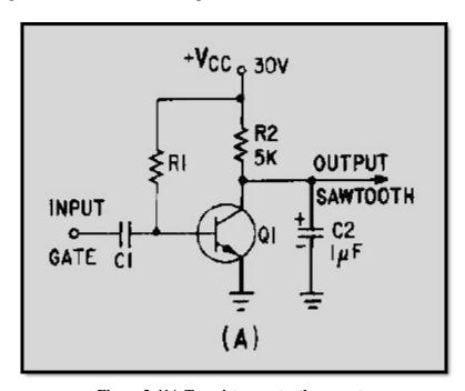
Figure 3-41A Transistor sawtooth generator
