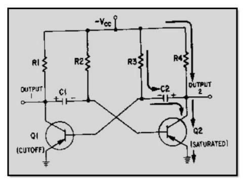
Figure 3-6 Astable multivibrator. (Q2 saturated)
