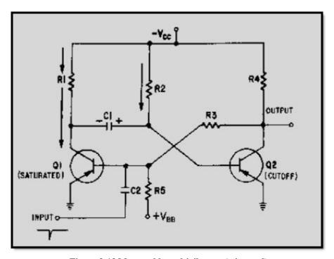
Figure 3-13 Monostable multivibrator (triggered)
