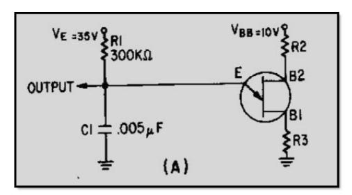
Figure 3-45A Improved unijunction sawtooth generator
