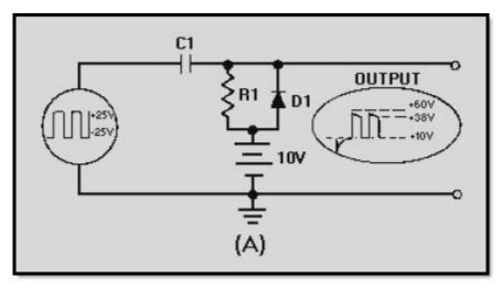
Figure 4-19A Positive clamper with positive bias
