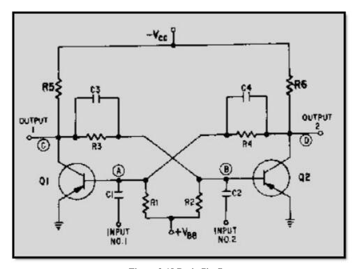
Figure 3-18 Basic flip-flop
