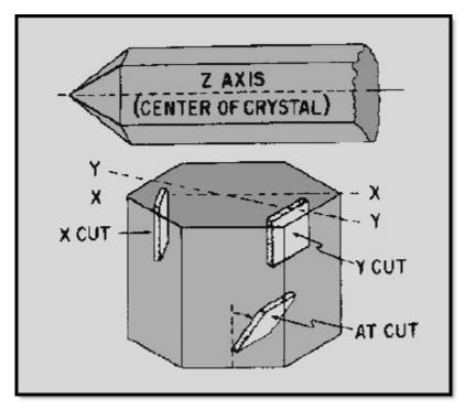
Figure 2-19 Quartz crystal cuts
