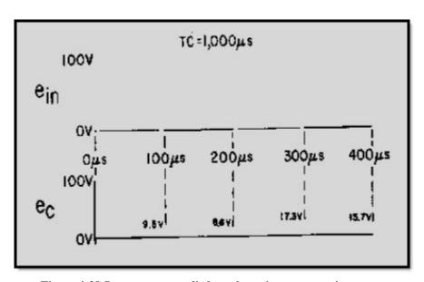
Figure 4-38 Square wave applied to a long time-constant integrator
