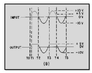
Figure 4-4B.—Series-positive limiter with positive bias
