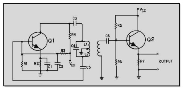
Figure 2-29 Shunt-fed Hartley oscillator with buffer amplifier
