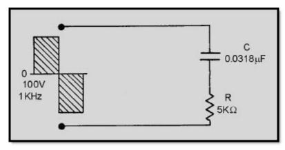
Figure 4-29 Square wave applied to an RC circuit
