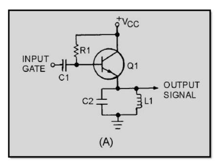
Figure 2-25A Pulsed oscillator
