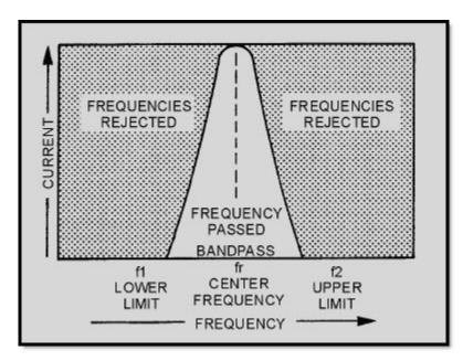
Figure 1-19 Bandpass filter response curve
