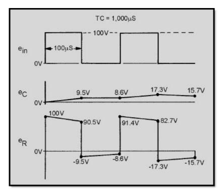
Figure 4-42 Voltage outputs in a long time-constant differentiator
