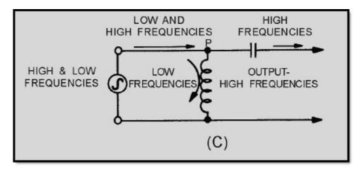
Figure 1-18C.—Components of a simple high-pass filter
