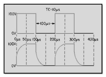
Figure 4-36 Square wave applied to a short time-constant integrator
