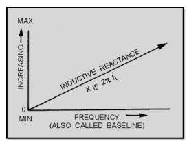
Figure 1-2 Effect of frequency on inductive reactance
