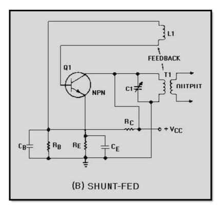
Figure 2-9B.—Series- and shunt-fed, tuned-collector Armstrong oscillators. SHUNT-FED
