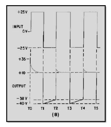
Figure 4-23B.—Negative clamper with positive bias
