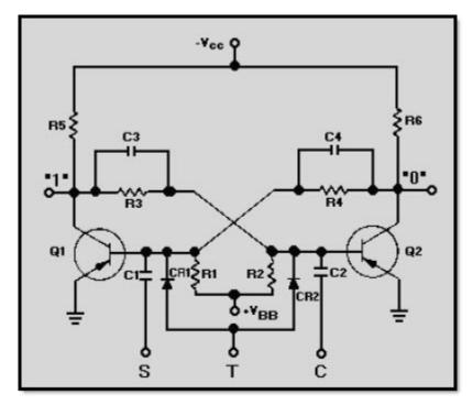
Figure 3-28 Flip-flop with three inputs
