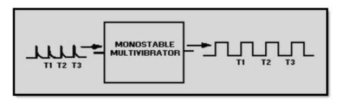
Figure 3-10 Monostable multivibrator block diagram
