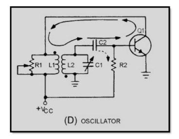
Figure 2-10D.—Basic Armstrong oscillator circuit. OSCILLATOR
