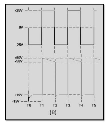
Figure 4-19B.—Positive clamper with positive bias
