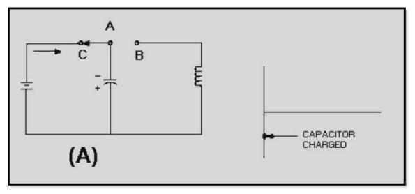
Figure 1-8A. Capacitor and inductor action in a tank circuit
