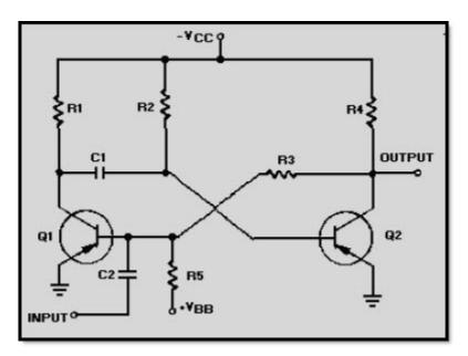
Figure 3-11 Monostable multivibrator schematic
