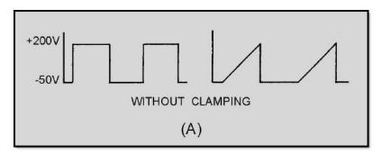
Figure 4-16A Clamping waveforms. WITHOUT CLAMPING
