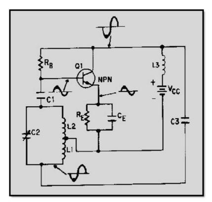
Figure 2-14 Shunt-fed, tuned-base Hartley oscillator
