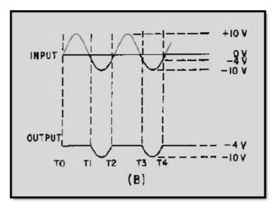
Figure 4-10B.—Parallel limiter with negative bias
