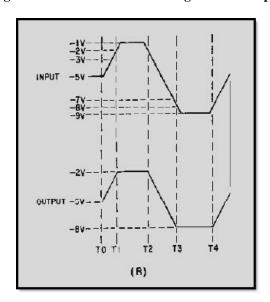
Figure 4-24B.—Common-base configuration clamper
