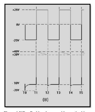
Figure 4-20B.—Positive clamper with negative bias
