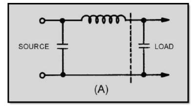
Figure 1-24A. Formation of a -type filter
