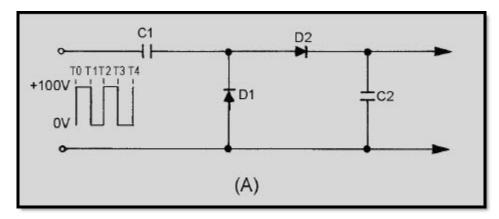
Figure 4-45A Basic step counter and waveforms
