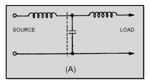
Figure 1-23A. Formation of a T-type filter
