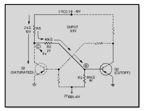
Figure 3-21 Flip-flop (Q2 voltage divider)
