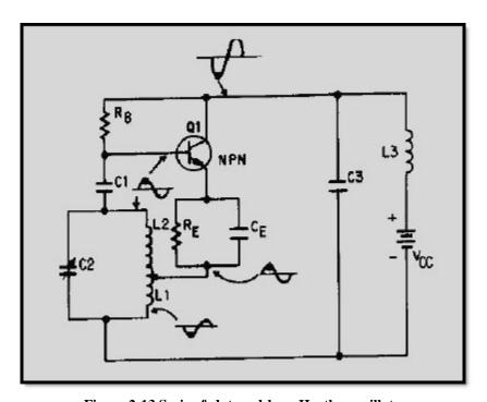
Figure 2-13 Series-fed, tuned-base Hartley oscillator
