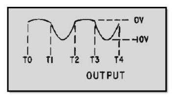
Figure 4-2 Actual output of a series-positive limiter
