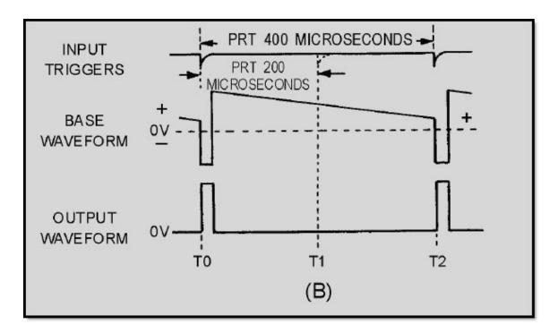
Figure 3-37B.—Blocking oscillator (synchronized)
