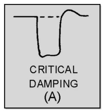
Figure 3-36A Waveform damping. CRITICAL DAMPING
