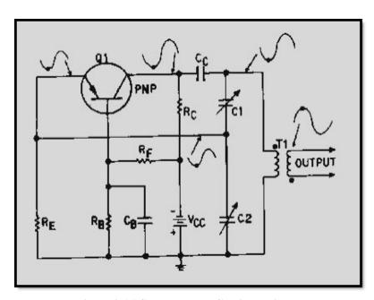
Figure 2-16 Common-base Colpitts oscillator
