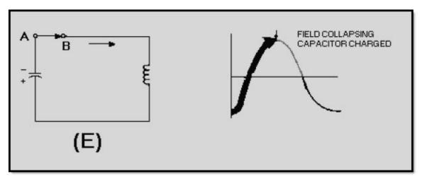
Figure 1-8E.—Capacitor and inductor action in a tank circuit
