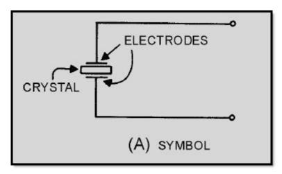
Figure 2-6A Crystal symbol and equivalent circuits. SYMBOL
