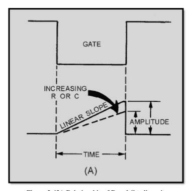
Figure 3-43A Relationship of R and C to linearity
