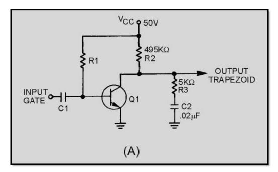
Figure 3-50A Trapezoidal waveform generator
