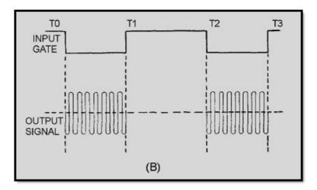
Figure 2-25B.—Pulsed oscillator
