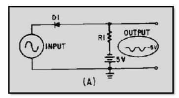
Figure 4-5A Series-positive limiter with negative bias
