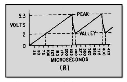
Figure 3-45B.—Improved unijunction sawtooth generator
