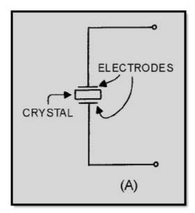
Figure 2-20A.—Quartz crystal and equivalent circuit
