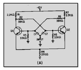
Figure 3-17A Bistable multivibrator and waveforms
