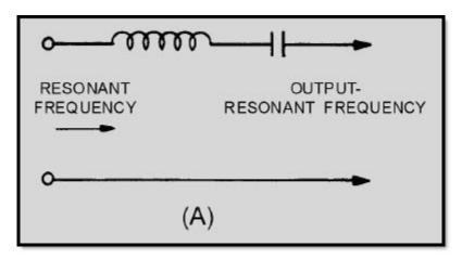
Figure 1-20A. Components of a simple bandpass filter
