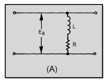
Figure 3-49A Series LR circuit
