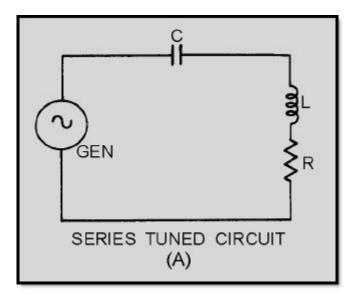
Figure 1-1A. — Basic tuned circuits. SERIES TUNED CIRCUIT
