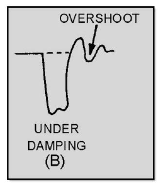
Figure 3-36B.—Waveform damping. UNDER DAMPING.
