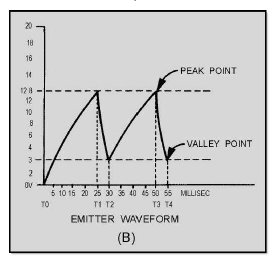
Figure 3-44B.—Unijunction sawtooth generator. EMITTER WAVEFORM
