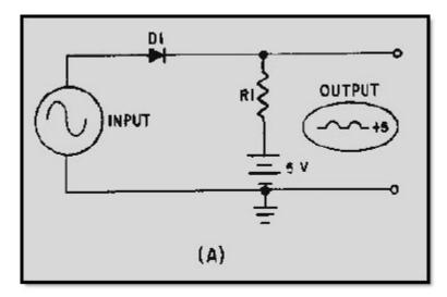
Figure 4-8A Series-negative limiter with positive bins
