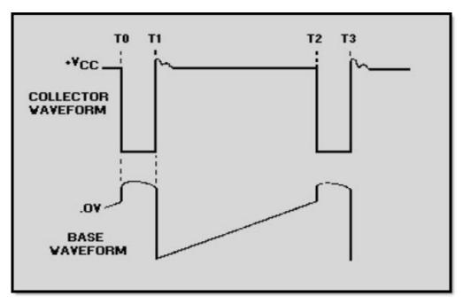
Figure 3-34 Blocking oscillator idealized waveforms
