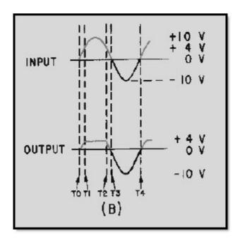
Figure 4-11B.—Parallel-positive Limiter with positive bias
