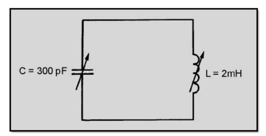
Figure 1-4 Practice tank circuit
