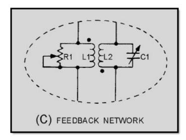
Figure 2-10C.—Basic Armstrong oscillator circuit. FEEDBACK NETWORK
