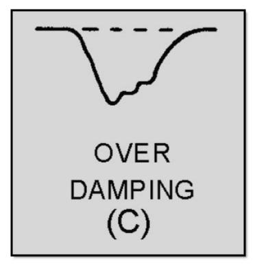
Figure 3-36C.—Waveform damping. OVER DAMPING
