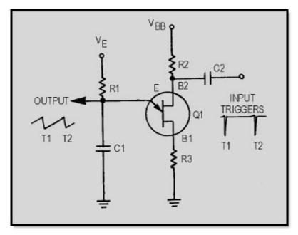
Figure 3-46 Synchronized sawtooth generator
