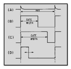
Figure 3-16 Monostable multivibrator waveforms with a variable gate
