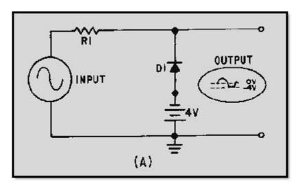
Figure 4-13A Parallel-negative limiter with negative bias
