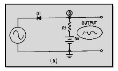
Figure 4-4A Series-positive limiter with positive bias
