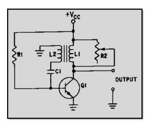
Figure 3-35 Circuit damping
