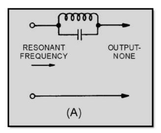
Figure 1-22A. Components of a simple band-reject filter
