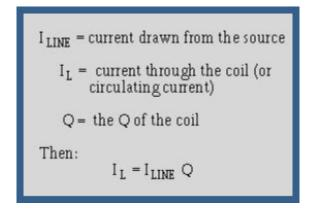
Again, if the Q were 100, the circulating current would be 100 times the value of the line current. This may help explain why some of the wire sizes are very large in high-power amplifying circuits.
