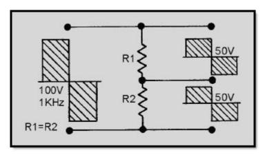
Figure 4-28 Square wave applied to a resistive circuit
