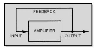
Figure 2-1 Basic oscillator block diagram
