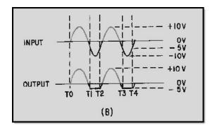
Figure 4-7B.—Series-negative limiter with negative bias
