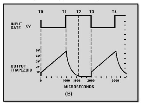
Figure 3-50B.—Trapezoidal waveform generator
