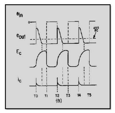
Figure 4-43B.—Positive-diode counter and waveform
