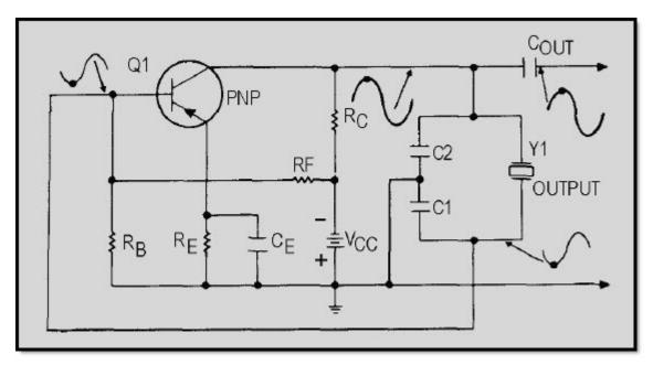
Figure 2-24 Pierce oscillator, common-emitter configuration
