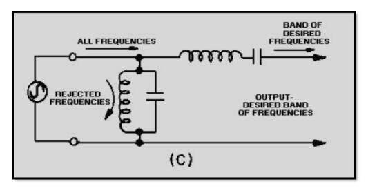
Figure 1-20C.—Components of a simple bandpass filter
