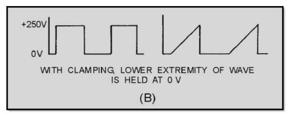
Figure 4-16B.—Clamping waveforms. WITH CLAMPING, LOWER EXTREMITY OF WAVE IS HELD AT 0V
