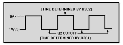
Figure 3-7 Square wave output from Q2
