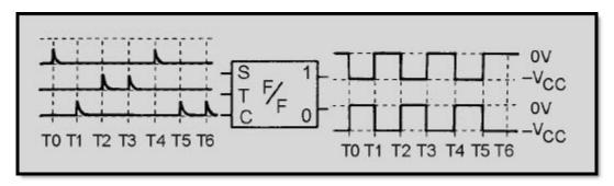
Figure 3-30 Flip-flop with three inputs (block diagram)
