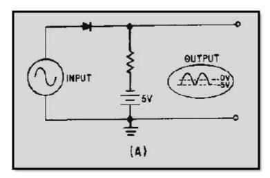
Figure 4-7A Series-negative limiter with negative bias
