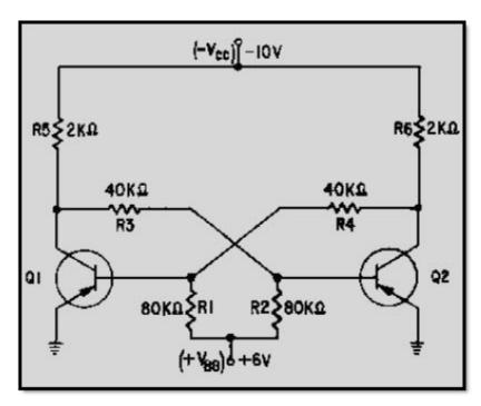
Figure 3-19 Flip-flop (capacitors removed)
