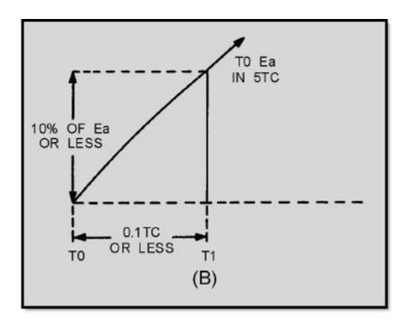
Figure 3-38B.—Series RC circuit
