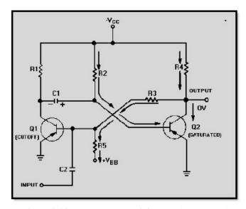
Figure 3-12 Monostable multivibrator (stable state)
