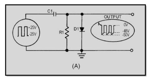
Figure 4-21A Negative clamper and waveform
