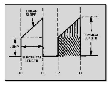
Figure 3-48 Trapezoidal waveform
