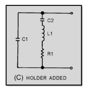
Figure 2-6C.—Crystal symbol and equivalent circuits. HOLDER ADDED
