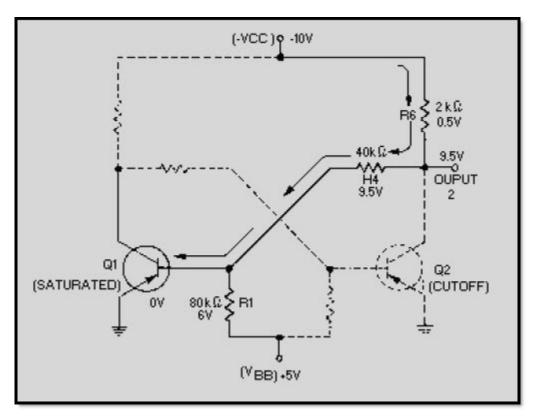
Figure 3-20 Flip-flop (Q1 voltage divider)
