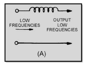
Figure 1-16A. Components of a simple lowpass filter
