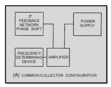
Figure 2-8A.—Basic configurations. COMMON-COLLECTOR CONFIGURATION
