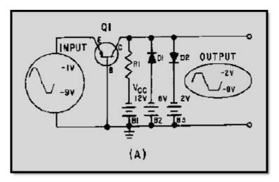
Figure 4-24A Common-base configuration clamper
