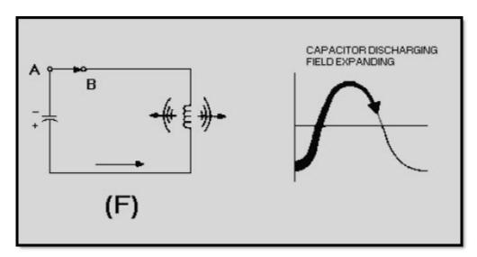
Figure 1-8F.—Capacitor and inductor action in a tank circuit
