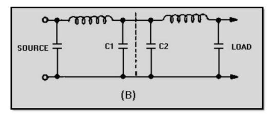
Figure 1-24B.—Formation of a -type filter
