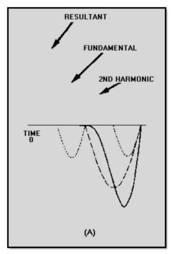
Figure 4-26A Composition of a sawtooth wave
