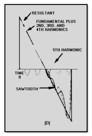
Figure 4-26D.—Composition of a sawtooth wave
