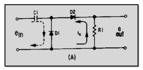
Figure 4-43A Positive-diode counter and waveform
