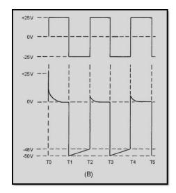
Figure 4-21B.—Negative clamper and waveform
