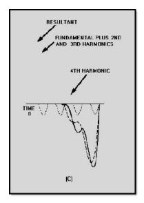
Figure 4-26C.—Composition of a sawtooth wave
