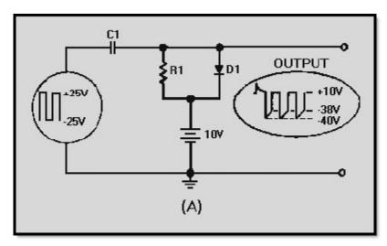
Figure 4-23A Negative clamper with positive bias
