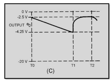
Figure 3-47C.—Transistor sawtooth generator (pnp)
