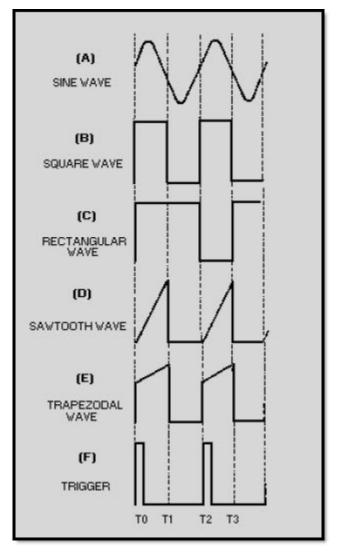
Figure 3-1 Periodic waveforms
