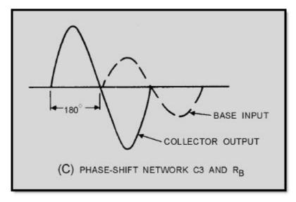
Figure 2-18C.—Three-section, phase-shifting RC network. PHASE-SHIFT NETWORK C3 AND  $R_{\rm B}$
