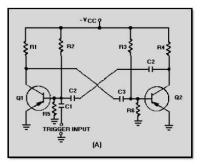
Figure 3-9A Triggered astable multivibrator and output
