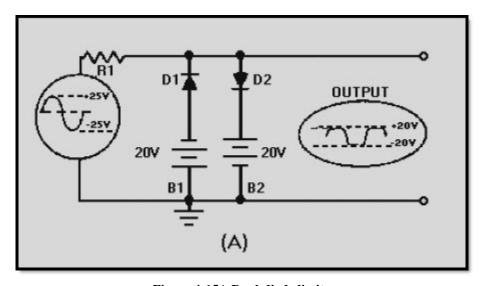
Figure 4-15A Dual-diode limiter
