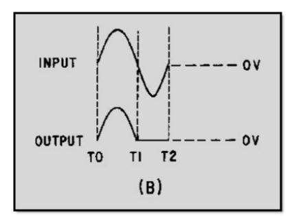
Figure 4-12B.—Parallel-negative limiter
