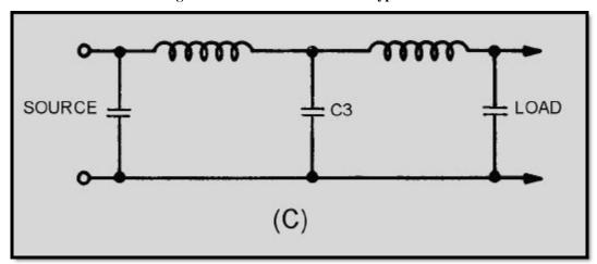
Figure 1-24C.—Formation of a -type filter
