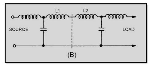
Figure 1-23B.—Formation of a T-type filter
