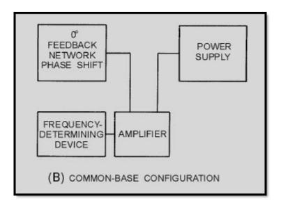
Figure 2-8B.—Basic configurations. COMMON-BASE CONFIGURATION
