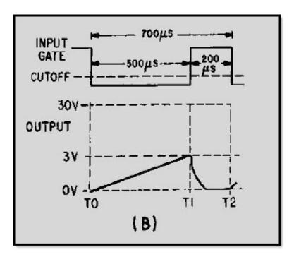
Figure 3-41B.—Transistor sawtooth generator
