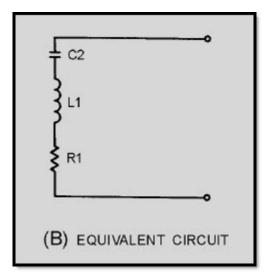
Figure 2-6B.—Crystal symbol and equivalent circuits. EQUIVALENT CIRCUIT
