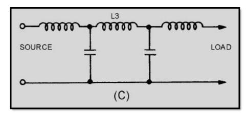
Figure 1-23C.—Formation of a T-type filter
