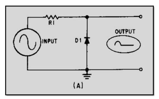
Figure 4-12A Parallel-negative limiter
