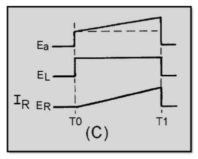
Figure 3-49C.—Series LR circuit
