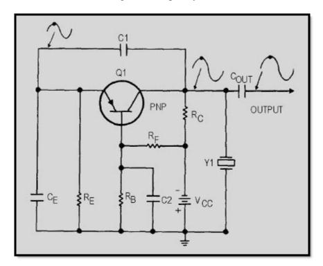
Figure 2-23 Pierce oscillator, common-base configuration
