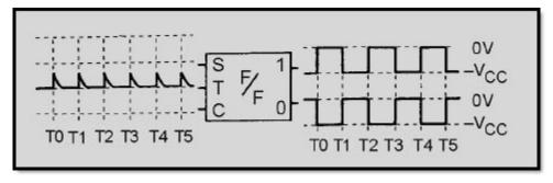
Figure 3-29 Block diagram of a flip-flop with a toggle input
