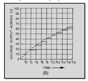
Figure 4-46B.—Step counter as a frequency divider and waveforms
