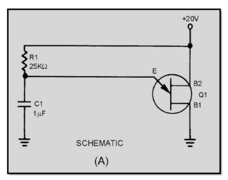
Figure 3-44A Unijunction sawtooth generator. SCHEMATIC
