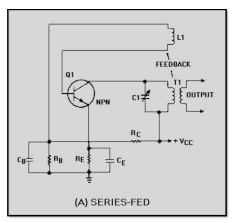
Figure 2-9A Series- and shunt-fed, tuned-collector Armstrong oscillators. SERIES-FED
