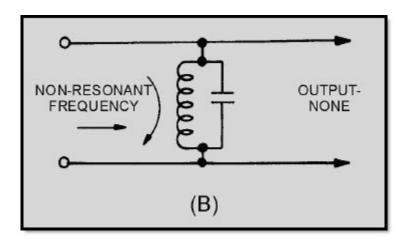
Figure 1-20B.—Components of a simple bandpass filter
