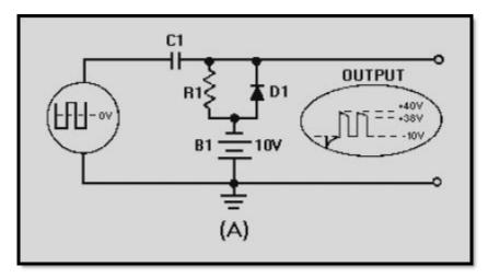
Figure 4-20A Positive clamper with negative bias
