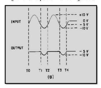
Figure 4-5B.—Series-positive limiter with negative bias
