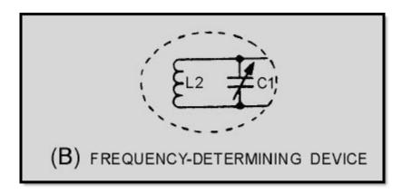
Figure 2-10B.—Basic Armstrong oscillator circuit. FREQUENCY-DETERMINING DEVICE
