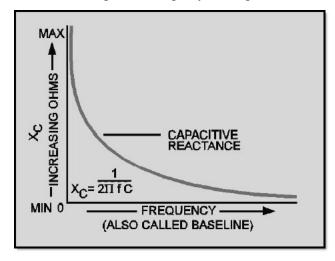
Figure 1-3 Effect of frequency on capacitive reactance
