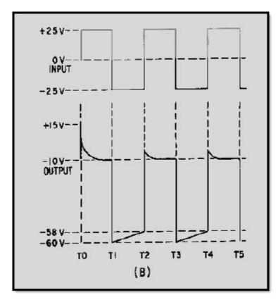
Figure 4-22B.—Negative damper with negative bias
