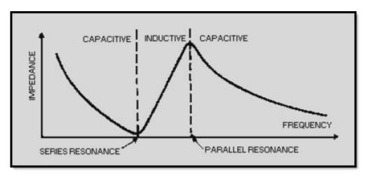
Figure 2-21 Frequency response of a crystal
