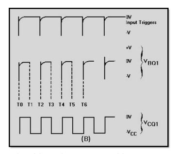
Figure 3-9B.—Triggered astable multivibrator and output
