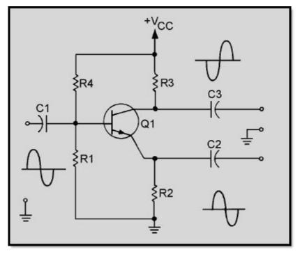
Figure 1-27 Single-stage transistor phase splitter
