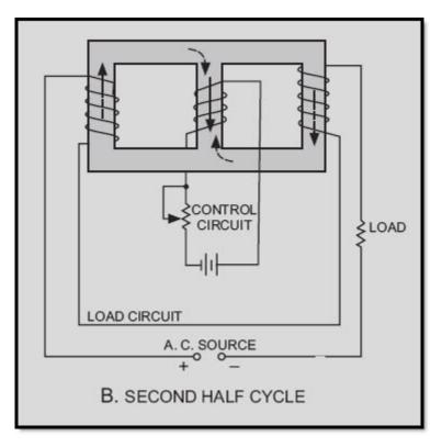
Figure 3-36B.—Three-legged, saturable-core reactor. SECOND HALF CYCLE
