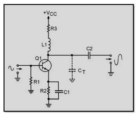
Figure 2-7 Shunt peaking coil
