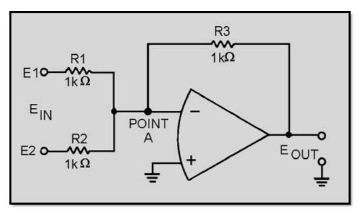
Figure 3-20 Two-input adder
