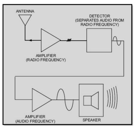
Figure 1-2 Amplifiers as used in radio receiver
