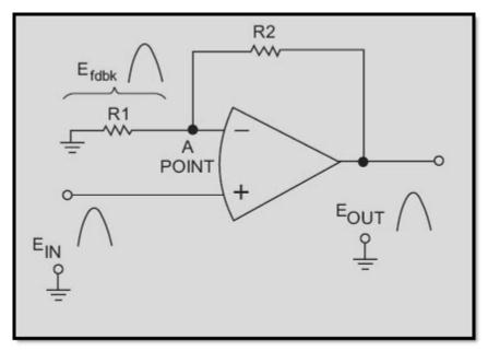
Figure 3-16 Noninverting configuration
