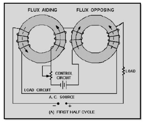
Figure 3-37A Toroidal saturable-core reactor. FIRST HALF CYCLE
