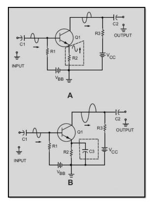
Figure 1-20A-B Decoupling (bypass) capacitor in a transistor amplifier
