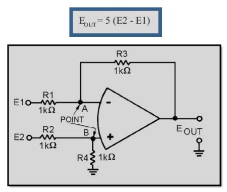
Figure 3-25 Subtractor circuit
