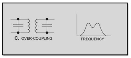
Figure 2-16C.—Effect of coupling on frequency response. OVER-COUPLING
