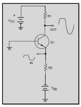
Figure 1-5 A simple class AB transistor amplifier
