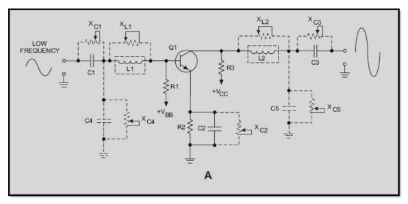
Figure 2-4A Amplifiers showing reactive elements and reactance
