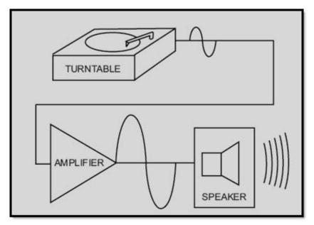
Figure 1-1 Amplifier as used with turntable and speaker
