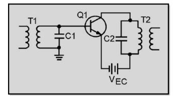
Figure 2-15 Transformer-coupled rf amplifier
