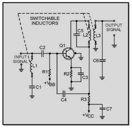
Figure 2-20 Typical vhf television rf amplifier
