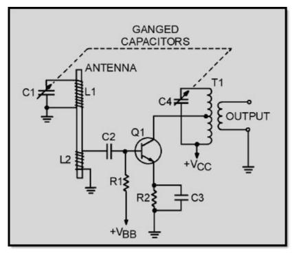
Figure 2-19 Typical AM radio rf amplifier
