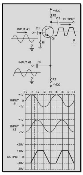
Figure 3-5 Input signals 90° out of phase
