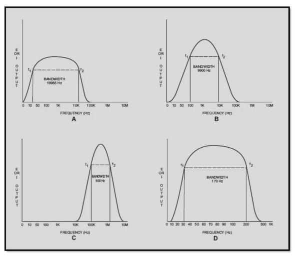
Figure 2-2 Frequency response curves, A THROUGH D
