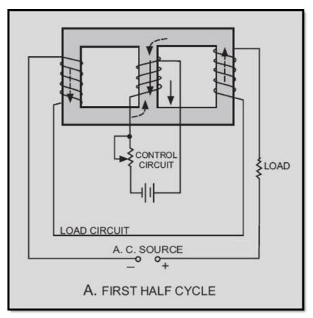
Figure 3-36A Three-legged, saturable-core reactor. FIRST HALF CYCLE
