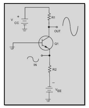
Figure 1-4 A simple class A transistor amplifier
