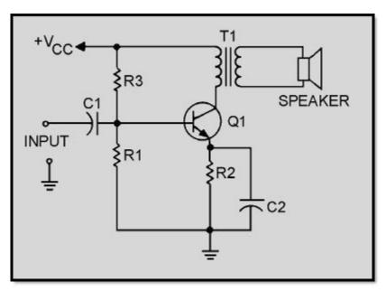
Figure 1-25 Single-stage audio amplifier
