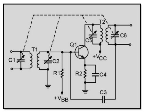
Figure 2-21 Typical rf amplifier
