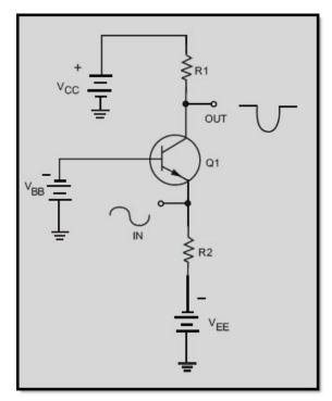
Figure 1-7 A simple class C transistor amplifier
