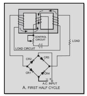
Figure 3-39A Simple full-wave magnetic amplifier. FIRST HALF CYCLE
