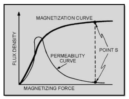
Figure 3-31 Magnetization and permeability curves
