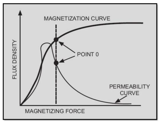
Figure 3-34 Magnetization and permeability curves with operating point
