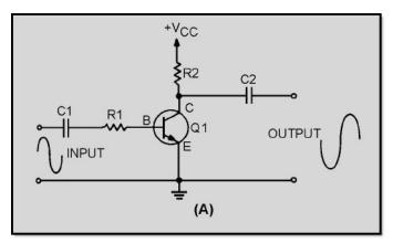
Figure 3-1A Common-emitter and common-base amplifiers
