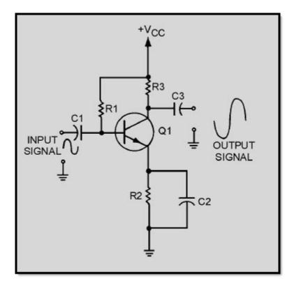
Figure 1-23 Transistor audio amplifier
