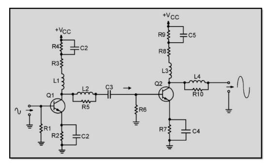
Figure 2-10 Video amplifier circuit
