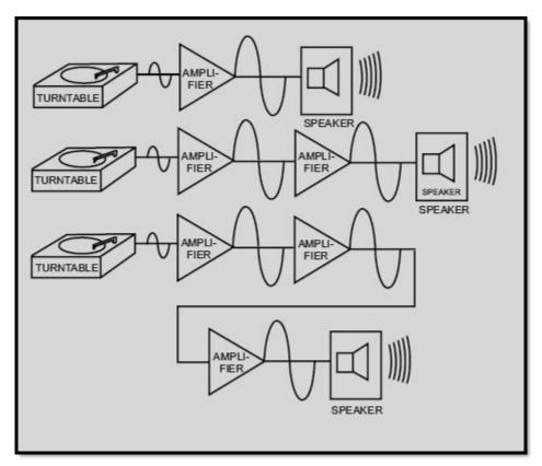
Figure 1-8 Adding stages of amplification
