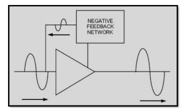
Figure 1-17D.—Feedback uses in amplifiers
