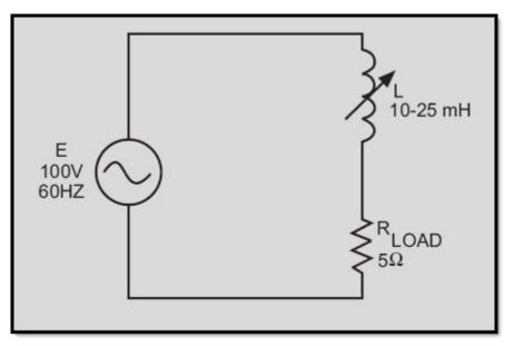
Figure 3-29 Variable inductor in series with a load
