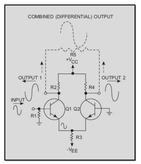
Figure 3-8 Single-input, differential-output differential amplifier
