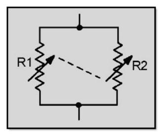
Figure 2-13 Parallel variable resistors (ganged)
