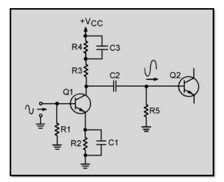
Figure 2-9 Low frequency compensation network
