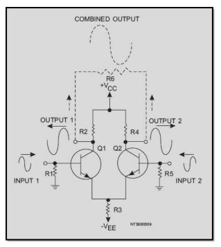
Figure 3-9 Differential-input, differential-output differential amplifier
