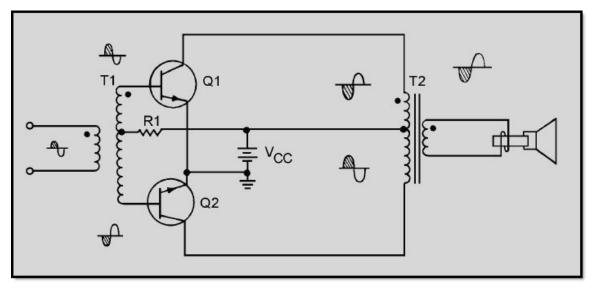
Figure 1-29 Class A transistor push-pull amplifier
