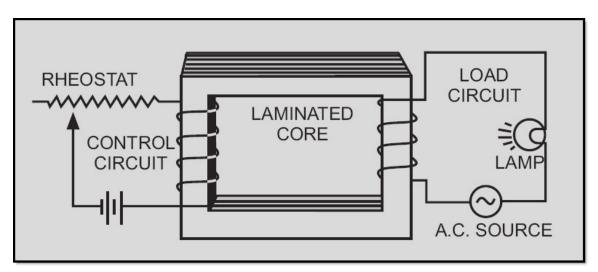
Figure 3-32 A simple saturable-core reactor circuit
