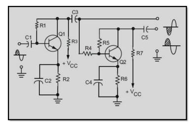
Figure 1-28 Two-stage transistor phase splitter
