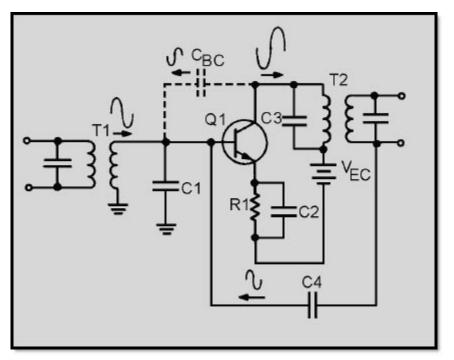
Figure 2-18 Neutralized rf amplifier
