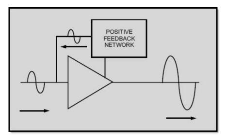
Figure 1-17B.—Feedback uses in amplifiers
