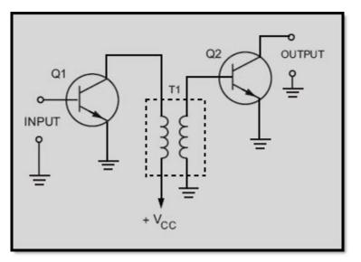
Figure 1-12 Transformer-coupled transistor amplifier
