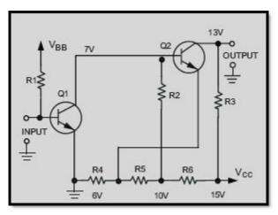
Figure 1-9 Direct-coupled transistor amplifier
