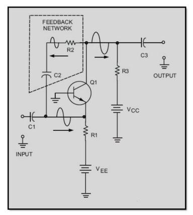
Figure 1-18 Positive feedback in a transistor amplifier
