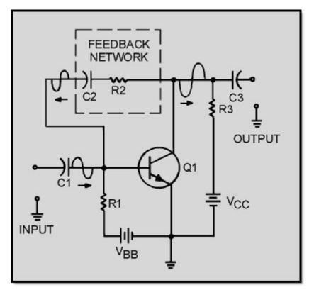
Figure 1-21 Negative feedback in a transistor amplifier
