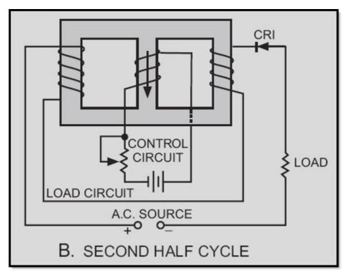
Figure 3-38B.—Simple half-wave magnetic amplifier. SECOND HALF CYCLE
