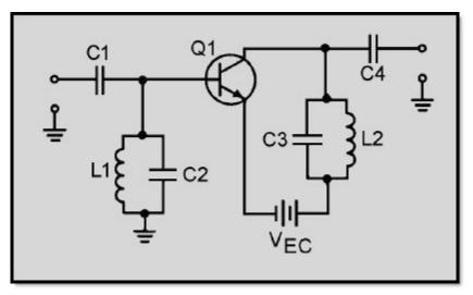
Figure 2-14 Simple rf amplifier
