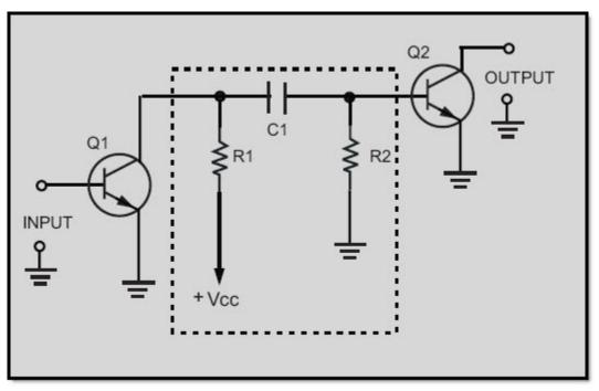
Figure 1-10 RC-coupled transistor amplifier
