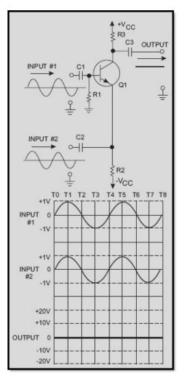
Figure 3-4 Input signals in phase
