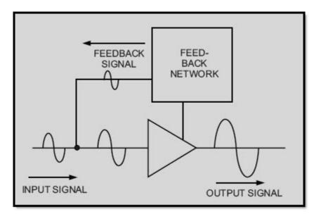
Figure 1-15 Positive feedback in an amplifier
