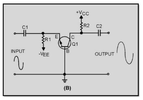
Figure 3-1B.—Common-emitter and common-base amplifiers
