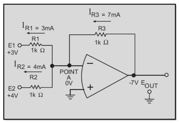
Figure 3-21 Current and voltage in a two-input adder
