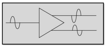
Figure 1-26 Block diagram of a phase splitter
