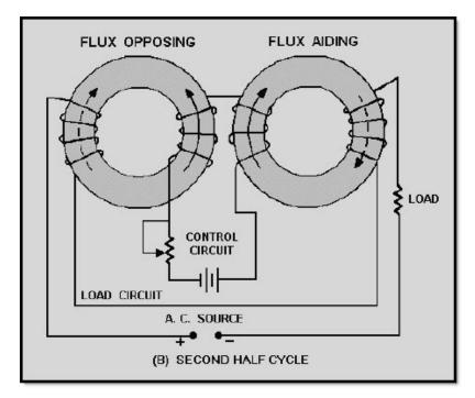
Figure 3-37B.—Toroidal saturable-core reactor. SECOND HALF CYCLE
