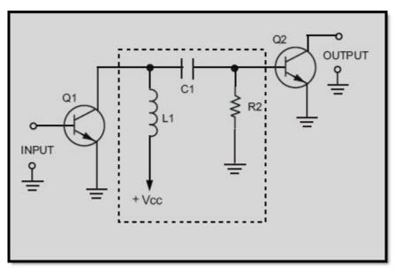
Figure 1-11 Impedance-coupled transistor amplifier
