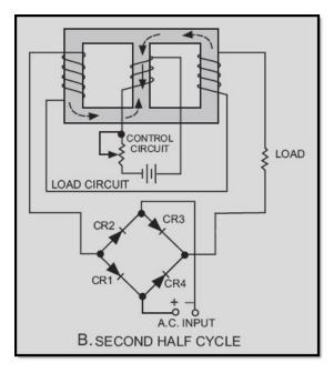
Figure 3-39B.—Simple full-wave magnetic amplifier. SECOND HALF CYCLE
