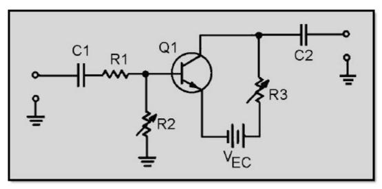
Figure 2-11 Variable input and output impedances
