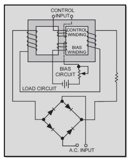
Figure 3-40 Full-wave magnetic amplifier with bias winding
