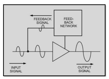
Figure 1-16 Negative feedback in an amplifier
