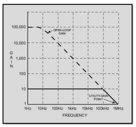
Figure 3-19 Closed-loop frequency-response curve for gain of 10
