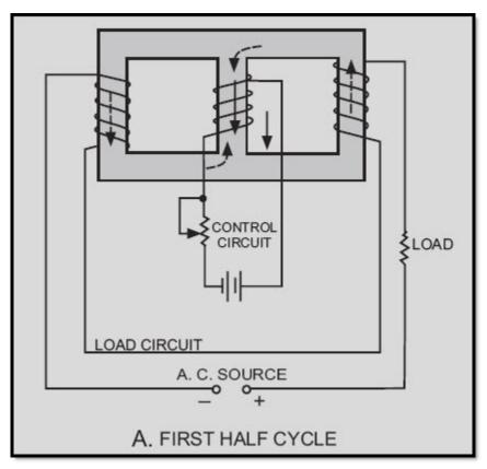
Figure 3-38A Simple half-wave magnetic amplifier. FIRST HALF CYCLE
