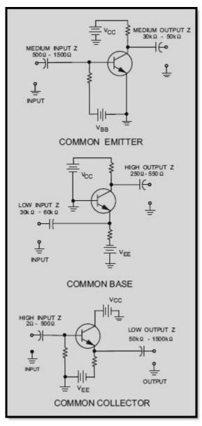
Figure 1-14 Transistor amplifier configurations and their impedance characteristics
