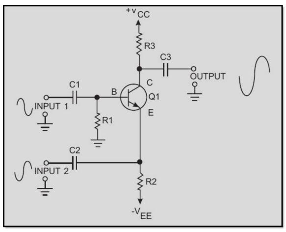
Figure 3-2 Two-input, single-output, difference amplifier
