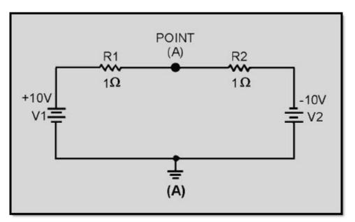
Figure 3-14A Virtual ground circuits
