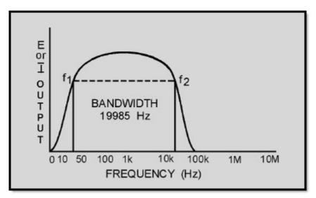
Figure 2-1 Frequency response curve of audio amplifier
