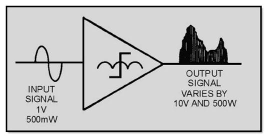
Figure 3-41 Magnetic amplifier input and output signals
