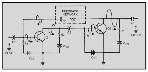
Figure 1-19 Positive feedback in two stages of transistor amplification
