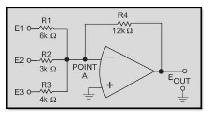
Figure 3-24 Scaling amplifier
