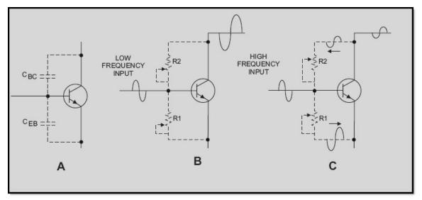
Figure 2-5 Interelectrode capacitance of a transistor
