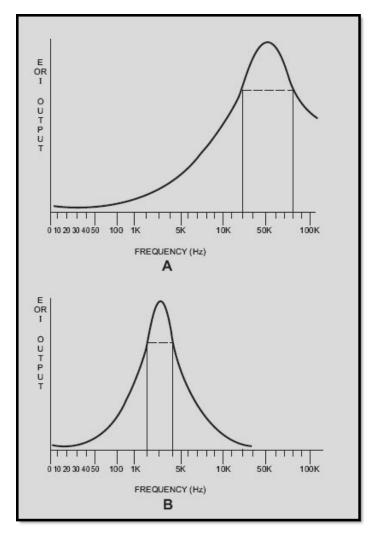
Figure 2-3A-B Frequency-response curves for Q3
