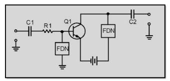
Figure 2-12 Semiblock diagram of rf amplifier
