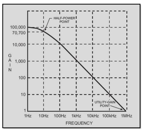
Figure 3-17 Open-loop frequency-response curve
