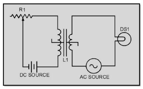
Figure 3-33 Schematic diagram of a simple saturable-core reactor
