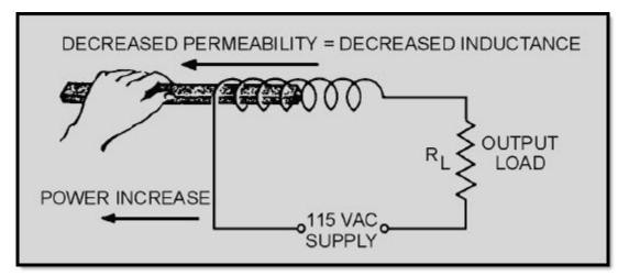
Figure 3-30 Varying coil inductance with a movable coil
