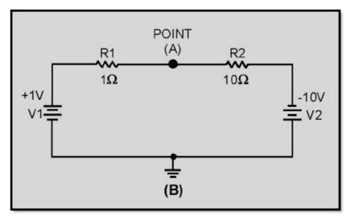
Figure 3-14B.—Virtual ground circuits
