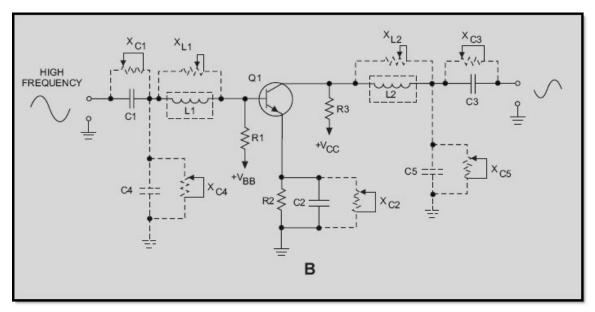
Figure 2-4B.—Amplifiers showing reactive elements and reactance
