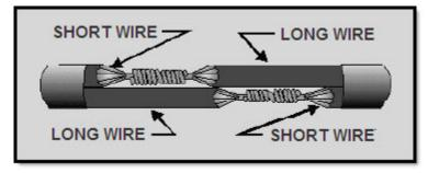
Figure 2-6 Staggering splices
