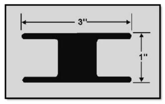
Figure 2-40 Lacing shuttle
