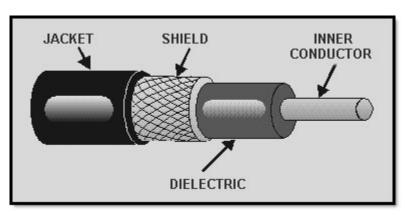
Figure 1-18 Coaxial cable
