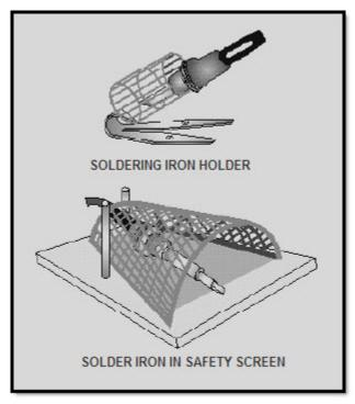
Figure 2-38 Soldering iron safety devices
