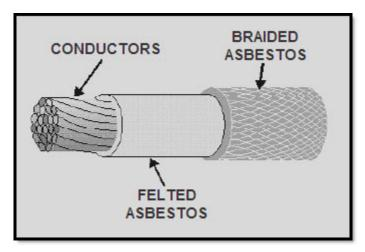
Figure 1-9 Asbestos Insulation
