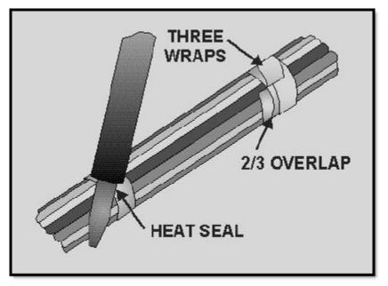
Figure 2-52 Securing wire bundles in high-temperature areas
