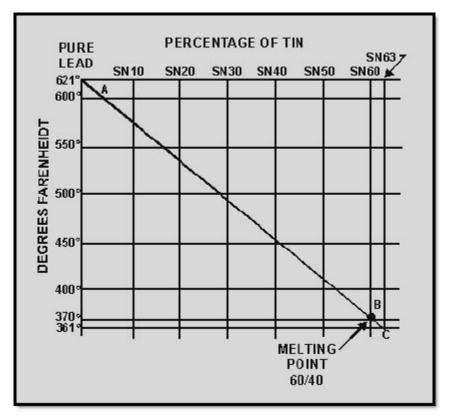
Figure 2-35 Tin-lead fusion diagram
