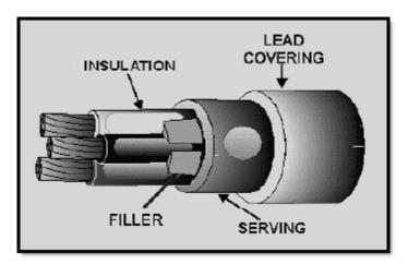
Figure 1-16 Lead-sheathed cable
