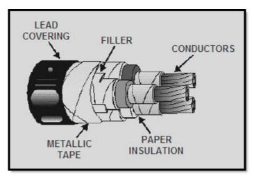
Figure 1-11 Paper-insulated power cables
