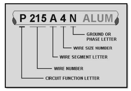
Figure 3-3 Aircraft wire marking
