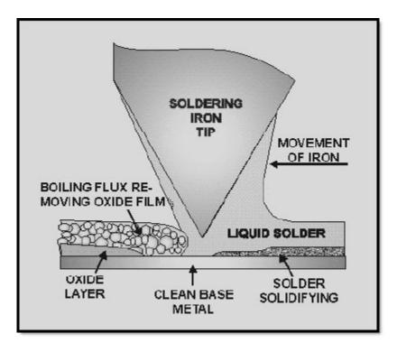
Figure 2-36 Action of flux
