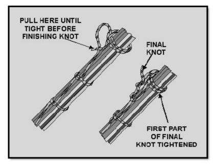
Figure 2-45 Alternate method of terminating the lace
