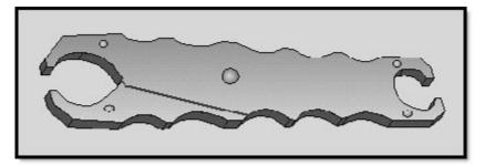
Figure 3-13 Fuse puller
