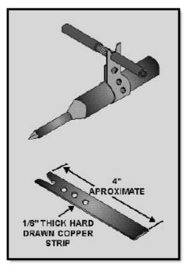
Figure 2-4 Locally made hot-blade stripper
