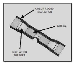
Figure 2-23 Preinsulated copper splice
