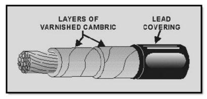
Figure 1-8 Varnished cambric insulation
