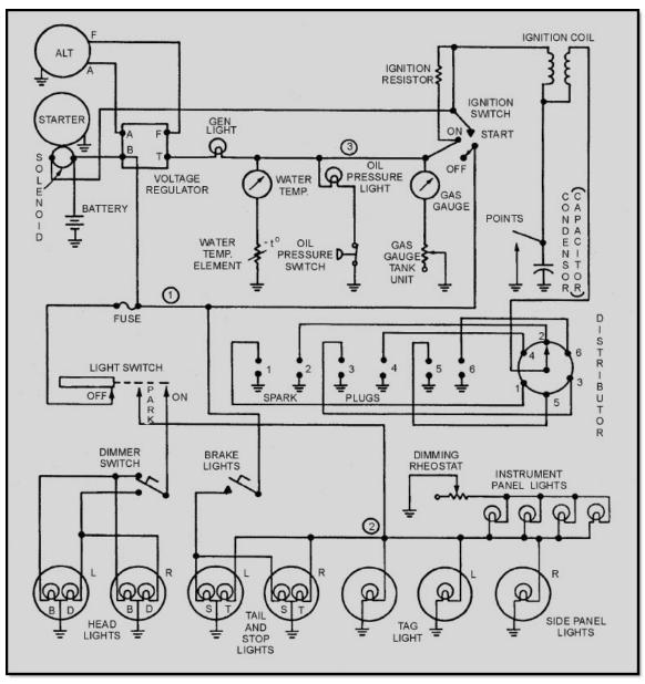
Figure 3-10 Schematic diagram
