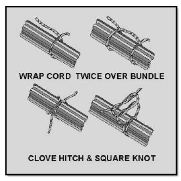
Figure 2-49 Making spot ties
