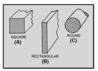
Figure 1-1 Cross-sectional areas of conductors
