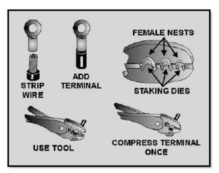
Figure 2-12 Crimping small copper uninsulated terminals
