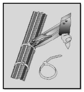
Figure 2-50 Installing self-clinching cable straps
