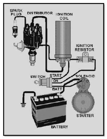
Figure 3-6 Pictorial diagram of automotive starter and ignition systems
