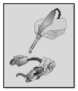
Figure 2-32 Resistance soldering set
