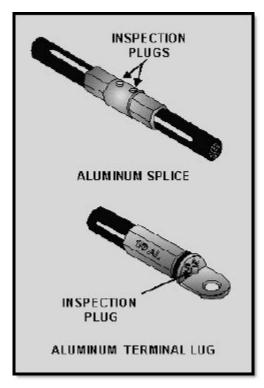
Figure 2-17 Aluminum terminal lug and splice
