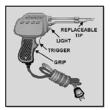
Figure 2-31 Soldering gun
