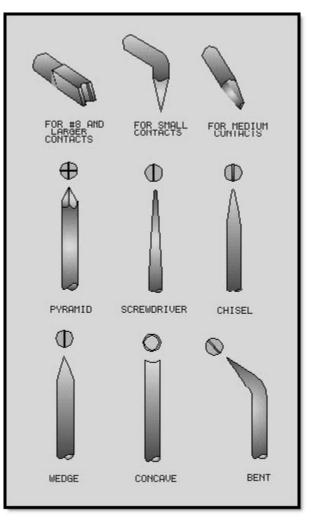
Figure 2-29 Soldering iron tip shapes
