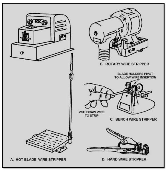
Figure 2-1 Typical wire-stripping tools
