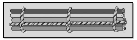
Figure 2-39 Conductor lacing
