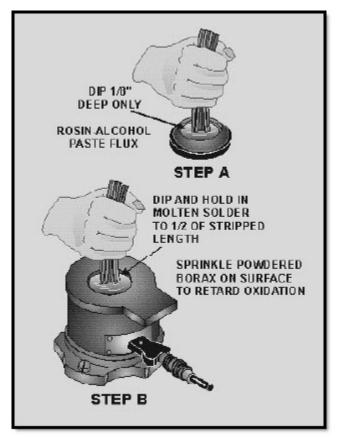
Figure 2-25 Dip-tinning In a solder pot
