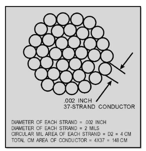
Figure 1-6 Stranded conductor
