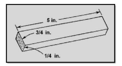
Figure 1A Rectangular Bar Conductor
