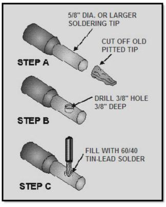
Figure 2-26 Alternate dip-tinning method
