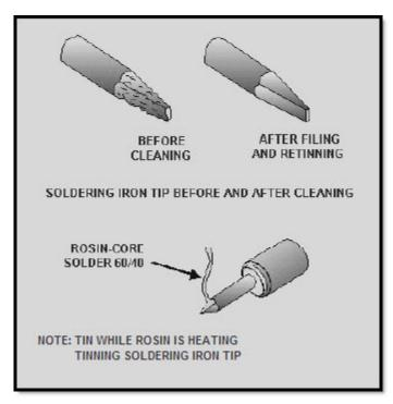
Figure 2-30 Reconditioning pitted soldering iron tip
