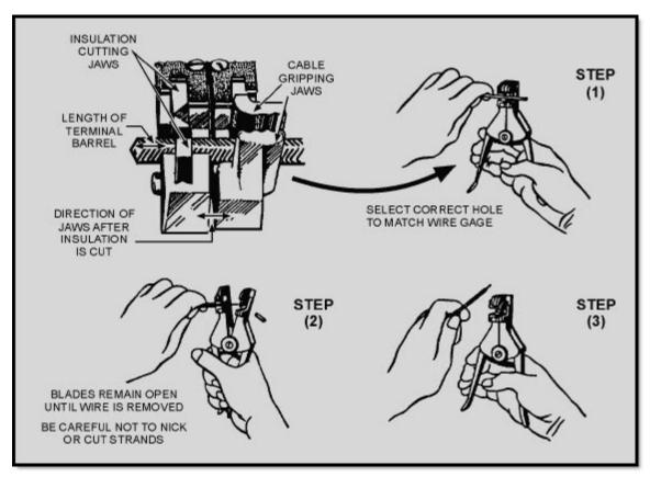
Figure 2-2 Stripping wire with a hand stripper
