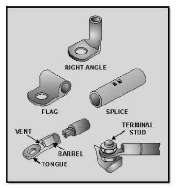
Figure 2-11 Noninsulated terminal lugs and splices
