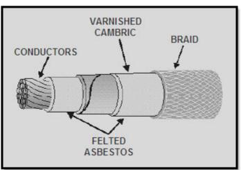
Figure 1-10 Asbestos and varnished cambric insulation
