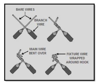
Figure 2-8 Fixture joint
