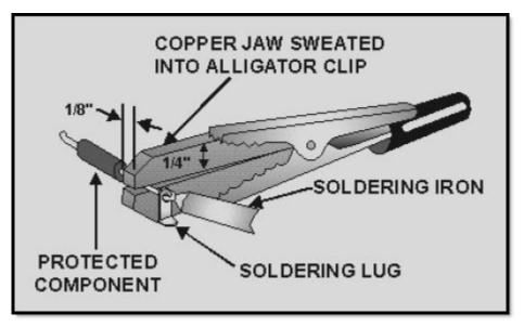
Figure 2-37 Heat shunt
