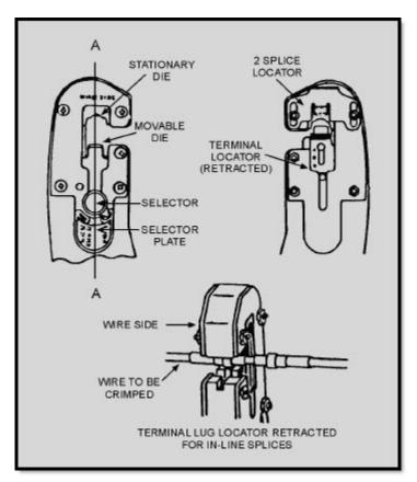
Figure 2-24 Locating splice in crimping tool
