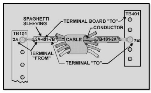
Figure 3-4 Designating conductor marking between unlike terminals
