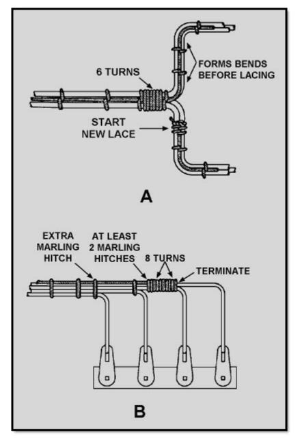
Figure 2-42 Lacing branches and breakouts
