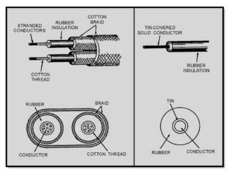
Figure 1-7 Rubber insulation
