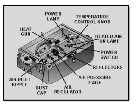
Figure 2-16 Compressed air/nitrogen heating tool
