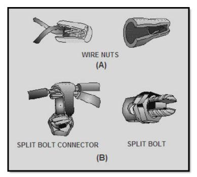
Figure 2-10 Wire nut and split bolt splices
