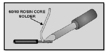
Figure 2-27 Tinning wire with a soldering iron
