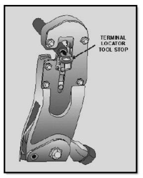
Figure 2-21 Crimping tool with terminal lug inserted
