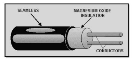
Figure 1-14 Two-conductor mineral-insulated (MI) cable
