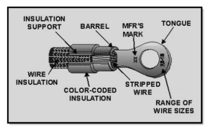
Figure 2-19 Preinsulated straight copper terminal lug
