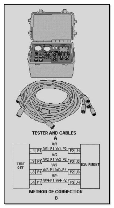
Figure 3-2 Test equipment cable marking
