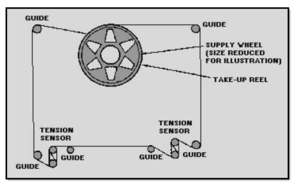
Figure 4-8 Co-axial tape reeling configuration
