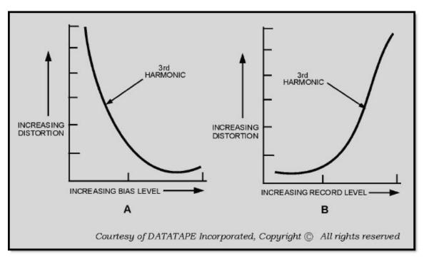
Figure 6-4 A & B Effect of signal bias level and record level on harmonic-distortion level
