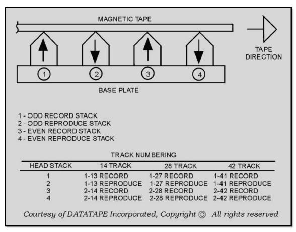
Figure 3-4 Magnetic head track placement
