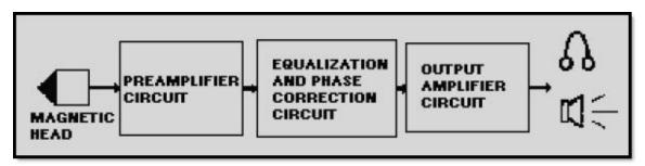
**Figure 5-2 Direct reproduce electronics**
