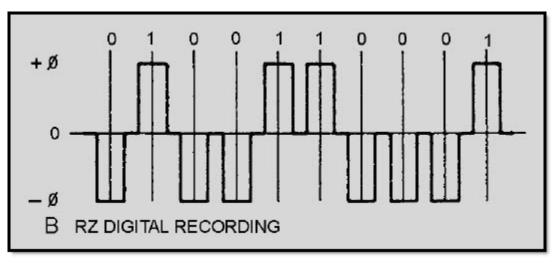
Figure 7-3 Return-to-zero (RZ) digital encoding method
