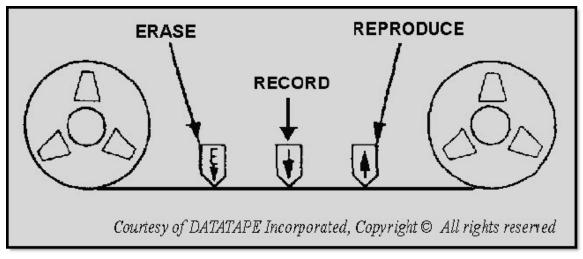
Figure 3-3 Placement of magnetic tape recorder heads
