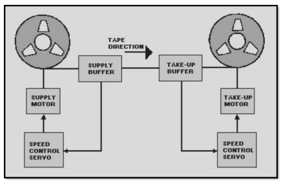
Figure 4-2 Tape buffering arrangement
