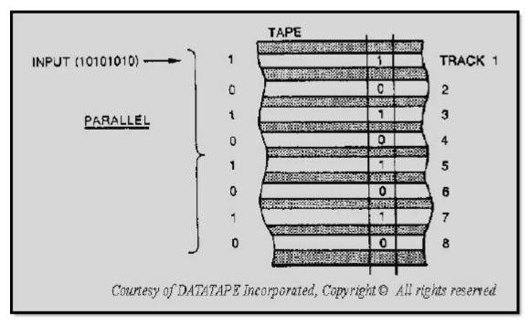
Figure 7-1B Digital magnetic tape recording formats
