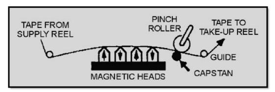
Figure 4-9 Open-loop capstan drive tape transport
