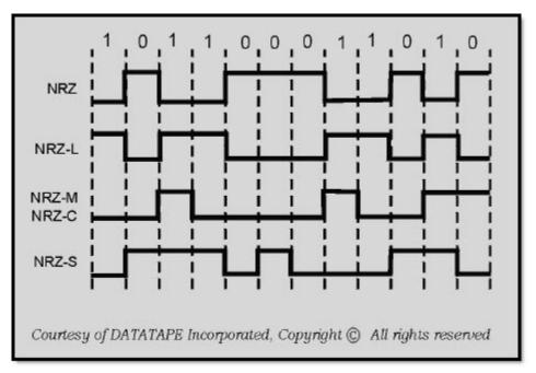
Figure 7-4 Non-return-to-zero (NRZ) digital encoding method
