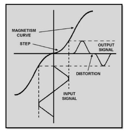
Figure 1-1 Magnetic recording without bias voltage
