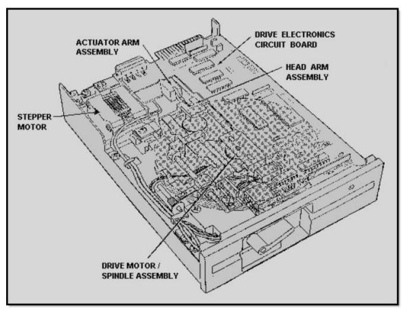
Figure 8-9 Typical floppy disk drive transport
