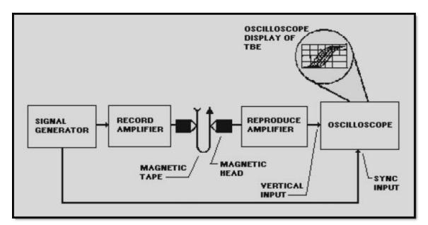
Figure 6-9 Test equipment setup for measuring time-base error
