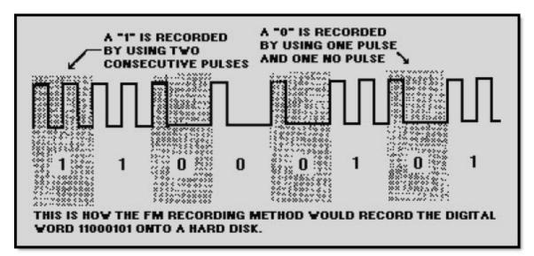
Figure 8-7 Frequency-modulation (FM) encoding
