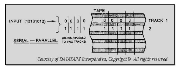
Figure 7-1C Digital magnetic tape recording formats
