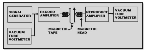
Figure 6-1 Test equipment setup for measuring signal-to-noise ratio
