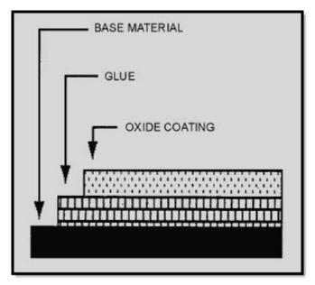
Figure 2-1 Magnetic tape construction
