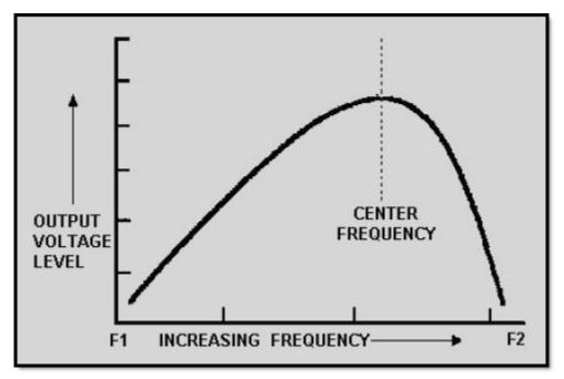
Figure 6-2 Frequency response of a reproduce head
