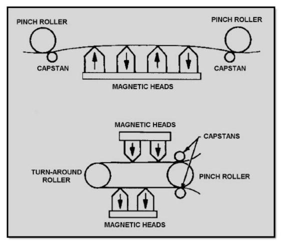
Figure 4-10 Closed loop capstan drive tape transport
