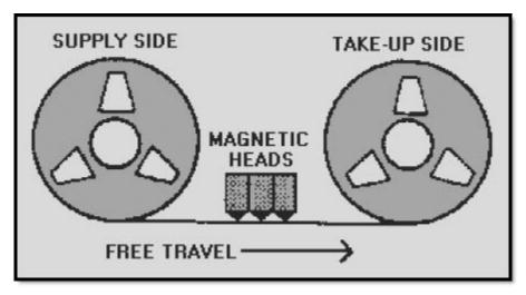
Figure 4-1 Basic tape transport assembly
