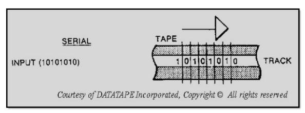
Figure 7-1A Digital magnetic tape recording formats
