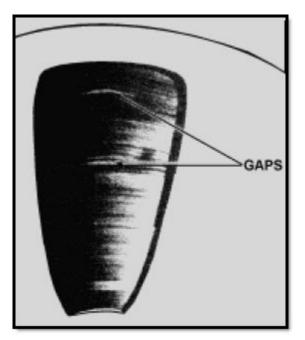
Figure 2-5 Example of windowed tape pack
