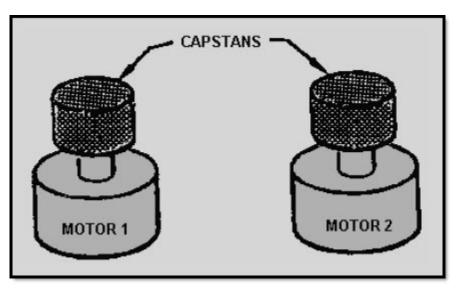
Figure 4-12 Dual-motors dual capstans drive system
