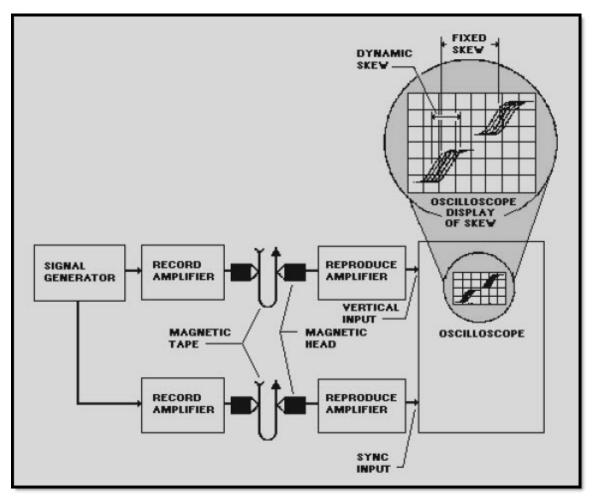
Figure 6-10 Test equipment setup for measuring skew
