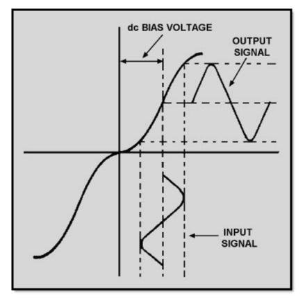
Figure 1-2 Magnetic recording with dc bias voltage
