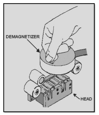
Figure 3-6 Demagnetizing magnetic heads with a degausser
