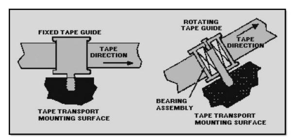
Figure 4-6 Typical fixed and rotary tape guides
