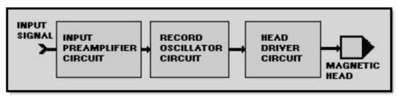
Figure 5-4 FM record electronics
