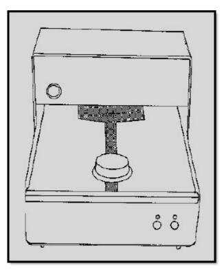
Figure 2-7 Automatic tape degausser
