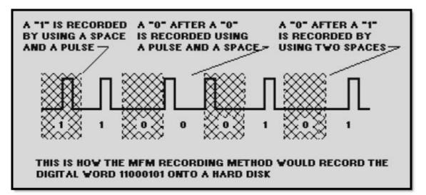
Figure 8-8 Modified frequency-modulation (MFM) encoding
