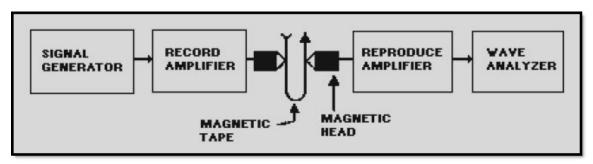
Figure 6-5 Test equipment setup for measuring harmonic distortion
