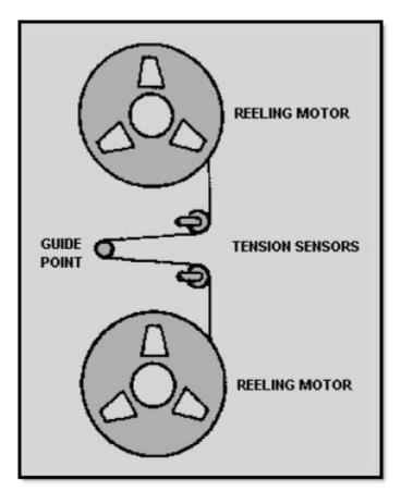
Figure 4-7 Co-planar tape reeling configuration
