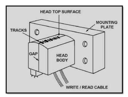
Figure 3-1 Typical multitrack magnetic tape recorder head
