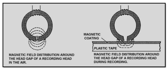
Figure 1-4 Magnetic field distribution around the head gap
