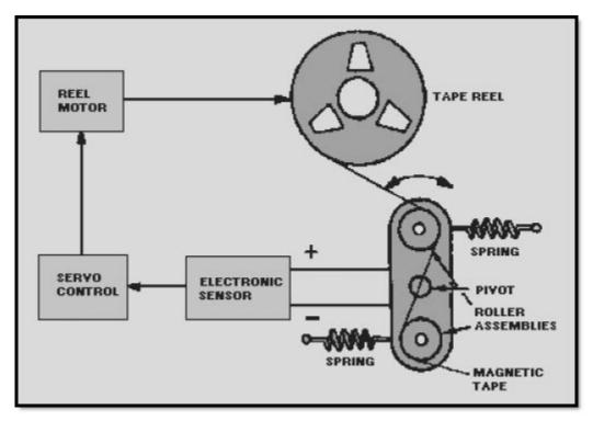
Figure 4-4 Mechanical arm spring-tension tape buffering
