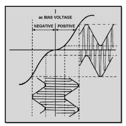
Figure 1-3 Magnetic recording with ac bias voltage
