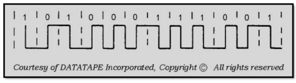
Figure 7-6 Bi-phase level digital encoding method
