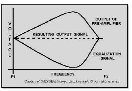
**Figure 5-3 Equalization process**
