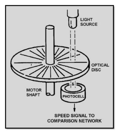
Figure 4-15 Capstan speed monitor using a photo-optical tachometer
