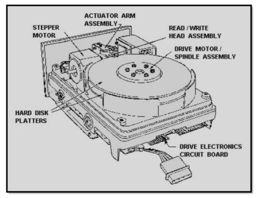
Figure 8-10 Typical hard disk drive transport
