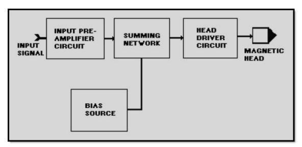
Figure 5-1 Direct record electronics
