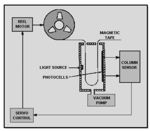
Figure 4-5 Vacuum-column tape buffering system
