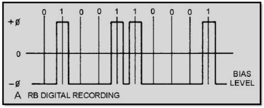
Figure 7-2 Return-to-bias (RB) digital encoding method
