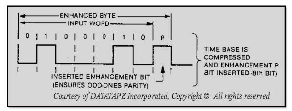
Figure 7-5 Enhanced non-return-to-zero-level (E-NRZ-L) digital encoding method
