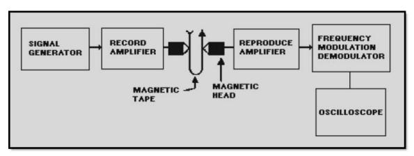
Figure 6-8 Test equipment setup for measuring flutter
