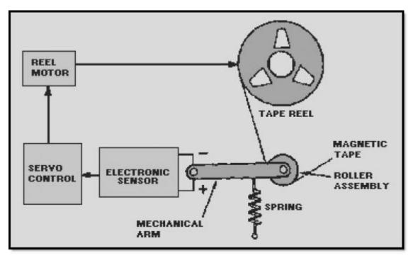
Figure 4-3 Mechanical arm spring-tension tape buffering
