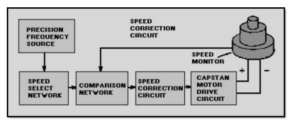
Figure 4-14 Six parts of the capstan speed control function
