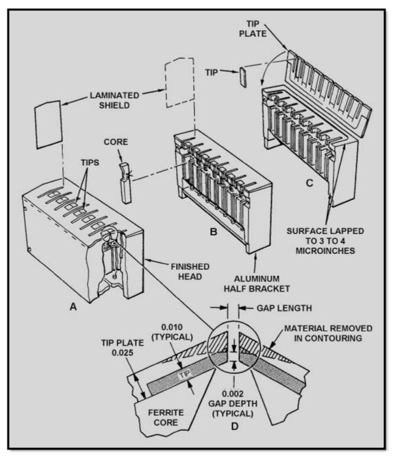
Figure 3-2 Multitrack tape recorder head construction
