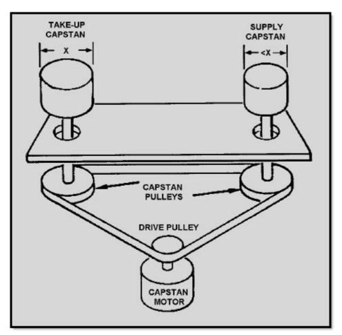
Figure 4-11 Differential velocity capstan drive
