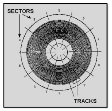
Figure 8-2 Tracks and sectors of a magnetic disk
