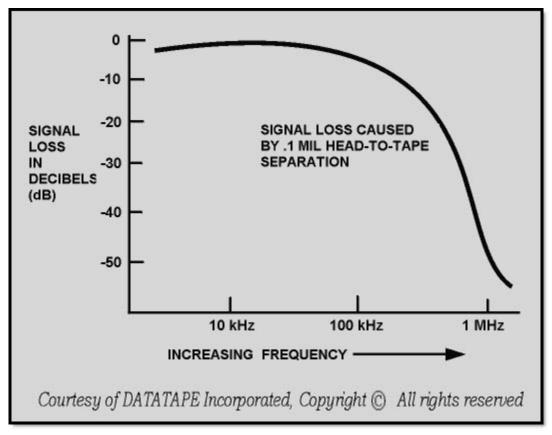
Figure 6-3 Effects of poor tape-to-head contact
