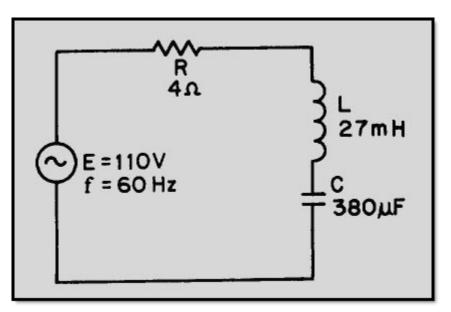
Figure 4-11 Example series RLC circuit
