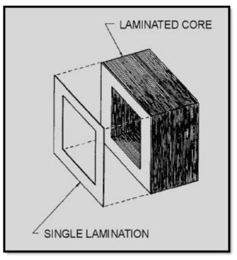
Figure 5-2 Hollow-core construction
