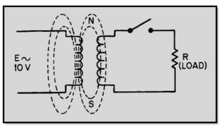
Figure 5-8 Transformer under no-load conditions
