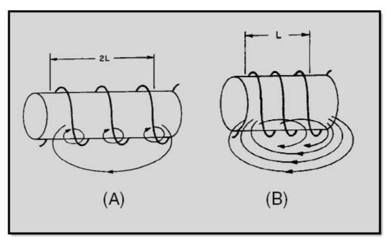
Figure 2-7 Inductance factor (coil length). CLOSELY WOUND
