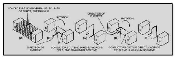
Figure 1-7 Simple alternating-current generator
