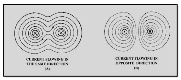
Figure 1-4 Magnetic field around two parallel conductors
