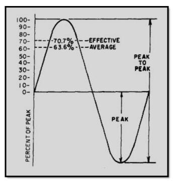
Figure 1-16 Various values used to indicate sine-wave amplitude
