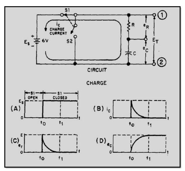
Figure 3-9 Charge of an RC series circuit
