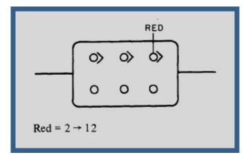
5. Read the multiplier dot and multiply the first two digits by multiplier. (Remember that the multiplier is in picofarads).
