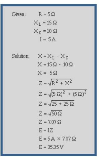
*Q18.* What are the Ohm's law formulas used in an ac circuit to determine voltage and current?
