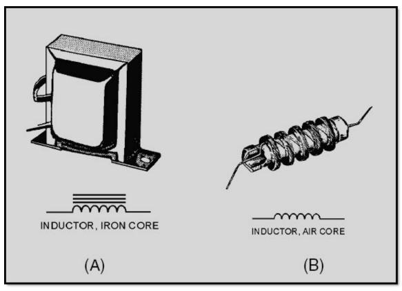
Figure 2-4 Inductor types and schematic symbols
