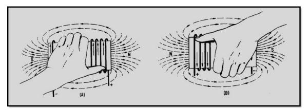
Figure 1-6 Left-hand rule for coils
