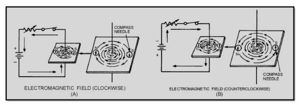
Figure 1-2 Magnetic field around a current-carrying conductor
