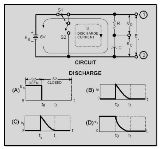
Figure 3-10 Discharge of an RC Series circuit
