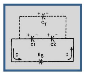
Figure 3-13 Capacitors in series
