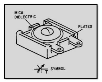
Figure 3-20 Trimmer capacitor
