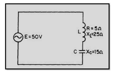
Figure 4-8 Series LC circuit
