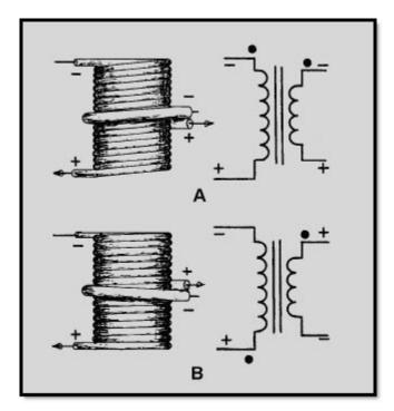
Figure 5-9 Instantaneous polarity depends on direction of winding
