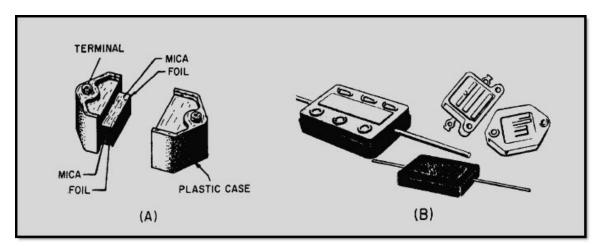
Figure 3-16 Typical mica capacitors
