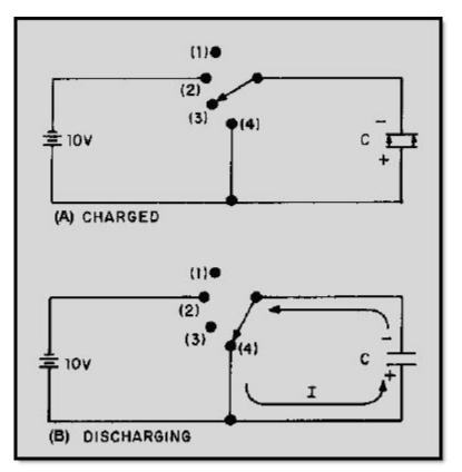
Figure 3-8 Discharging a capacitor
