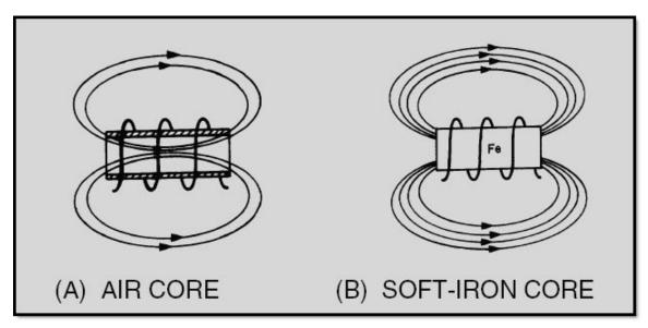
Figure 2-8 Inductance factor (core material)
