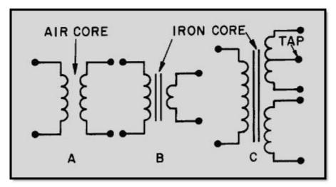
Figure 5-7 Schematic symbols for various types of transformers
