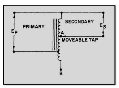
Figure 5-13 Schematic diagram of an autotransformer
