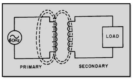
Figure 5-1 Basic transformer action
