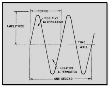
Figure 1-10 Period of a sine wave
