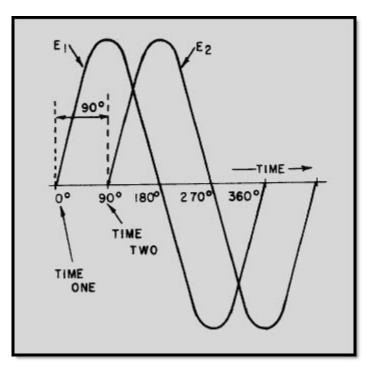
Figure 1-18 Voltage waves 90° out of phase
