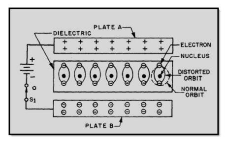
Figure 3-4 Distortion of electron orbits in a dielectric
