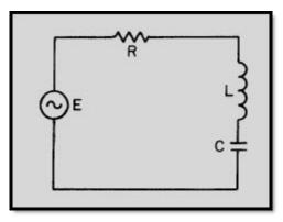
Figure 4-4 Series RLC circuit
