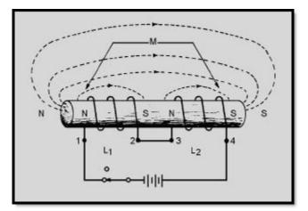
Figure 2-14 Series inductors with aiding fields
