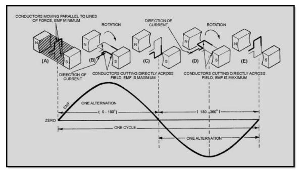
Figure 1-8 Basic alternating-current generator
