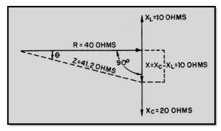
Figure 4-7 Vector diagram showing relationship of resistance, reactance (capacitive and inductive), and
