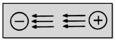
Figure 3-1 Electrostatic field attracts two unlike charged particles
