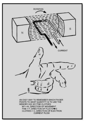
Figure 1-9 Left-hand rule for generators
