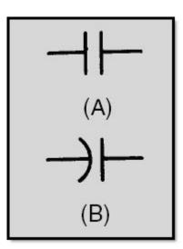
Figure 3-5 Circuit symbols for capacitors
