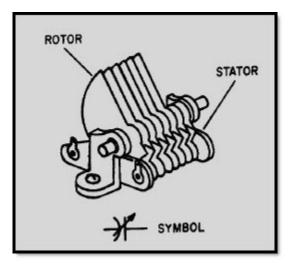
Figure 3-19 Rotor-stator type variable capacitor
