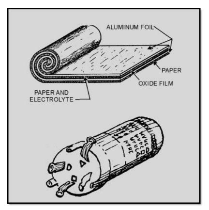
Figure 3-18 Construction of an electrolytic capacitor
