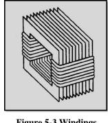
Figure 5-3 Windings wrapped around laminations 5-5
