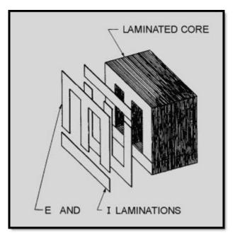
Figure 5-4 Shell-type core construction
