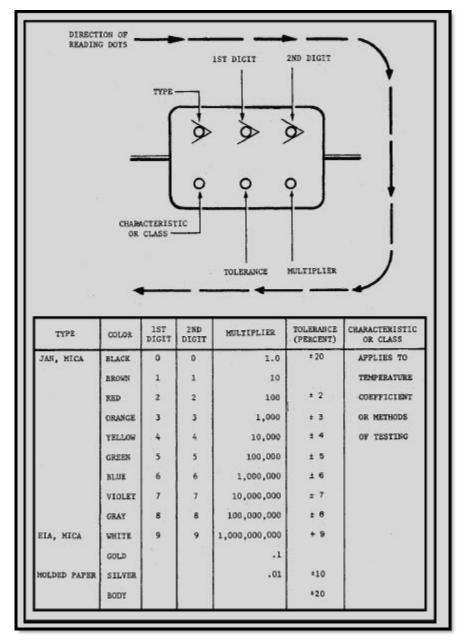
Figure 3-21 6-dot color code for mica and molded paper capacitors
