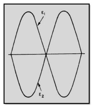
Figure 1-19 Voltage waves 180° out of phase
