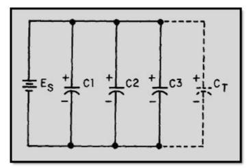
Figure 3-14 Parallel capacitive circuit
