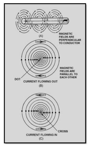
Figure 1-3 Magnetic field around a currentcarrying conductor, detailed view
