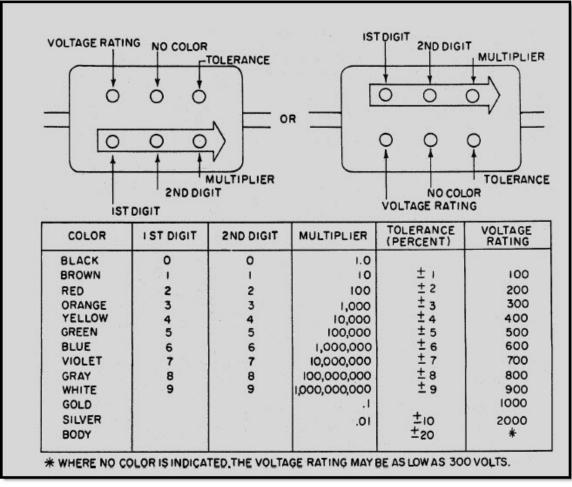
Figure 3-24 Mica capacitor color code
