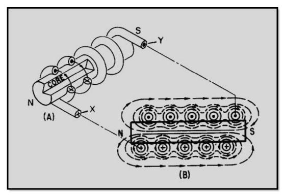
Figure 1-5 Magnetic field produced by a current-carrying coil
