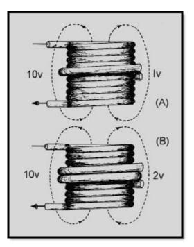
Figure 5-10 Transformer turns and voltage ratios
