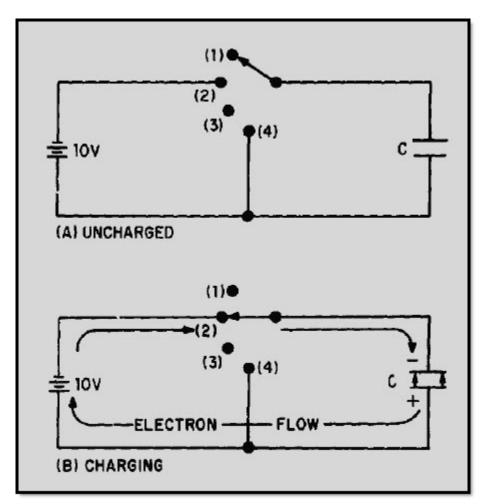
Figure 3-6 Charging a capacitor
