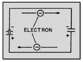
Figure 3-7 Electron motion during charge
