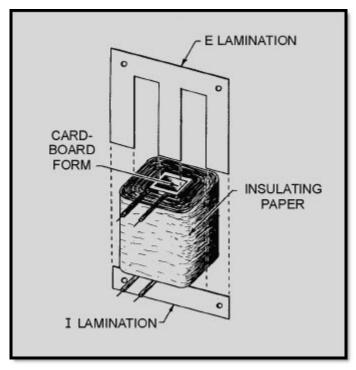
Figure 5-5 Exploded view of shell-type transformer construction
