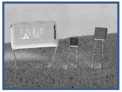
Figure 3-17 Ceramic capacitors
