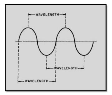
Figure 1-12 Wavelength measurement
