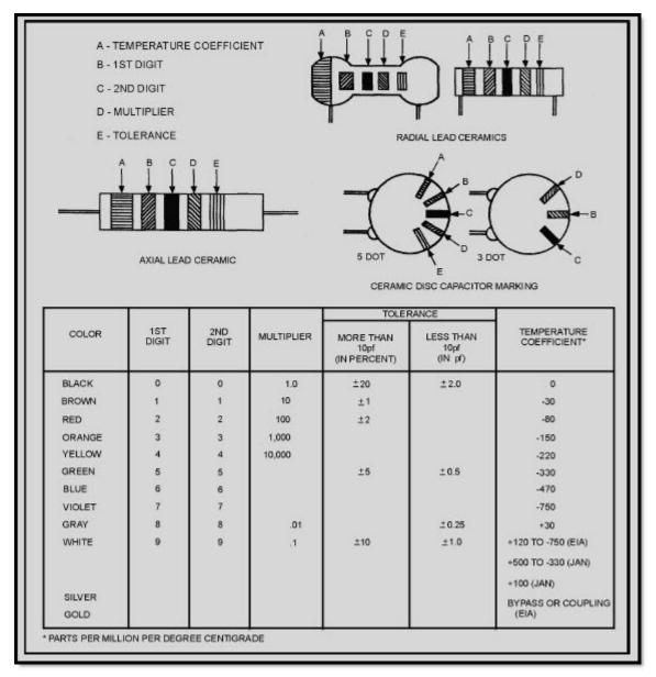
Figure 3-23 Ceramic capacitor color code
