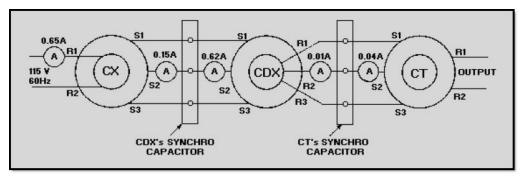
Figure 1-33 The effects of synchro capacitors in a control synchro system using a CDX and a CT
