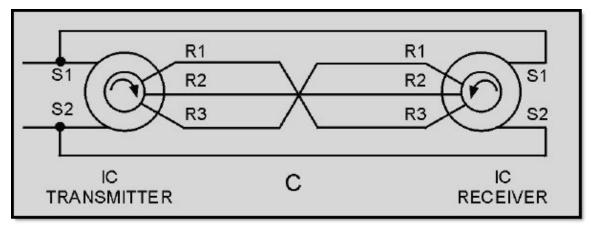
Figure 4-2C.—IC versus standard synchro connections
