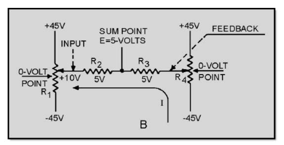
Figure 2-4B.—Development of the error signal
