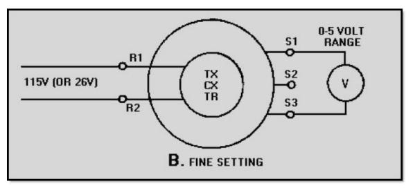
Figure 1-39B.—Zeroing differential synchros by the voltmeter method.
