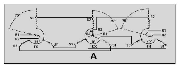
Figure 1-21A TX-TR system operation (addition)
