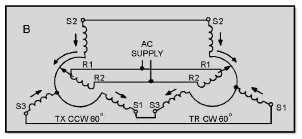
Figure 1-17B.—Effect of reversing the S1 and S3 connections between the transmitter and the receiver
