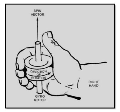
Figure 3-9 Determining spin vector direction
