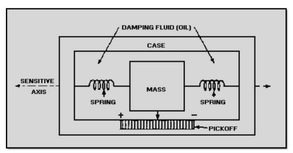
Figure 3-20 The basic accelerometer
