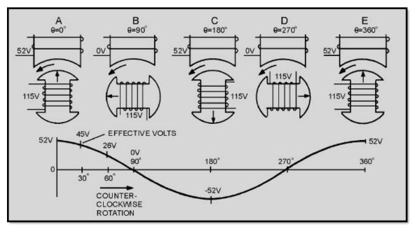
Figure 1-14 Stator voltage vs rotor position
