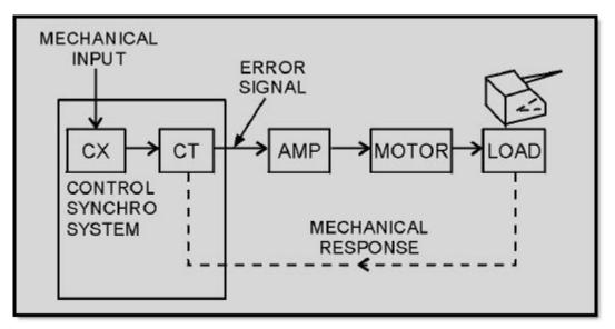
Figure 1-28 A positioning servo system using a control synchro system
