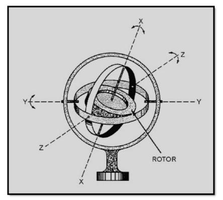
Figure 3-1 Gyro model, universally mounted
