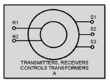
Figure 1-3A Schematic symbols for synchros
