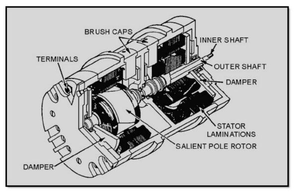
Figure 1-35 Cutaway view of a double receiver
