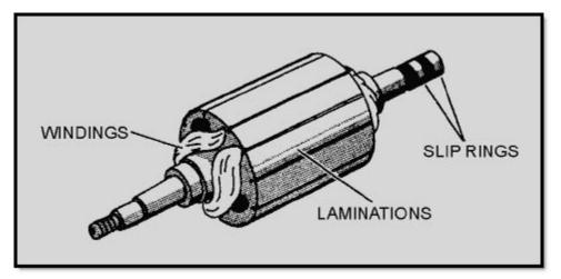
Figure 1-6 Drum or wound rotor
