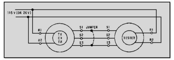
Figure 1-43 Zeroing a synchro using a synchro tester
