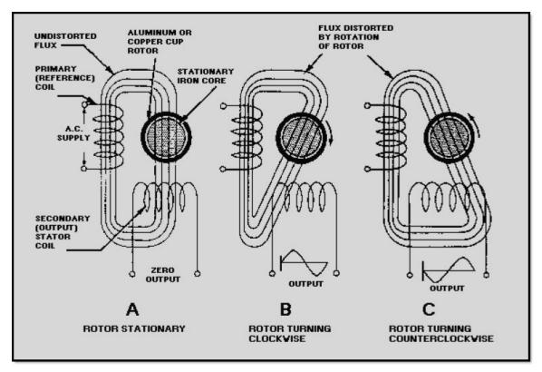
Figure 2-16 Ac drag-cup rate generator
