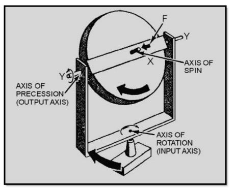
Figure 3-14 Rate gyro precession
