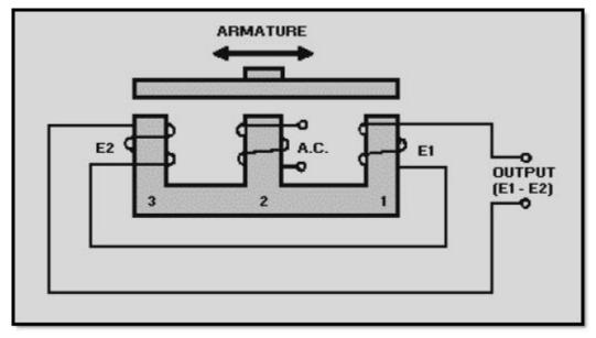
Figure 2-14 Basic-E transformer
