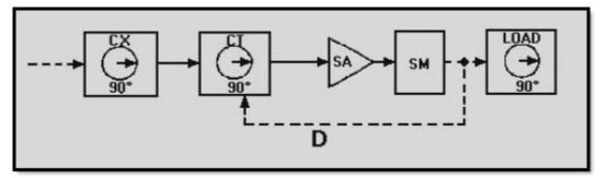
Figure 2-2D.—A basic servo system (closed-loop)
