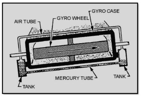
Figure 3-12 Mercury erecting system
