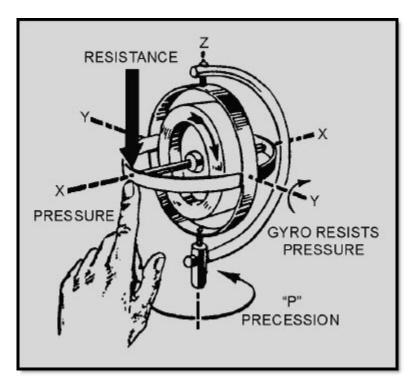
Figure 3-8 Force applied to a gyro
