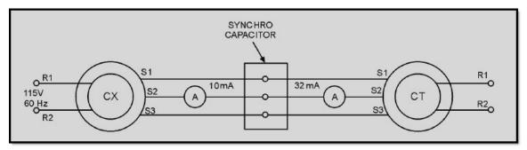
Figure 1-30 The use of a synchro capacitor with a CT
