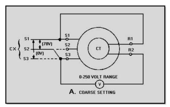
Figure 1-40A Zeroing a control transformer by the voltmeter method
