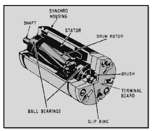
Figure 1-4 Typical synchro assembly
