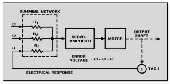
Figure 2-13 Summing network as an error detector
