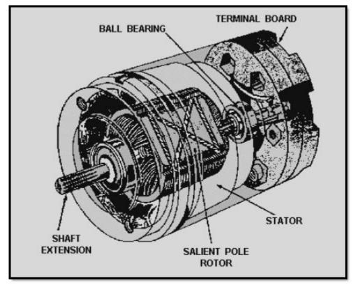
Figure 1-1 Phantom view of a synchro
