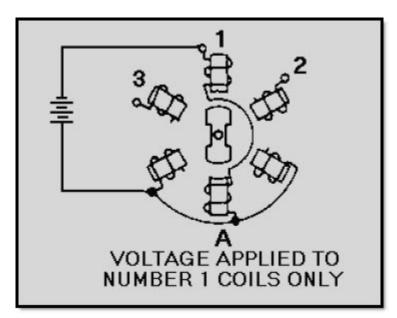
Figure 4-4A Step-by-step motor in various positions. VOLTAGE APPLIED TO NUMBER 1 COILS ONLY
