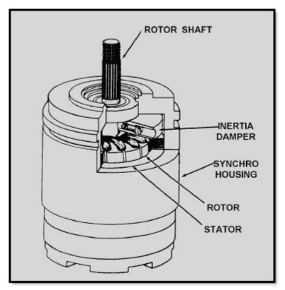
Figure 1-15 Cutaway view of torque receiver with inertia damper
