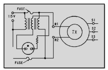
Figure 1-46 Blown fuse indicator requiring only one lamp
