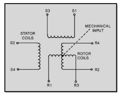
Figure 4-6 Resolver schematic
