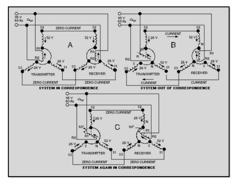
Figure 1-16 A simple synchro transmission system
