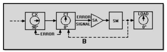
Figure 2-2B.—A basic servo system (closed-loop)
