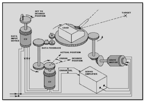
Figure 2-5 Typical position servo
