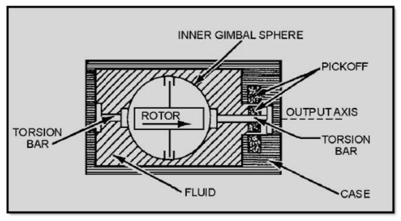
Figure 3-17 Torsion bar-restrained floated rate gyro
