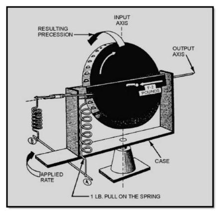
Figure 3-15 Precession of a spring restrained rate gyro
