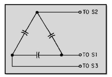
Figure 1-29 The synchro capacitor
