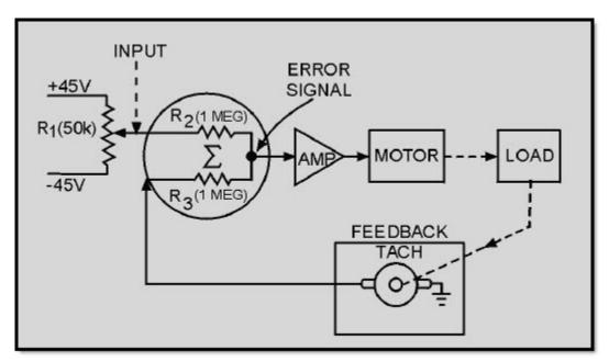
Figure 2-7 Block diagram of a velocity servo
