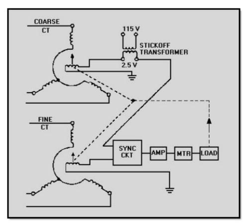
Figure 1-36 Dual-speed synchro system using a stickoff transformer
