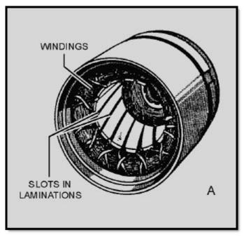
Figure 1-7A Typical stator
