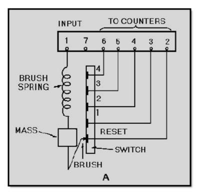
Figure 3-22A Pulse counting accelerometer
