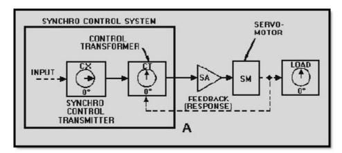
Figure 2-2A A basic servo system (closed-loop)
