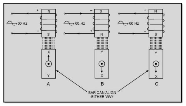
Figure 1-11 Operation of an electromagnet with ac voltage
