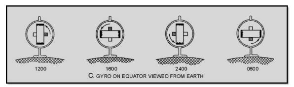
Figure 3-11C.—Fixed direction in space. Gyro on equator viewed from earth
