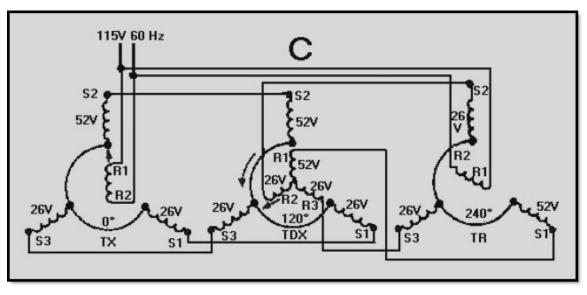
Figure 1-20C.—TX-TDX-TR system operation (subtraction)
