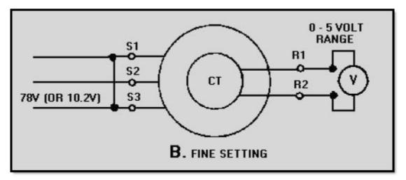
Figure 1-40B.—Zeroing a control transformer by the voltmeter method
