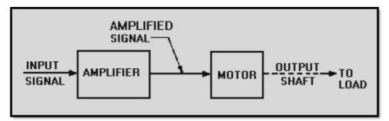
Figure 2-1 Open-loop control system basic block diagram
