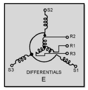
Figure 1-3E.—Schematic symbols for synchros
