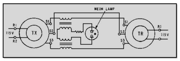
Figure 1-44 Overload stator current indicator
