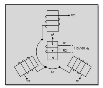
Figure 1-13 Synchro transmitter
