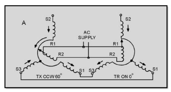
Figure 1-17A Effect of reversing the S1 and S3 connections between the transmitter and the receiver
