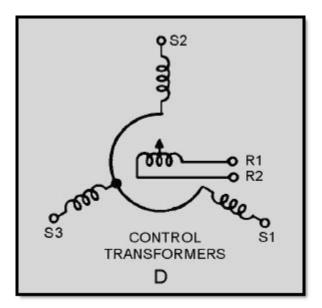
Figure 1-3D.—Schematic symbols for synchros
