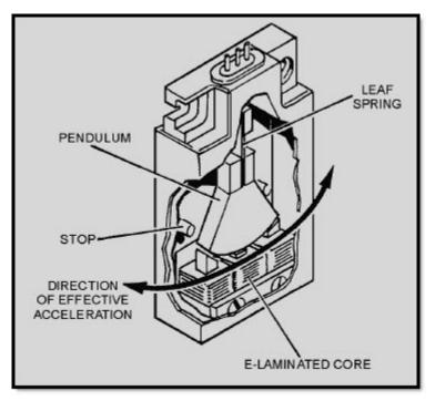
Figure 3-21 E-transformer accelerometer
