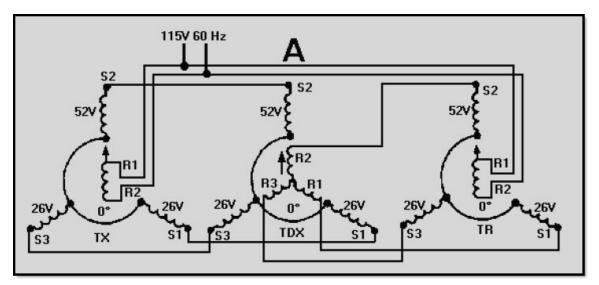
Figure 1-20A TX-TDX-TR system operation (subtraction)
