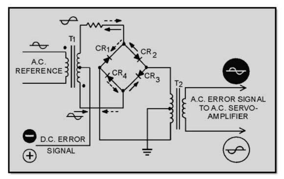
Figure 2-17 Crystal diode modulator
