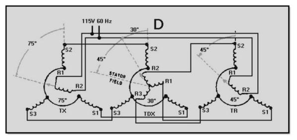
Figure 1-20D.—TX-TDX-TR system operation (subtraction)
