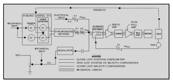
Figure 2-21 Multi-loop servo system
