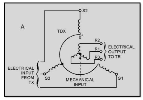
Figure 1-19A Torque differential transmitter
