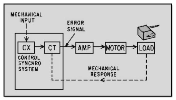
Figure 1-27A Control synchro system operation
