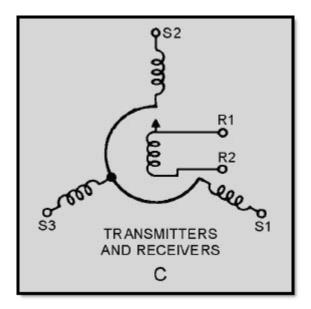
Figure 1-3C.—Schematic symbols for synchros
