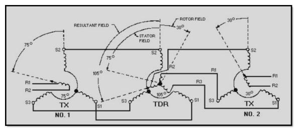
Figure 1-23 TX-TDR-TX system operation (addition)
