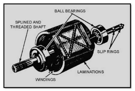
Figure 1-5 Salient-pole rotor
