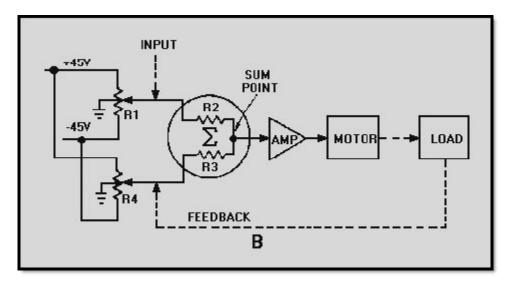
Figure 2-3B.—Block diagram of a position servo
