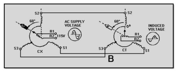
Figure 1-27B.—Control synchro system operation
