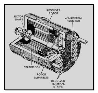
Figure 4-5 Cutaway view of a resolver
