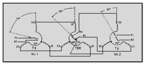
Figure 1-22 TX-TDR-TX system operation (subtraction)
