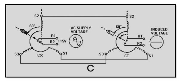
Figure 1-27C.—Control synchro system operation
