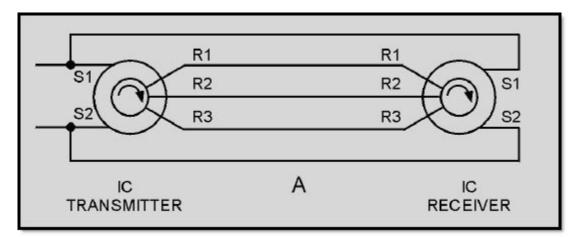
Figure 4-2A IC versus standard synchro connections
