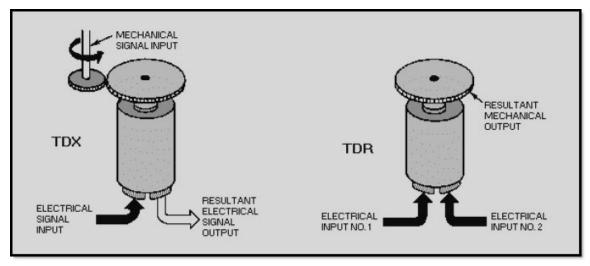
**Figure 1-18 Torque differentials**
