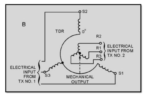
Figure 1-19B.—Torque differential receiver
