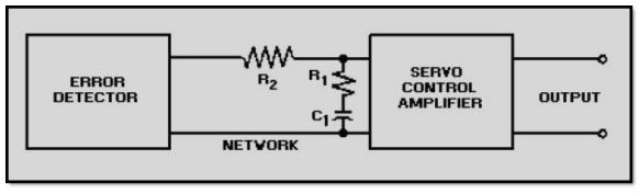
Figure 2-9 Error rate stabilization network using an RC integrator
