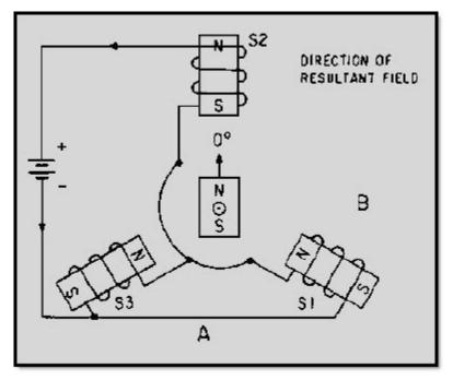
Figure 1-9 Operation of three electromagnets spaced 120° apart
