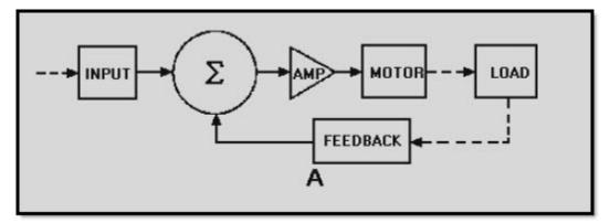
Figure 2-3A Block diagram of a position servo
