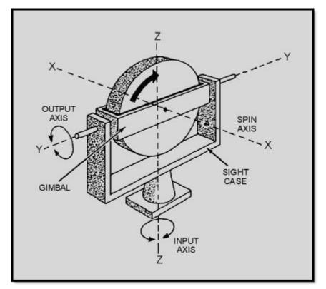
Figure 3-13 Rate gyro (single degree of freedom)
