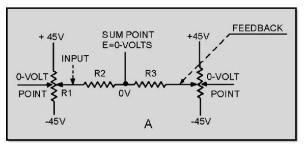
Figure 2-4A Development of the error signal
