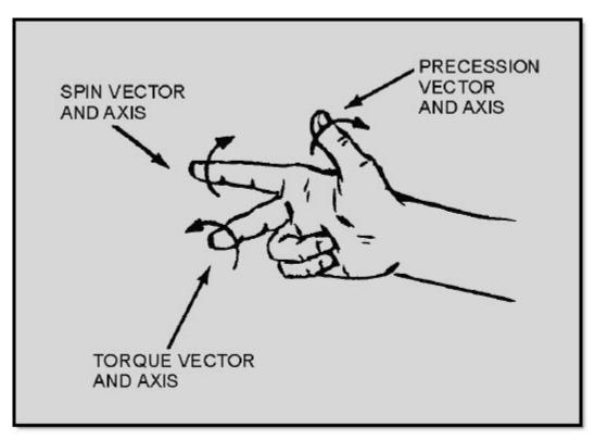
Figure 3-10 Right-hand rule for determining direction of precession
