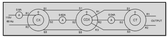
Figure 1-32 Synchro current in a control synchro system using a CDX and a CT
