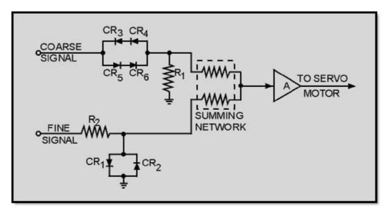
Figure 2-19 Semiconductor diode synchronizing network
