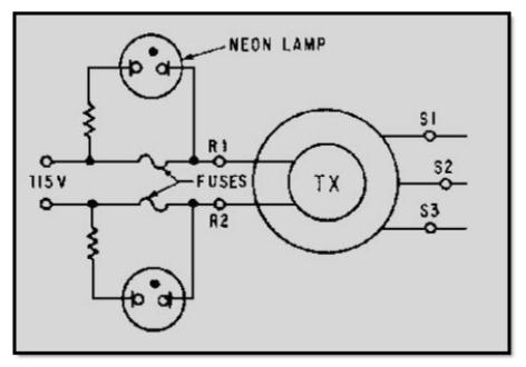
Figure 1-45 Simple blown fuse indicator
