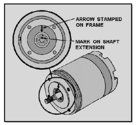
Figure 1-37 Coarse electrical zero markings
