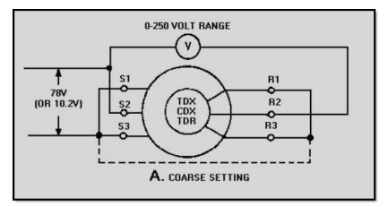
Figure 1-39A Zeroing differential synchros by the voltmeter method
