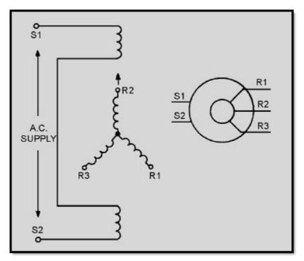
Figure 4-1 IC synchro schematic diagrams
