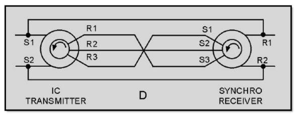
Figure 4-2D.—IC versus standard synchro connections
