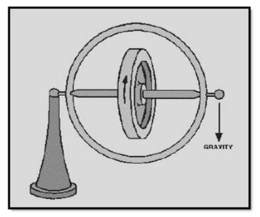
Figure 3-3 Gyro top with axis horizontal
