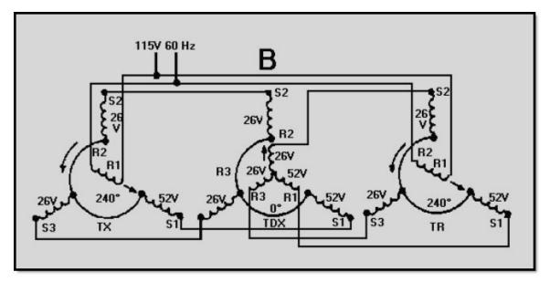
Figure 1-20B.—TX-TDX-TR system operation (subtraction)
