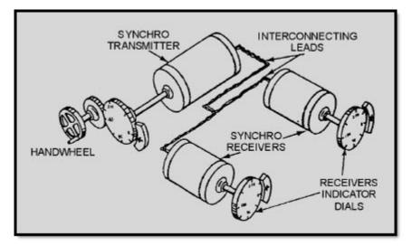
Figure 1-2 Data transfer with synchros
