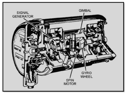
Figure 3-18 Rate gyro, cutaway view
