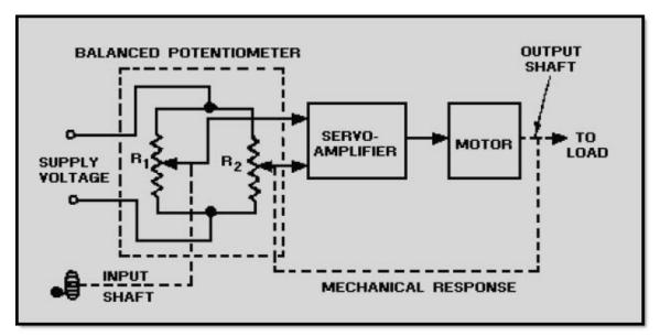
Figure 2-12 Balanced potentiometer used in position sensing
