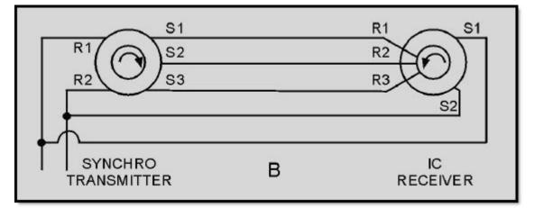
Figure 4-2B.—IC versus standard synchro connections
