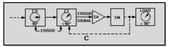
Figure 2-2C.—A basic servo system (closed-loop)
