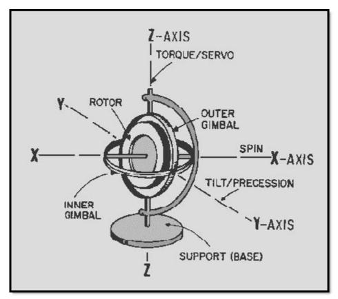
Figure 3-5 Basic universally mounted gyro
