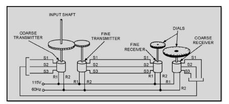
Figure 1-34 Dual-speed synchro system
