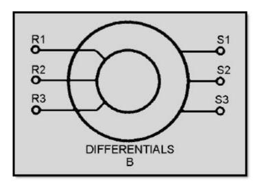
Figure 1-3B.—Schematic symbols for synchros
