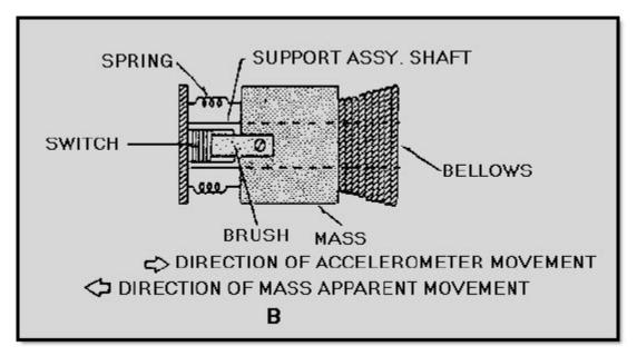
Figure 3-22B.—Pulse counting accelerometer
