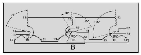
Figure 1-21B.—TX-TR system operation (addition)
