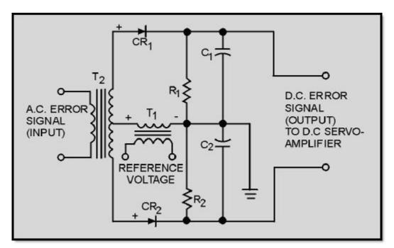
Figure 2-18 Diode demodulator
