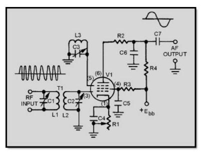
Figure 3-16 Gated-beam detector
