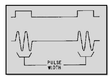
Figure 2-35 Pulse width (pw)
