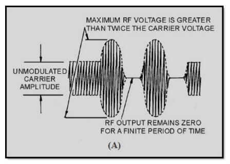
Figure 1-41A Overmodulation conditions
