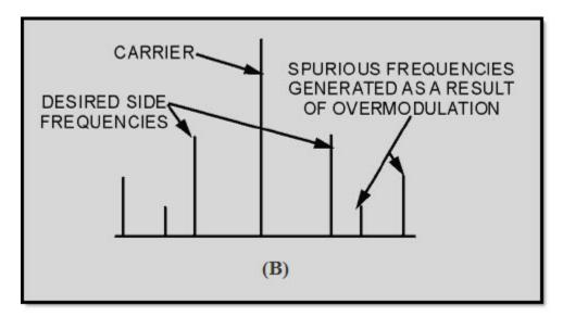
Figure 1-41B Overmodulation conditions
