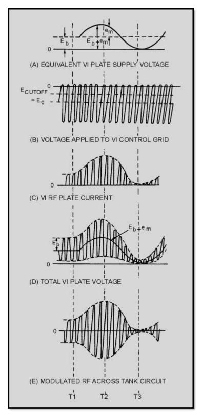
Figure 1-46 Plate-modulator waveforms
