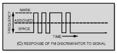
Figure 2-3C Comparison of AM and fm receiver response to an fm signal. RESPONSE OF FM DISCRIMINATOR TO SIGNAL
