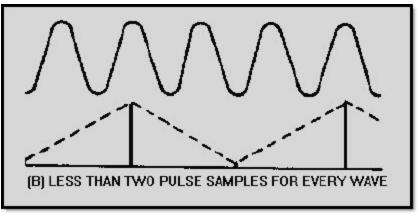
Figure 2-41B Pulse sampling rates. LESS THAN TWO PULSE SAMPLES FOR EVERY WAVE
