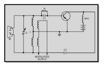
Figure 2A Oscillator circuit
