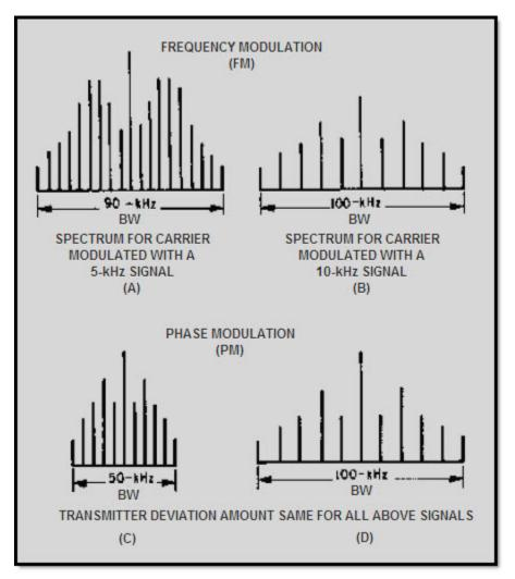
Figure 2-21 Fm versus pm spectrum distribution
