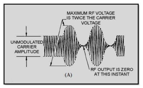
Figure 1-40A Conditions for 100-percent modulation
