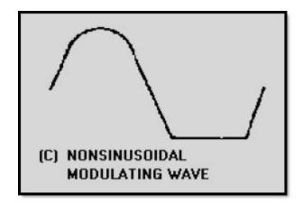
Figure 2-27C Overmodulation of a carrier. NONSINUSOIDAL MODULATING WAVE
