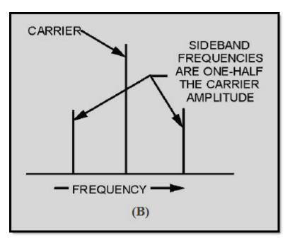
Figure 1-40B Conditions for 100-percent modulation
