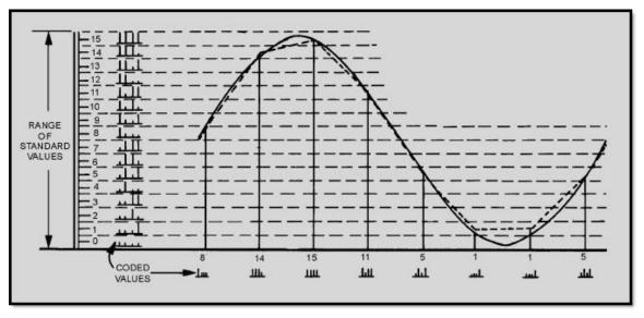
Figure 2-51 Pulse-code modulation of a quantized wave (32 bits)
