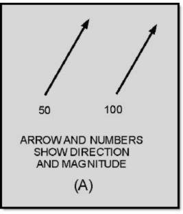
Figure 1-1A Vectors representing magnitude and direction
