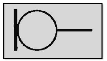
Figure 1-32 Microphone schematic symbol
