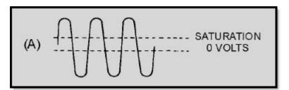
Figure 3-18A Gated-beam detector waveforms
