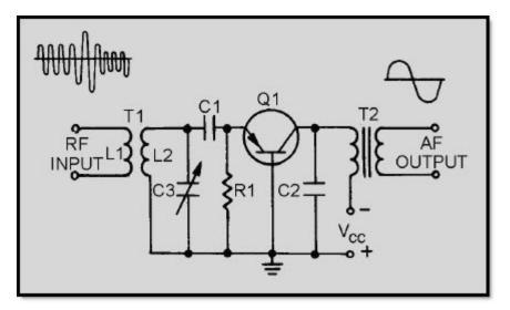
Figure 3-8 Common-base detector
