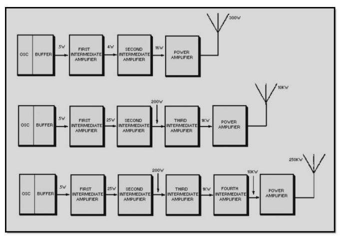
Figure 1-30 Block diagram of several medium-frequency transmitters
