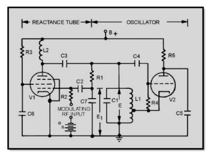
Figure 2-11 Reactance-tube fm modulator
