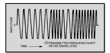
Figure 2-1D Comparison of ON-OFF and frequency-shift keying. TRANSMITTED FREQUENCY-SHIFT KEYED SIGNAL (FSK)
