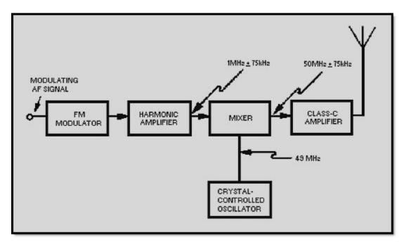
Figure 2-14 Method for improving frequency stability of fm system
