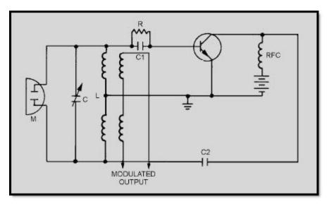
Figure 2-6 Oscillator circuit illustrating frequency modulation
