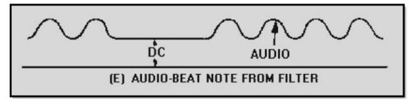
Figure 3-3E Heterodyne detection. AUDIO-BEAT NOTE FROM FILTER
