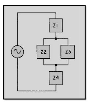
Figure 1-10 Sine wave generator applied to several impedances
