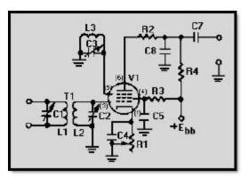
Figure 3H Gated-beam detector
