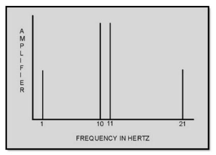
Figure 1-18 Spectrum analysis of heterodyned signal
