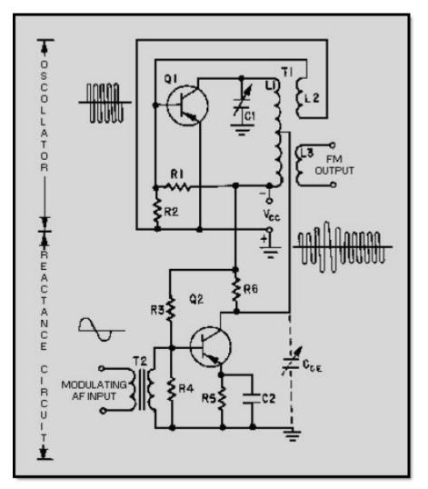
Figure 2-12 Reactance-semiconductor fm modulator
