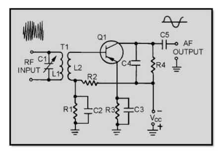
Figure 3-7 Common-emitter detector
