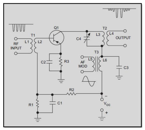
Figure 1-47 Collector-injection modulator
