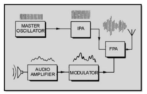
Figure 1-37 Block diagram of an AM transmitter
