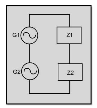
Figure 1-13 Two sine-wave generators with linear impedances
