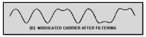
Figure 2-25D Phase-shift keying. MODULATED CARRIER AFTER FILTERING
