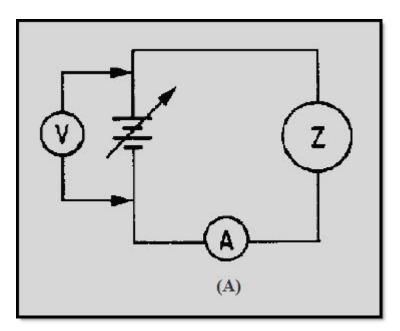
Figure 1-8A Nonlinear impedance circuit
