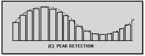
Figure 3-21C Peak detector. PEAK DETECTION
