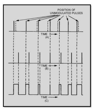
Figure 3-22 Conversion of ppm to pdm
