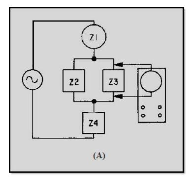
Figure 1-11A Circuit with nonlinear impedances
