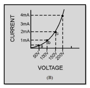
Figure 1-8B Nonlinear impedance circuit
