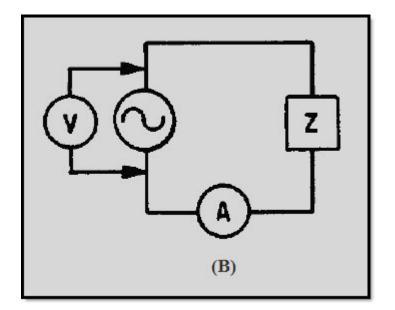
Figure 1-7B Linear impedance circuit
