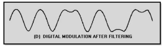
Figure 2-26D Simulated phase-shift keying. DIGITAL MODULATION AFTER FILTERING
