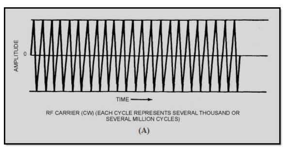
Figure 1-22A Essential elements of ON-OFF keying
