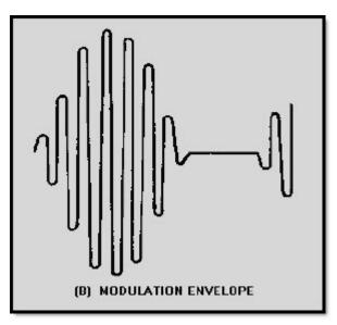
Figure 2-27B Overmodulation of a carrier. MODULATION ENVELOPE
