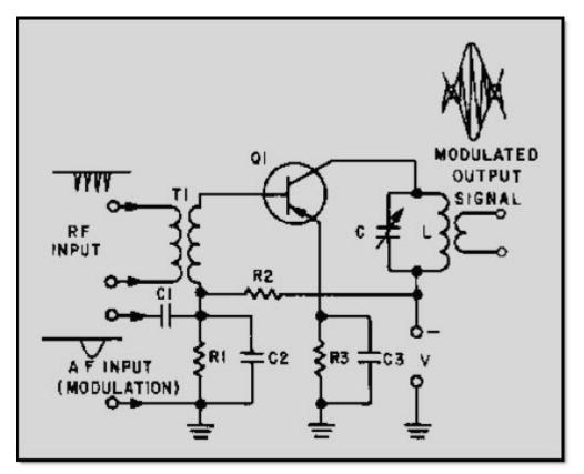
Figure 1-49 Base-injection modulator
