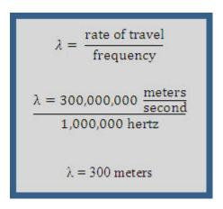
The *higher* the frequency, the *shorter* the wavelength of a sine wave. This important relationship between frequency and wavelength is illustrated in table 1-1.
