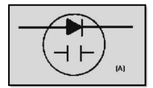
Figure 2-15 Varactor symbol and schematic. SCHEMATIC SYMBOL
