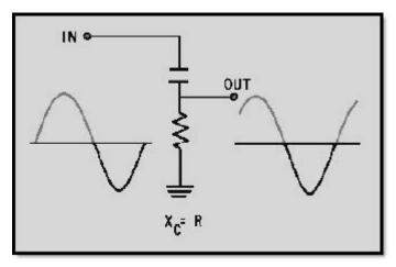
Figure 2-22 Phase shifting a sine wave
