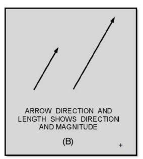
Figure 1-1B Vectors representing magnitude and direction
