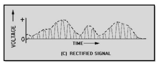
Figure 3-5C Series-diode detector and wave shapes. RECTIFIED SIGNAL
