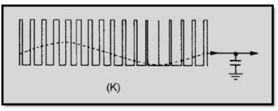
Figure 3-18K Gated-beam detector waveforms
