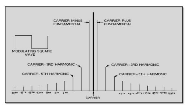
Figure 2-28 Spectrum distribution when modulating with a square wave
