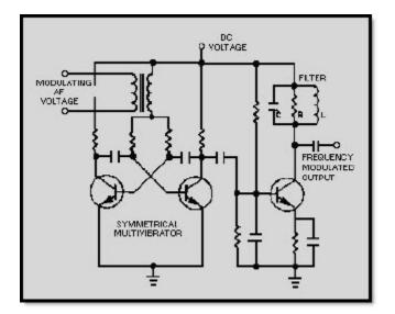
Figure 2D Multivibrator modulator
