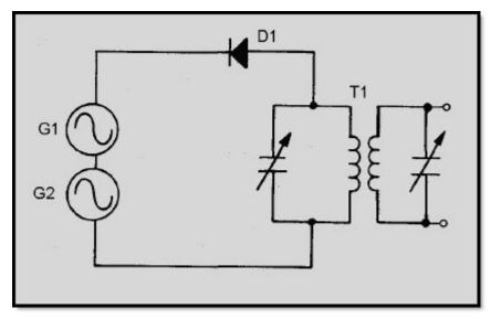
Figure 1-19 Typical heterodyning circuit
