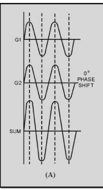
Figure 1-14A Waveforms across two nonlinear impedances
