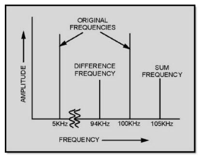
Figure 1-38 Radio-frequency spectrum
