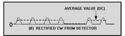
Figure 3-1B Cw demodulation. RECTIFIED CW FROM DETECTOR
