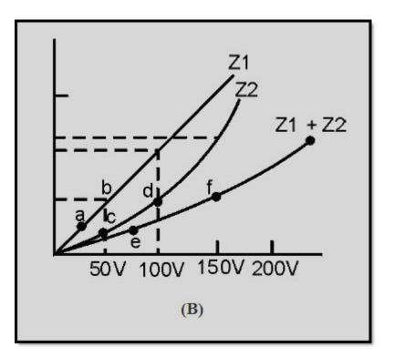
Figure 1-9B Combined linear and nonlinear impedances
