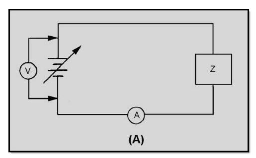
Figure 1-4A Circuit with one linear impedance
