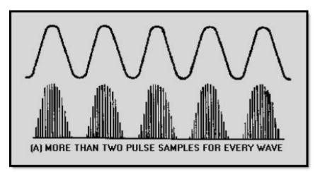
Figure 2-41A Pulse sampling rates. MORE THAN TWO PULSE SAMPLES FOR EVERY WAVE
