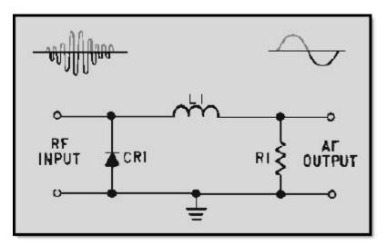
Figure 3-6 Shunt-diode detector
