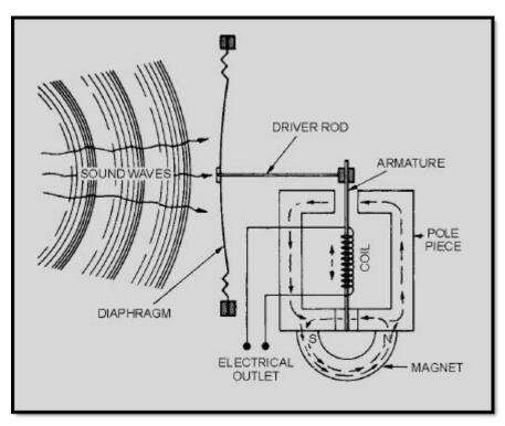
Figure 1-36 Magnetic microphone action
