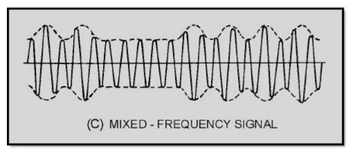
Figure 3-3C Heterodyne detection. MIXED-FREQUENCY SIGNAL
