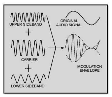
Figure 1-39 Formation of the modulation envelope
