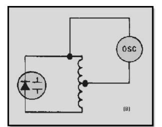
Figure 2-15B Varactor symbol and schematic. SIMPLIFIED CIRCUIT
