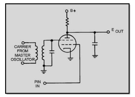
Figure 3-19 Phase detector
