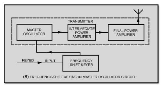
Figure 2-4B Two methods of frequency-shift keying (fsk). FREQUENCY-SHIFT KEYING IN MASTER OSCILLATOR CIRCUIT
