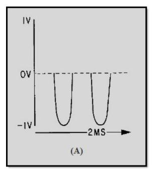
Figure 1-12A Waveform in a circuit with nonlinear impedances
