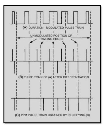
Figure 2-46 Pulse-position modulation (ppm)
