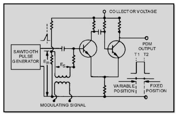
Figure 2-45 Circuit for producing pdm
