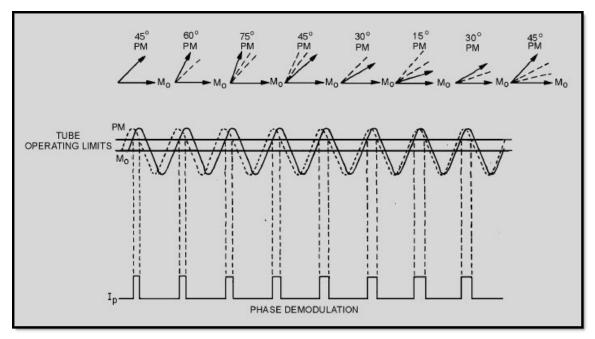
Figure 3-20 Phase-detector waveforms
