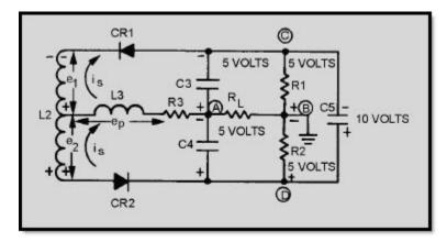
Figure 3-13 Current flow and polarities at resonance
