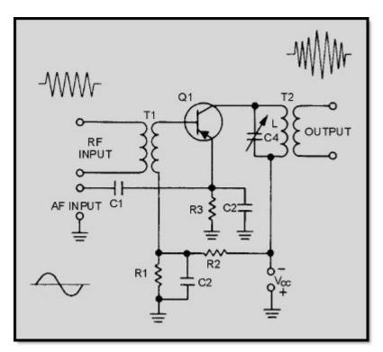
Figure 1-51 Emitter-injection modulator
