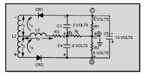
Figure 3-15 Current flow and polarities below resonance
