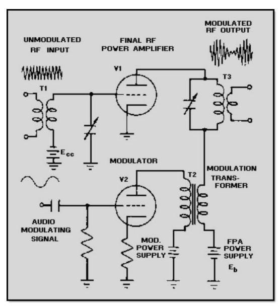
Figure 1-45 Plate-modulation circuit
