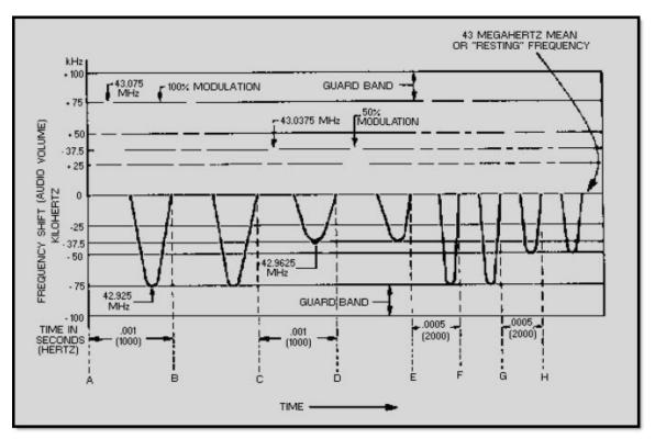
Figure 2-8 Frequency-modulating signal
