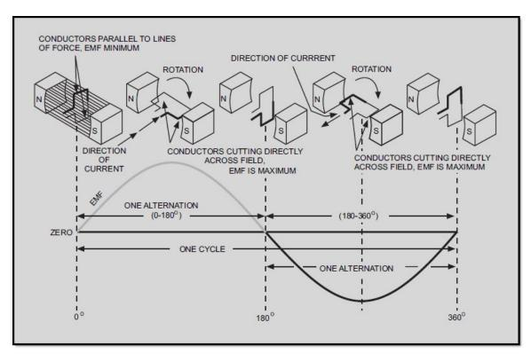
Figure 1-2 Sine-wave generator
