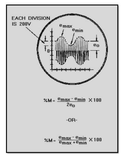
Figure 1-42 Computing percent of modulation from the modulation envelope
