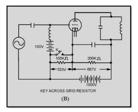
Figure 1-24B Blocked-grid keying
