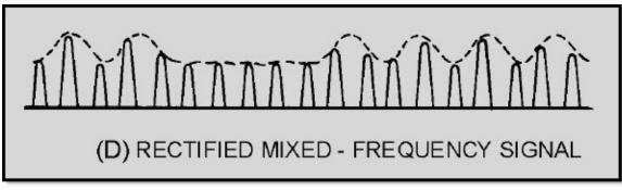
Figure 3-3D Heterodyne detection. RECTIFIED MIXED-FREQUENCY SIGNAL
