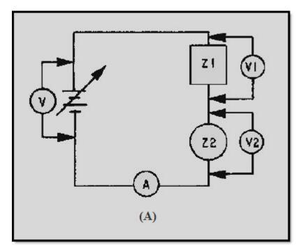
Figure 1-9A Combined linear and nonlinear impedances
