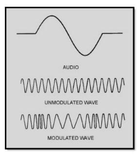
Figure 2-17 Phase modulation
