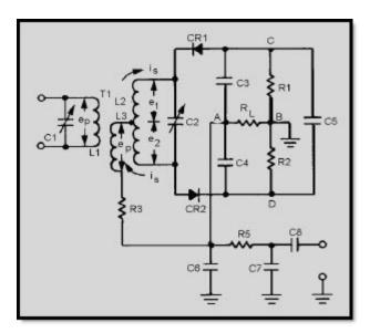
Figure 3G Ratio detector
