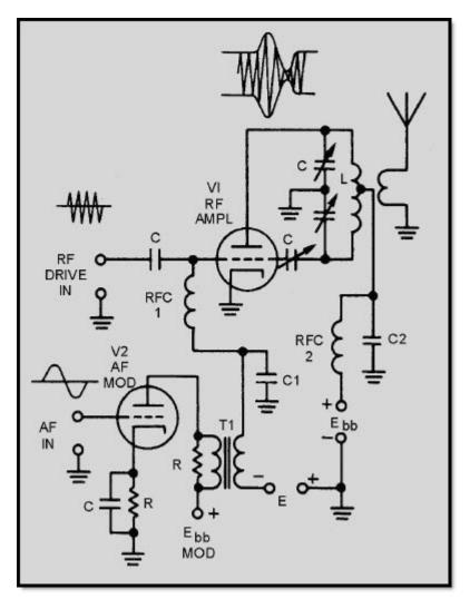
Figure 1-48 Control-grid modulator
