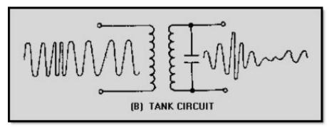
Figure 3-9B Slope detector. TANK CIRCUIT
