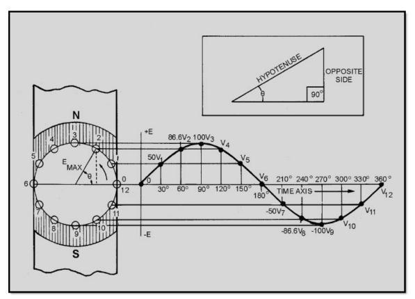
Figure 1-3 Generation of sine-wave voltage
