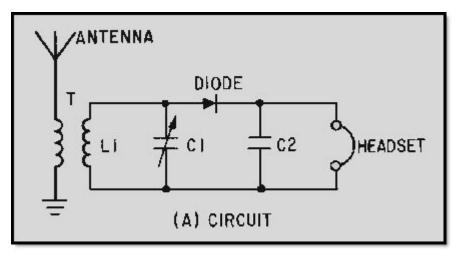
Figure 3-5A Series-diode detector and wave shapes. CIRCUIT
