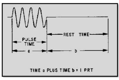
Figure 2-34 Pulse cycles
