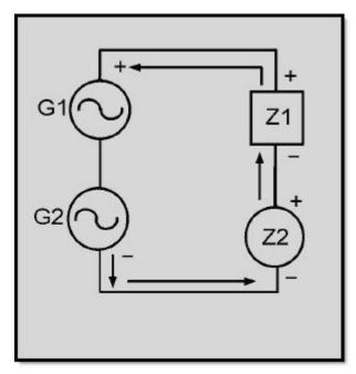
Figure 1-16 Sine-wave generators with a combination of impedances
