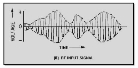
Figure 3-5B Series-diode detector and wave shapes. RF INPUT SIGNAL
