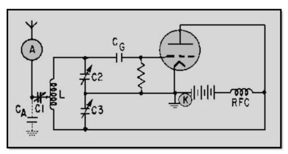
Figure 1-28 Simple electron-tube transmitter
