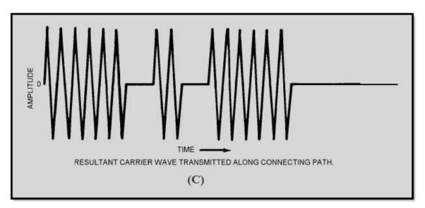
Figure 1-22C Essential elements of ON-OFF keying
