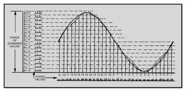
Figure 2-50 Pulse-code modulation of a quantized wave (128 bits)
