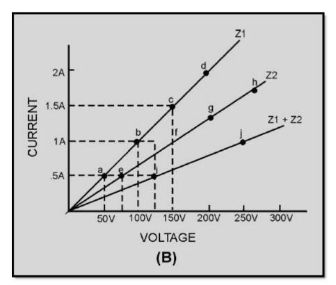
Figure 1-5B Circuit with two linear impedances
