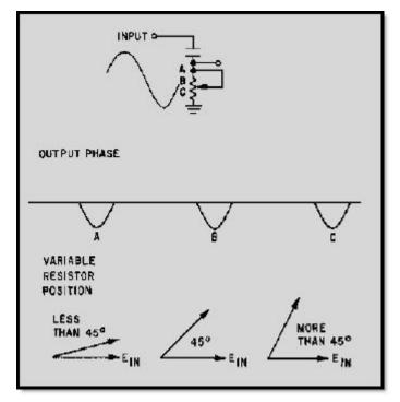
Figure 2-23 Control over the amount of phase shift
