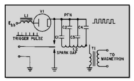
Figure 2-38 Fixed spark-gap modulator
