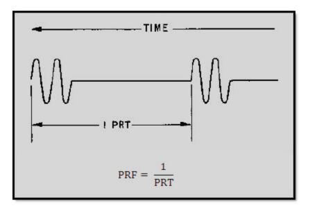
Figure 2-33 Pulse-repetition time (prt)
