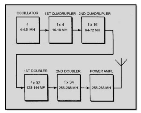
Figure 1-31 Block diagram of a vhf transmitter
