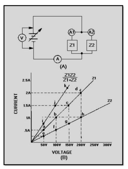
Figure 1-6 Circuit with parallel linear impedances
