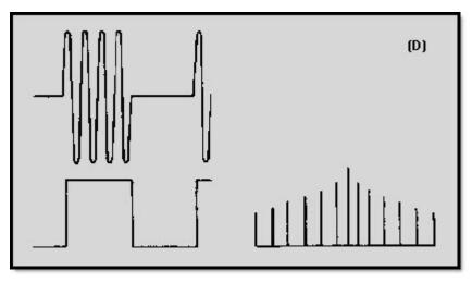
Figure 2-29D Various square-wave modulation levels with frequencyspectrum carrier and sidebands
