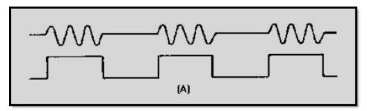
Figure 2-30A Pulse transmission
