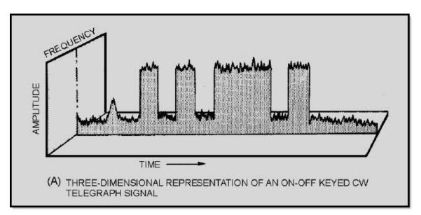
Figure 2-2A Comparison of AM and fm receiver response to an AM signal. THREE-DIMENSIONAL REPRESENTATION OF AN ON-OFF KEYED CW TELEGRAPH SIGNAL
