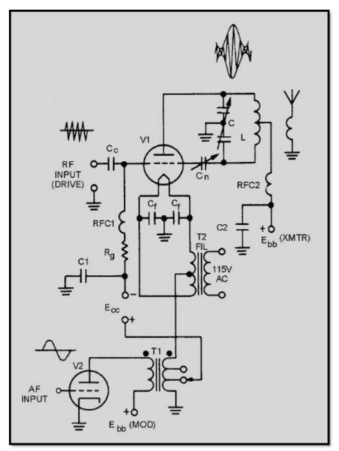
Figure 1-50 Cathode modulator
