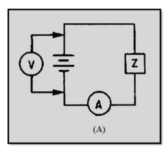
Figure 1-7A Linear impedance circuit
