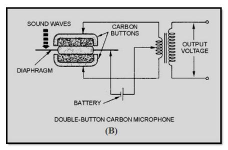
Figure 1-33B Carbon microphones. DOUBLE-BUTTON CARBON MICROPHONE
