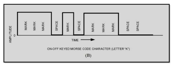
Figure 1-22B Essential elements of ON-OFF keying
