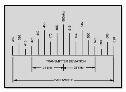
Figure 2-10 Frequency deviation versus bandwidth
