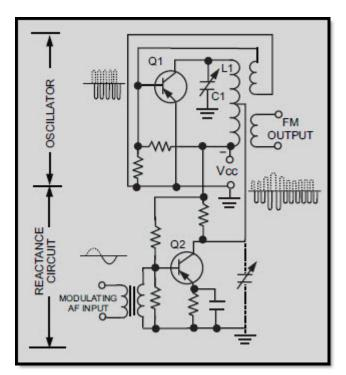
Figure 2C Semiconductor reactance modulator
