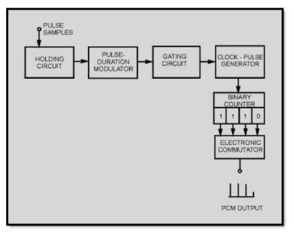
Figure 2-52 Block diagram of quantizer and pcm coder
