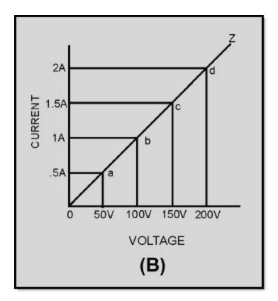
Figure 1-4B Circuit with one linear impedance
