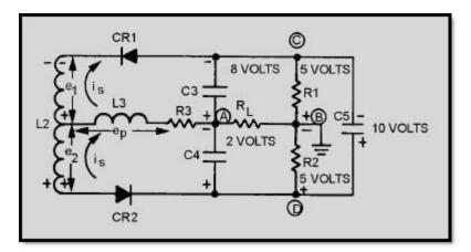
Figure 3-14 Current flow and polarities above resonance
