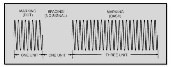
Figure 1-21 Dot and dash in radiotelegraph code
