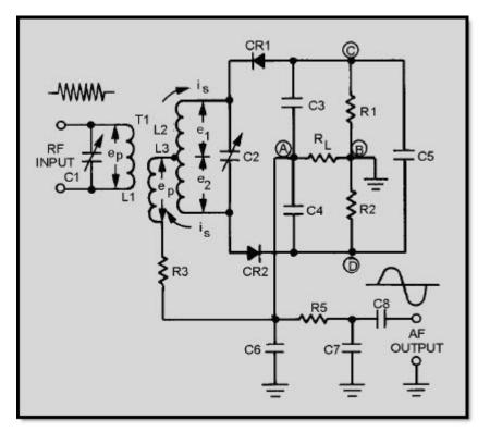
Figure 3-12 Ratio detector
