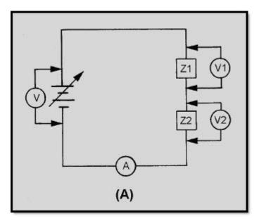
Figure 1-5A Circuit with two linear impedances
