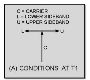
Figure 1-44A Vector diagrams for T1 and T2
