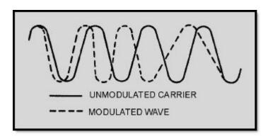
Figure 2-19 Carrier with and without modulation
