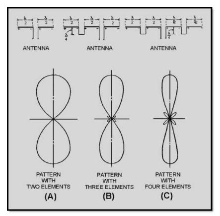
Figure 3-14 Horizontal array field patterns
