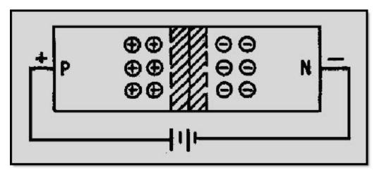
Figure 2-42C Pn-junction diode as a variable capacitor
