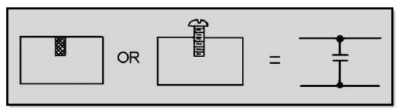
Figure 1-43A Conducting posts and screws. PENETRATING
