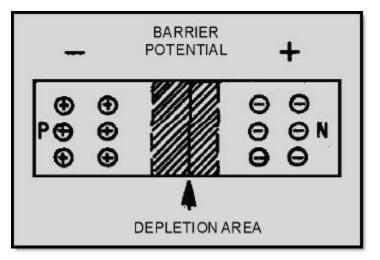
Figure 2-42A Pn-junction diode as a variable capacitor
