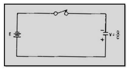
Figure 2-43 Voltage amplification from a varying capacitor
