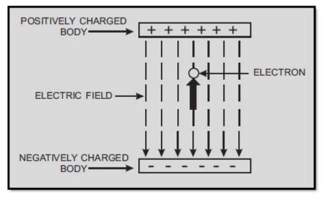
Figure 2-2 Moving electron gaining velocity and energy
