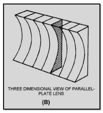
Figure 3-10B Waveguide lens
