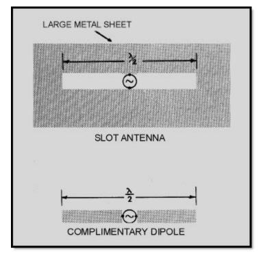
Figure 3-18 Slot antenna and complementary dipole
