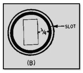
Figure 1-51B Choke joint
