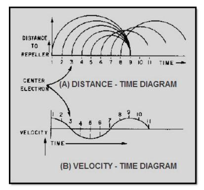
Figure 2-10 Electron bunching diagram
