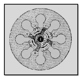
Figure 2-33 Rotating space-charge wheel in an eightcavity magnetron
