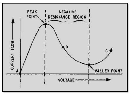
Figure 2-39 Tunnel-diode characteristic curve
