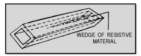
Figure 1-45C Terminating waveguides
