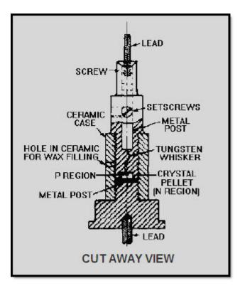
Figure 2-51C Point-contact diode. CUT AWAY VIEW
