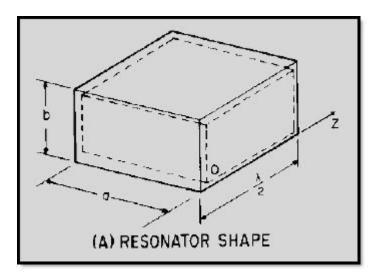
Figure 1-58A Rectangular waveguide cavity resonator. RESONATOR SHAPE
