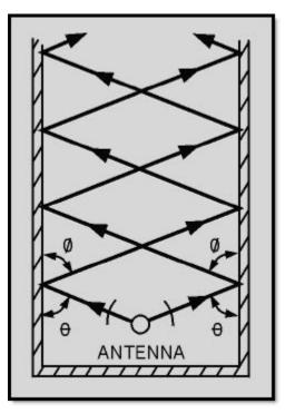
Figure 1-27B Different frequencies in a waveguide
