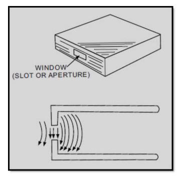
Figure 1-41 Slot coupling in a waveguide
