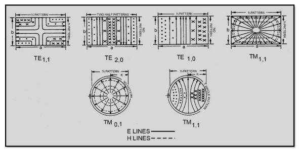
Figure 1-38 Various modes of operation for rectangular and circular waveguides
