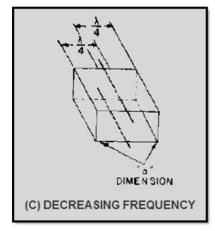
Figure 1-10C Frequency effects on a waveguide. DECREASING FREQUENCY
