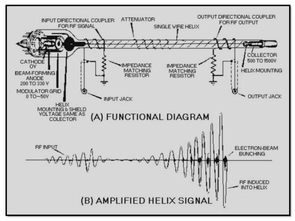
Figure 2-15 Functional diagram of a twt
