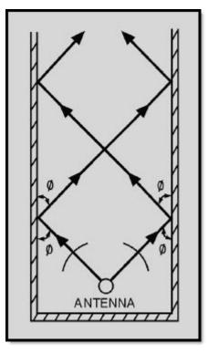
1-27 Different frequencies in a waveguide
