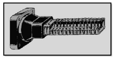
Figure 1-50 Flexible waveguide
