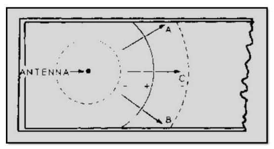
Figure 1-24 Radiation from probe placed in a waveguide
