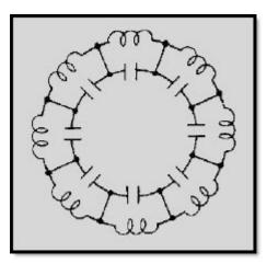
Figure 2-30 Cavities connected in series
