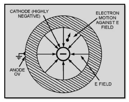
Figure 2-19 Electron motion in an electric field
