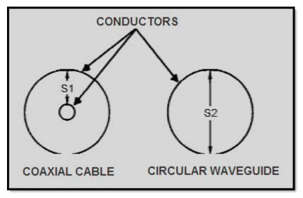
Figure 1-4 Comparison of spacing in coaxial cable and a circular waveguide
