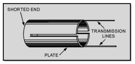
Figure 2-25 Plate tank circuit of a magnetron
