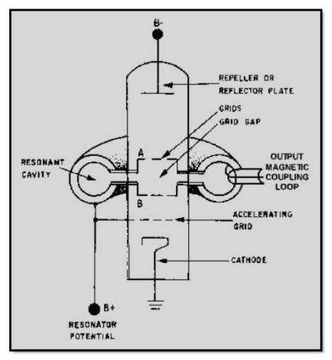
Figure 2-9 Functional diagram of a reflex klystron
