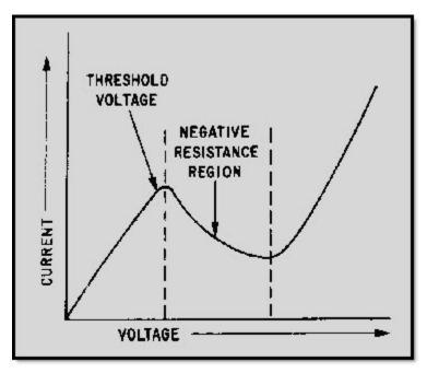
Figure 2-48 Characteristic curve for a bulk-effect semiconductor
