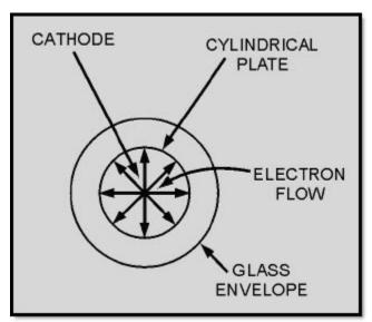
Figure 2-21B Basic magnetron. END VIEW OMITTING MAGNETS
