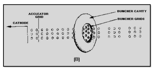
Figure 2-4B Electron gun with buncher grids
