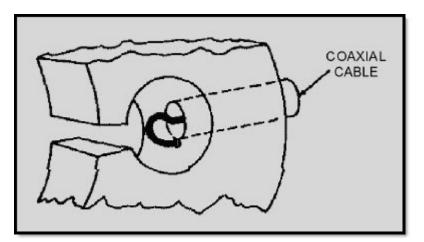
Figure 2-35A Magnetron coupling methods
