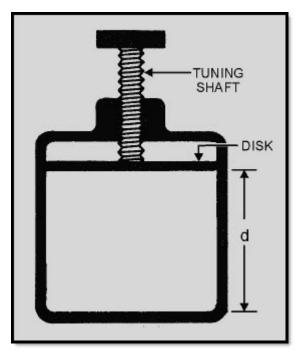
Figure 1-62 Cavity tuning by volume
