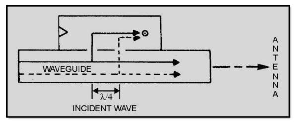
Figure 1-54 Incident wave in a directional coupler designed to sample incident waves
