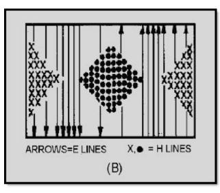
Figure 1-34B Waveguide operation in other than dominant mode
