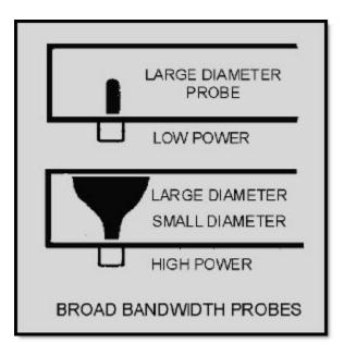
Figure 1-39D Probe coupling in a rectangular waveguide
