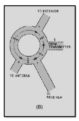
Figure 1-71B Hybrid ring with wavelength measurements
