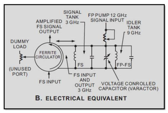
Figure 2-45B Nondegenerative parametric amplifier. ELECTRICAL EQUIVALENT
