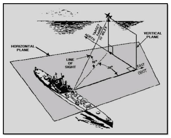
Figure 3-1 Radar target position
