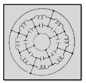
Figure 2-31 Cavities in parallel because of strapping
