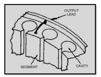
Figure 2-35C Magnetron coupling methods
