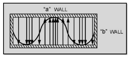
Figure 1-31 One and one-half sine E field distribution
