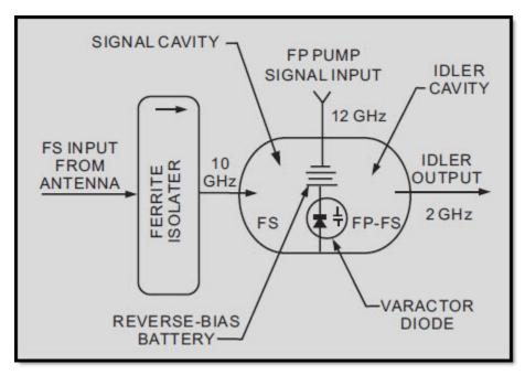
Figure 2-47 Lower-sideband parametric down-converter
