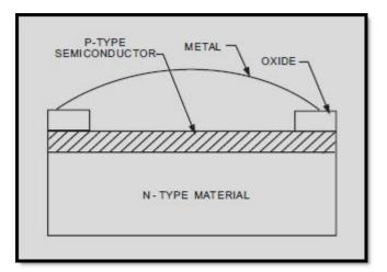
Figure 2-52 Schottky-barrier diode
