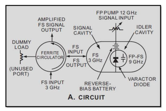
Figure 2-45A Nondegenerative parametric amplifier. CIRCUIT
