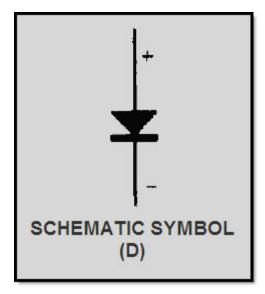
Figure 2-51D Point-contact diode. SCHEMATIC SYMBOL
