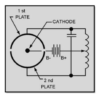
Figure 2-23B Split-anode magnetron
