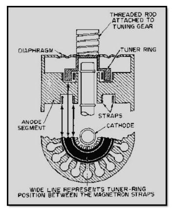
Figure 2-37 Capacitive magnetron tuning
