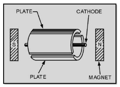
Figure 2-23A Split-anode magnetron
