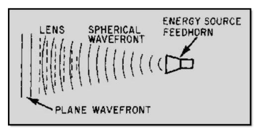
Figure 3-11 Delay-type lens
