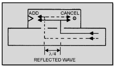
Figure 1-55 Reflected wave in a directional coupler
