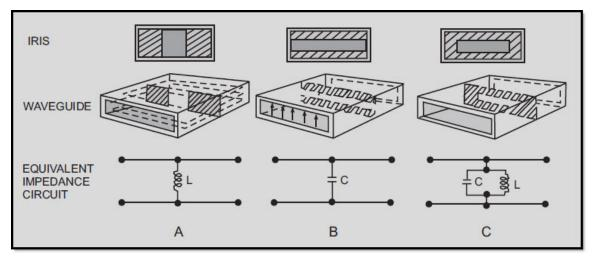
Figure 1-42 Waveguide irises
