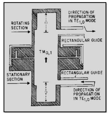
Figure 1-52 Rotating joint
