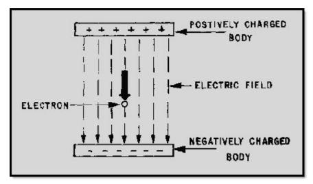
Figure 2-3 Moving electron losing energy and velocity
