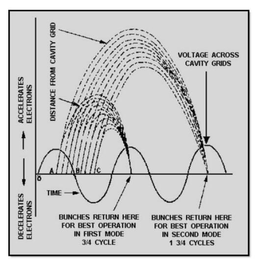
Figure 2-11 Bunching action of a reflex klystron
