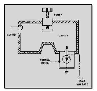
Figure 2-40 Tunnel-diode oscillator
