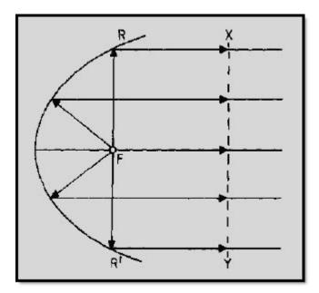
Figure 3-2 Parabolic reflector radiation
