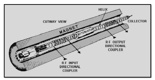
Figure 2-13 Physical construction of a twt
