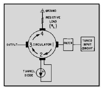
Figure 2-41 Tunnel-diode amplifier
