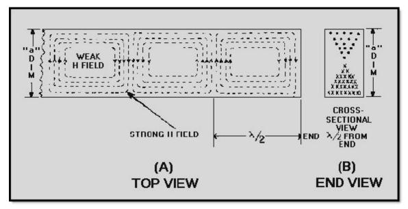
Figure 1-18 Magnetic field in a waveguide three half-wavelengths long
