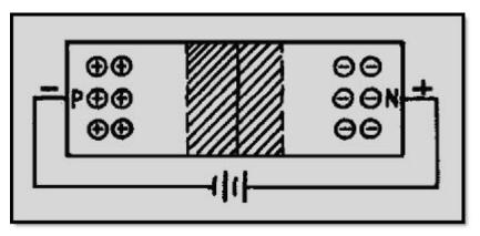
Figure 2-42B Pn-junction diode as a variable capacitor
