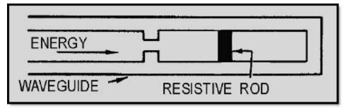
Figure 1-45B Terminating waveguides
