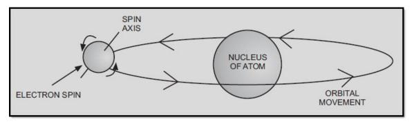
Figure 1-73 Two types of electron movement
