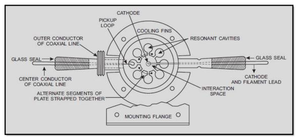
Figure 2-18 Cutaway view of a magnetron
