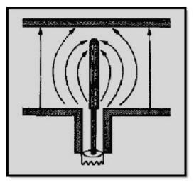
Figure 1-39A Probe coupling in a rectangular waveguide
