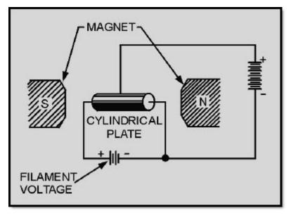
Figure 2-21A Basic magnetron. SIDE VIEW
