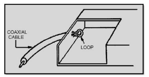
Figure 1-40A Loop coupling in a rectangular waveguide
