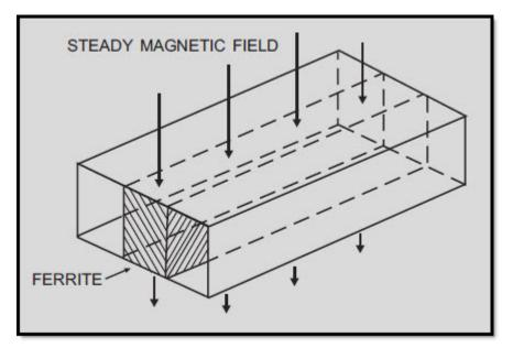
Figure 1-72 Ferrite attenuator
