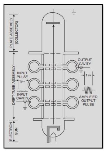
Figure 2-8 Three-cavity klystron
