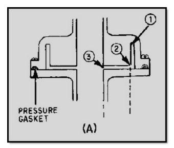
Figure 1-51A Choke joint
