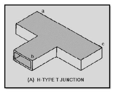
Figure 1-65A E fields in an H-type junction. H-TYPE T JUNCTION
