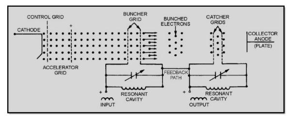
Figure 2-7B Functional and schematic diagram of a two-cavity klystron
