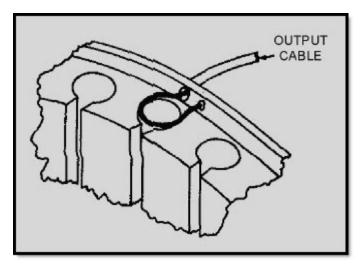
Figure 2-35B Magnetron coupling methods
