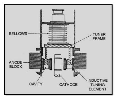
Figure 2-36 Inductive magnetron tuning
