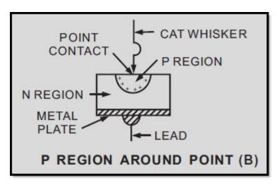
Figure 2-51B Point-contact diode. P REGION AROUND POINT
