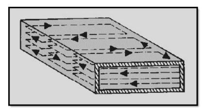
Figure 1-32 Magnetic field caused by a half-sine E field
