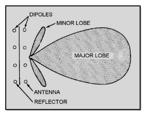
Figure 3-13 Field pattern of an antenna array
