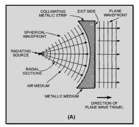
Figure 3-10A Waveguide lens
