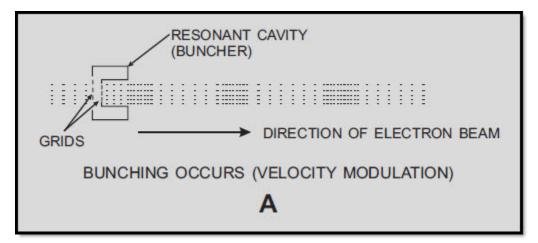
Figure 2-6A Removing energy from a velocity-modulated beam
