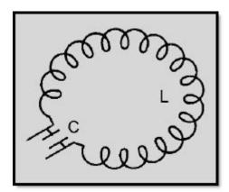
Figure 2-29B Equivalent circuit of a hole-and-slot cavity
