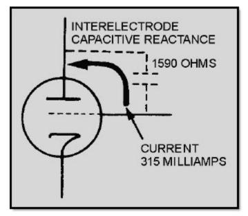
Figure 2-1B Interelectrode capacitance in a vacuum tube. 100 MEGAHERTZ
