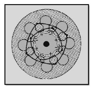
Figure 2-34 Alternate segments connected by strapping rings
