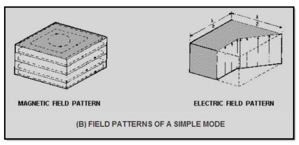
Figure 1-58B Rectangular waveguide cavity resonator. FIELD PATTERNS OF A SIMPLE MODE
