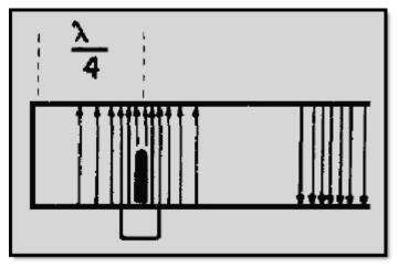
Figure 1-39B Probe coupling in a rectangular waveguide
