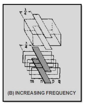
Figure 1-10B Frequency effects on a waveguide. INCREASING FREQUENCY
