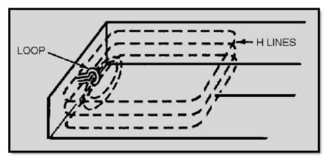
Figure 1-40B Loop coupling in a rectangular waveguide
