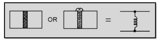
Figure 1-43B Conducting posts and screws. EXTENDING THROUGH
