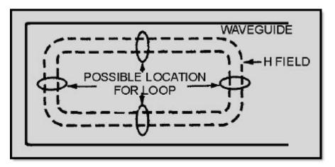
Figure 1-40C Loop coupling in a rectangular waveguide
