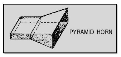
Figure 1-44C Waveguide horns. PYRAMID HORN
