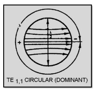
Figure 1-37 Counting wavelengths in a circular waveguide
