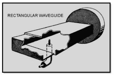
Figure 1-39C Probe coupling in a rectangular waveguide
