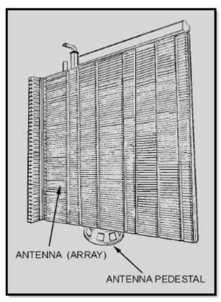
Figure 3-16 Frequency-sensitive antenna
