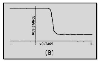
Figure 2-53B Diode equivalent circuit (pin)
