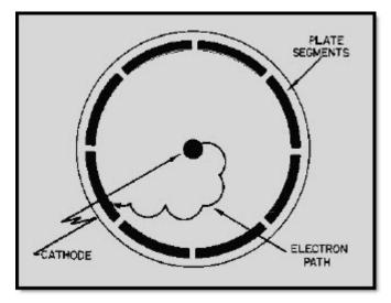
Figure 2-26 Electron path in an electron-resonance magnetron
