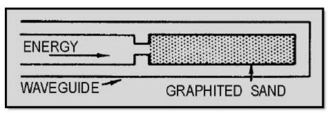
Figure 1-45A Terminating waveguides
