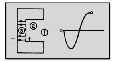
Figure 2-5D Buncher cavity action. ELECTRON #3 ACCELERATED
