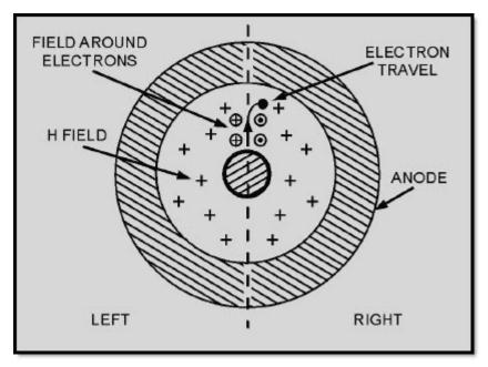
Figure 2-20 Electron motion in a magnetic field
