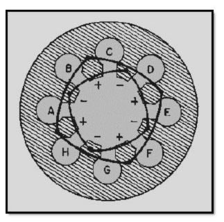
Figure 2-28 Strapping alternate segments
