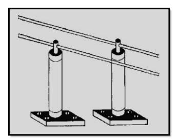
Figure 1-5 Two-wire transmission line using ordinary insulators
