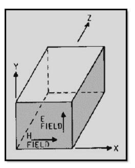
Figure 1-61 Rectangular cavity resonator
