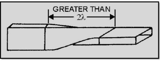
Figure 1-49 Waveguide twist
