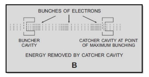
Figure 2-6B Removing energy from a velocity-modulated beam
