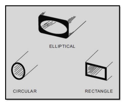
Figure 1-3 Waveguide shapes
