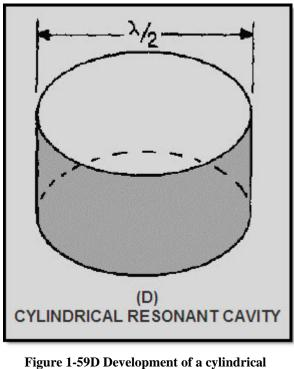
resonant cavity. CYLINDRICAL RESONANT CAVITY
