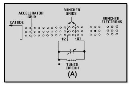
Figure 2-4A Electron gun with buncher grids
