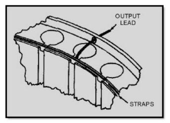
Figure 2-35D Magnetron coupling methods
