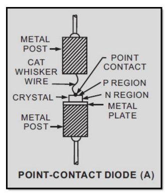
Figure 2-51A Point-contact diode. P REGION AROUND POINT
