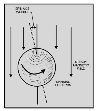
Figure 1-74 Electron wobble in a magnetic field
