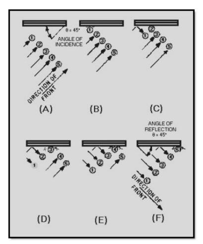
Figure 1-26 Reflection of a single wavefront
