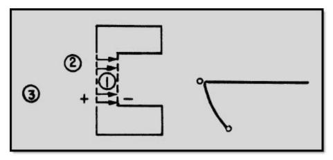
Figure 2-5B Buncher cavity action. ELECTRON #1 DECELERATED
