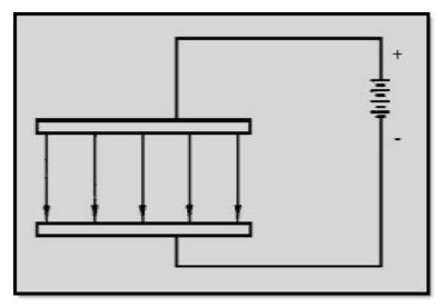
Figure 1-11A Simple electric fields. CAPACITOR
