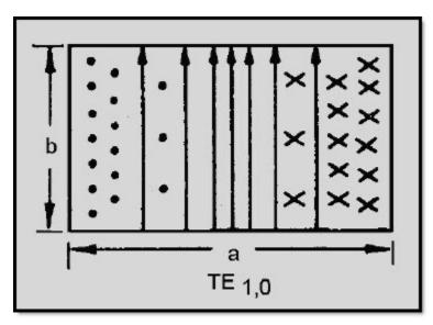
Figure 1-36 Dominant mode in a rectangular waveguide
