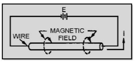
Figure 1-14 Magnetic field on a single wire
