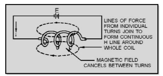
Figure 1-15 Magnetic field on a coil
