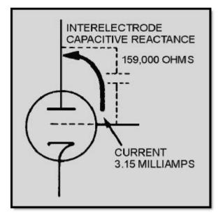
Figure 2-1A Interelectrode capacitance in a vacuum tube. 1 MEGAHERTZ
