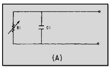
Figure 2-53A Diode equivalent circuit (pin)
