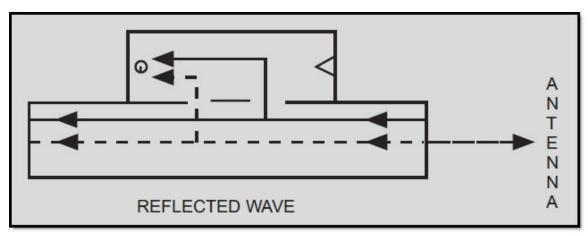
Figure 1-56 Directional coupler designed to sample reflected energy
