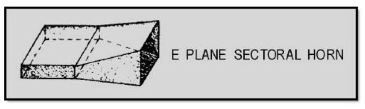
Figure 1-44A Waveguide horns. E PLANE SECTORAL HORN
