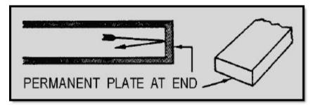
Figure 1-45D Terminating waveguides
