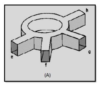
Figure 1-71 A Hybrid ring with wavelength measurements
