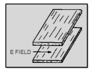
Figure 1-19B E field boundary condition. DOES NOT MEET BOUNDARY
