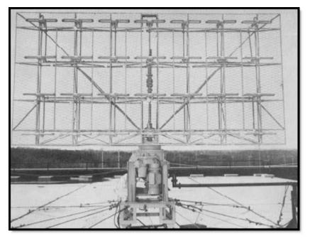
Figure 3-15 Bedspring array
