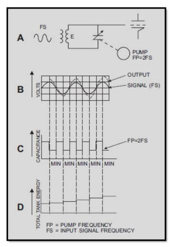
Figure 2-44 Energy transfer from pump signal to input signal
