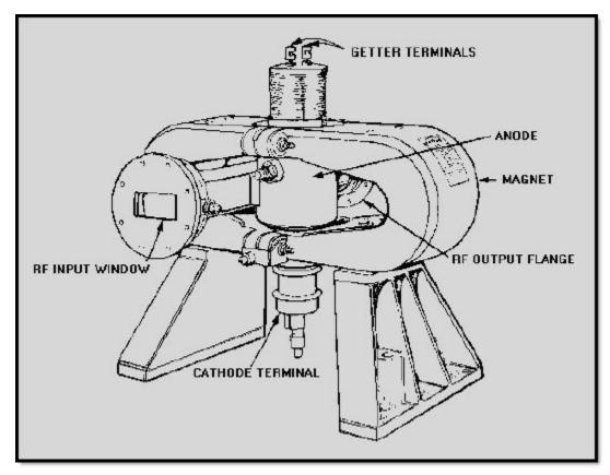
Figure 2-38 Crossed-field amplifier (Amplitron)
