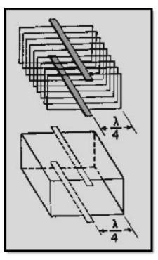
Figure 1-8 Forming a waveguide by adding quarter-wave sections
