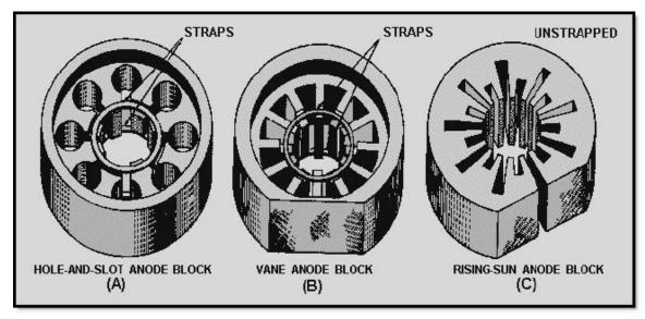
Figure 2-27 Common types of anode blocks
