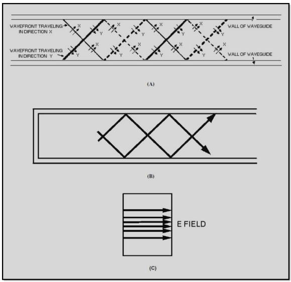
Figure 1-25 Wavefronts in a waveguide
