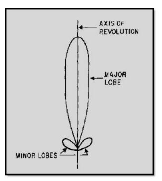
Figure 3-3 Parabolic radiation pattern
