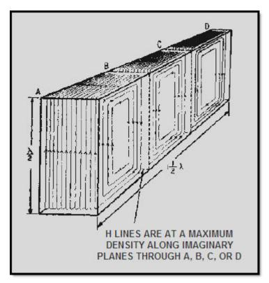
Figure 1-17 Magnetic field pattern in a waveguide
