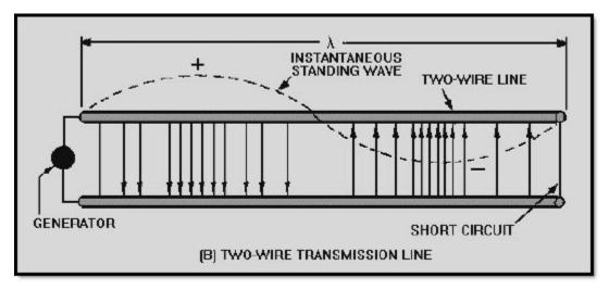
Figure 1-11B Simple electric fields. TWO-WIRE TRANSMISSION LINE
