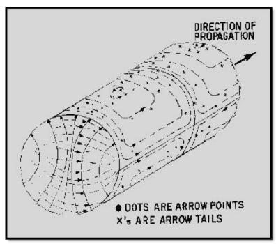
Figure 1-35 Dominant mode in a circular waveguide
