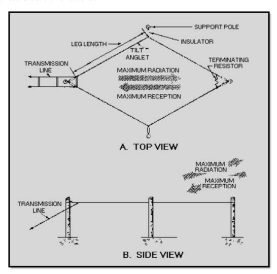
Figure 4-37 Basic rhombic antenna
