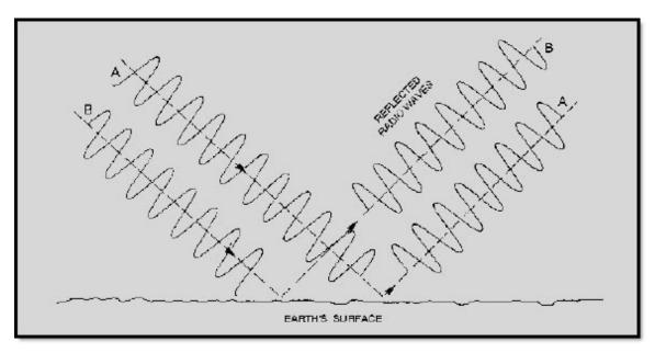
Figure 2-7 Phase shift of reflected radio waves
