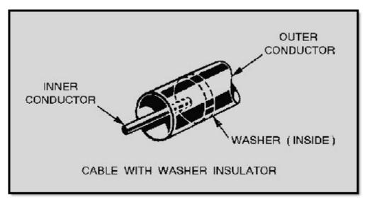
Figure 3-6 Air coaxial line
