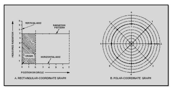
Figure 4-10 Comparison of rectangular- and polar-coordinate graphs for an isotropic source
