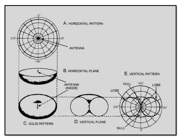
Figure 4-14 Development of vertical and horizontal patterns
