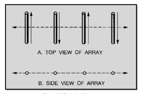
Figure 4-28 Typical end-fire array
