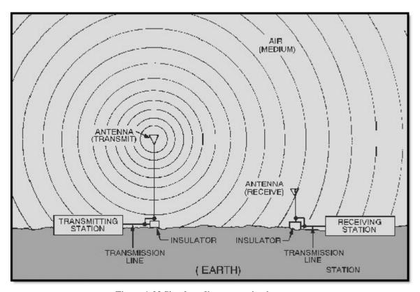
Figure 1-23 Simple radio communication system
