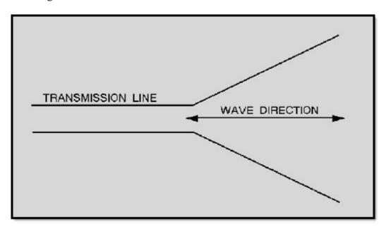
Figure 4-35 Basic V antenna
