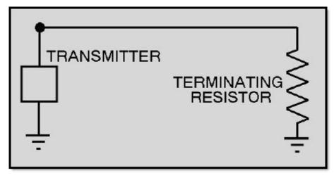
Figure 4-34 Beverage antenna
