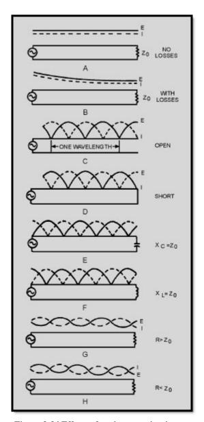
Figure 3-34 Effects of various terminations on standing waves
