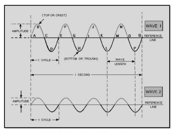
Figure 1-7 Comparison of waves with different amplitudes
