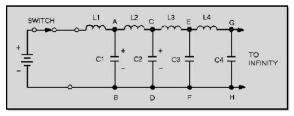
Figure 3-20 Dc applied to an equivalent transmission line
