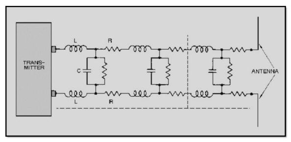
Figure 3-9 Equivalent circuit of a two-wire transmission line
