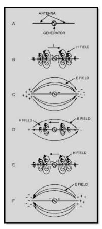
Figure 2-1 Induction field about an antenna
