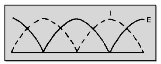
Figure 3-28 Conventional picture of standing waves
