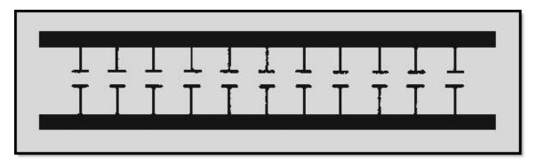
Figure 3-11 Distributed capacitance
