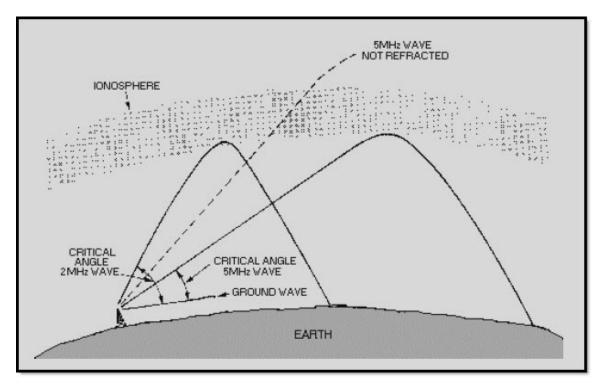
Figure 2-18 Effects of frequency on the critical angle
