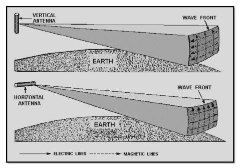
Figure 2-5 Vertical and horizontal polarization
