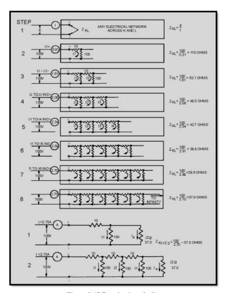
Figure 3-17 Termination of a line
