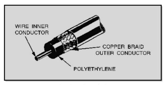
Figure 3-7 Flexible coaxial line
