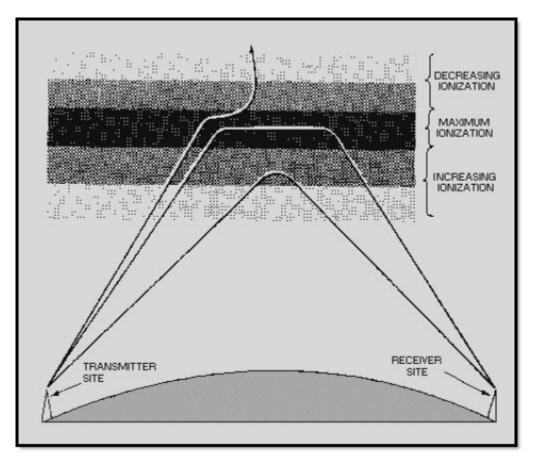
Figure 2-15 Effects of ionospheric density on radio waves
