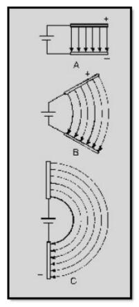
Figure 1-26 Electric fields between plates at different angles
