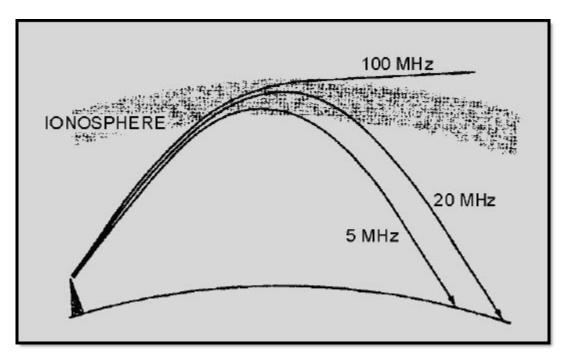
Figure 2-16 Frequency versus refraction and distance
