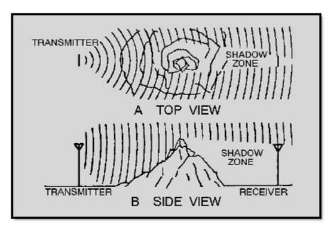
Figure 2-9 Diffraction around an object
