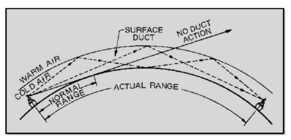
Figure 2-25 Duct effect caused by temperature inversion
