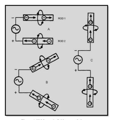
Figure 1-28 Magnetic fields around elements
