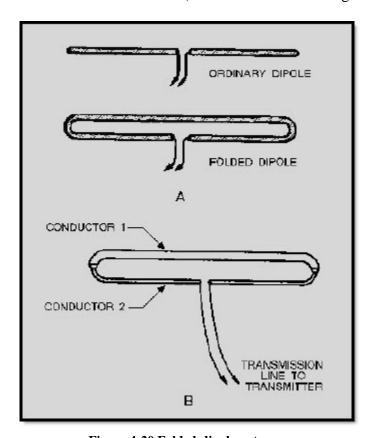
Figure 4-20 Folded-dipole antennas
