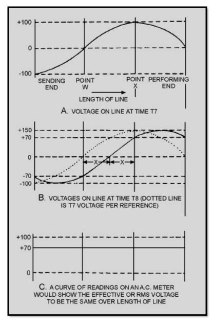
Figure 3-22 Instantaneous voltages along a transmission line
