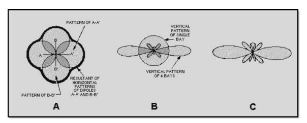
Figure 4-39 Turnstile antenna radiation pattern
