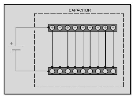
Figure 1-25 Electric fields between plates
