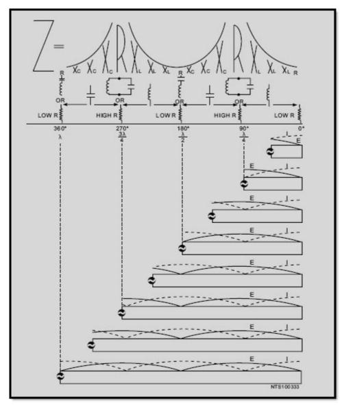
Figure 3-33 Voltage, current, and impedance on shorted line
