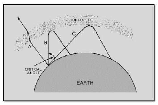
Figure 2-17 Different incident angles of radio waves
