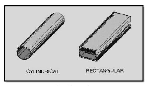
Figure 3-8 Waveguides
