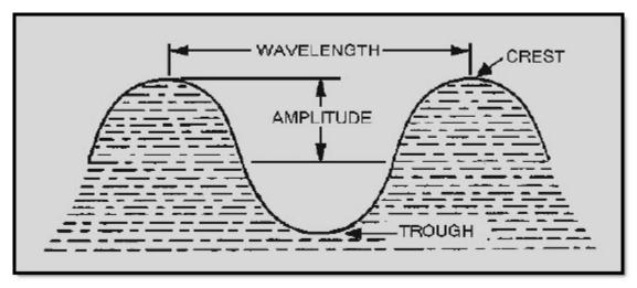
Figure 1-3 Elements of a wave
