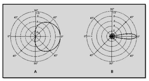
Figure 4-30 Unidirectional end-fire arrays
