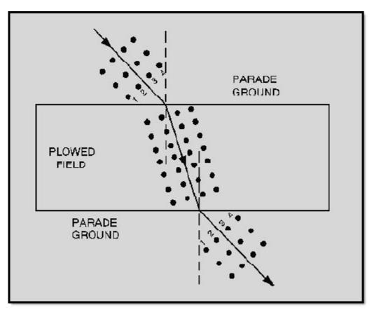
Figure 1-11 Analogy of refraction
