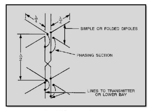
Figure 4-40 Stacked turnstile antennas
