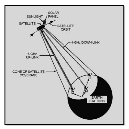
Figure 4-1 Satellite/earth station communications system
