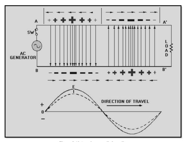
Figure 3-19 Ac voltage applied to a line
