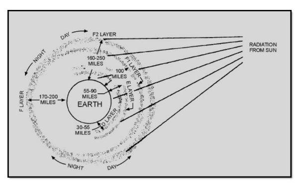
Figure 2-14 Layers of the ionosphere
