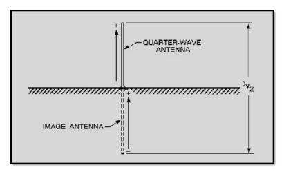
Figure 4-18 Grounded quarter-wave antenna image
