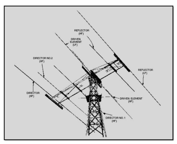
Figure 4-33 A typical parasitic array used for transmitting and receiving
