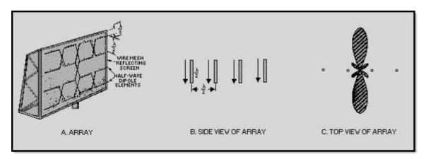
Figure 4-26 Typical broadside array
