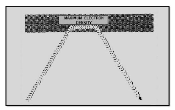
Figure 2-8 Radio wave refraction
