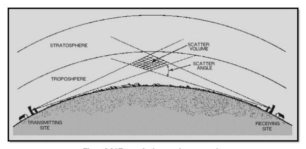
Figure 2-26 Tropospheric scattering propagation
