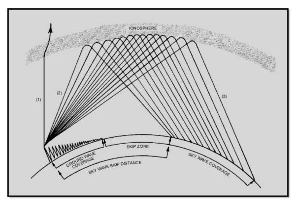
Figure 2-19 Relationship between skip zone, skip distance, and ground wave
