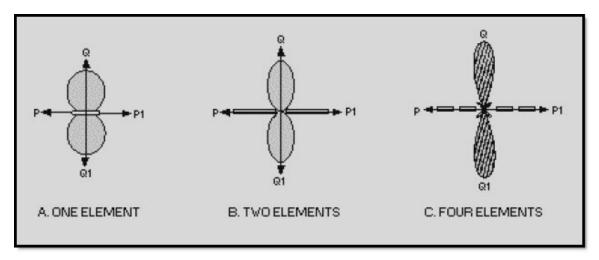
Figure 4-25 Single half-wave antenna versus two half-wave antennas in phase
