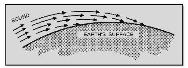
Figure 1-16 Refraction of sound
