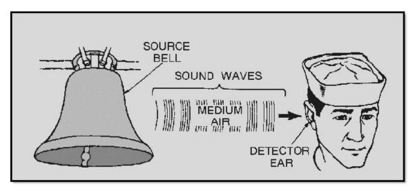
Figure 1-6 The three elements of sound
