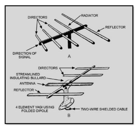
Figure 4-32 Yagi antenna
