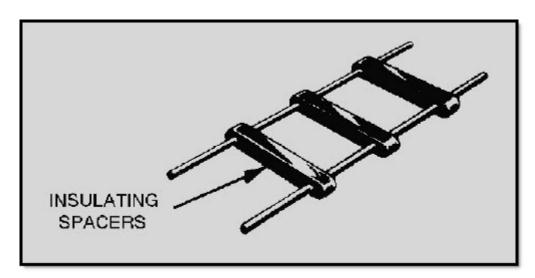
Figure 3-2 Parallel two-wire line
