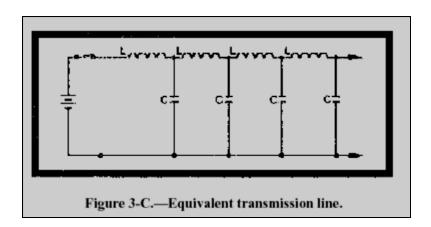
IN ANSWERING QUESTIONS 3-39 AND 3-40, REFER TO FIGURE 3-C. ASSUME THAT THE LINE IS 1,200 FEET LONG. A 150-FOOT SECTION IS MEASURED TO DETERMINE L AND C. THE 150-FOOT SECTION HAS AN INDUCTANCE OF 0.36 MILLIHENRIES AND A CAPACITANCE OF 1,000 PICOFARADS.
