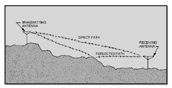
Figure 2-13 Space wave propagation
