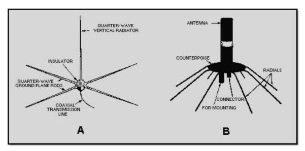
Figure 4-41 Ground-plane antennas
