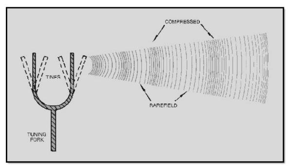
Figure 1-5 Sound propagation by a tuning fork
