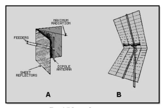
Figure 4-42 Corner-reflector antennas
