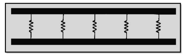
Figure 3-13 Leakage in a transmission line
