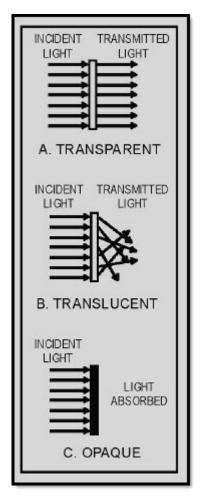
Figure 1-20 Transparent, translucent, and opaque substances
