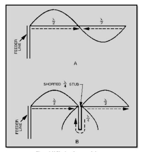
Figure 4-22 Phasing of connected elements
