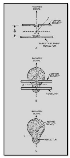
Figure 4-31 Patterns obtained using a reflector with proper spacing
