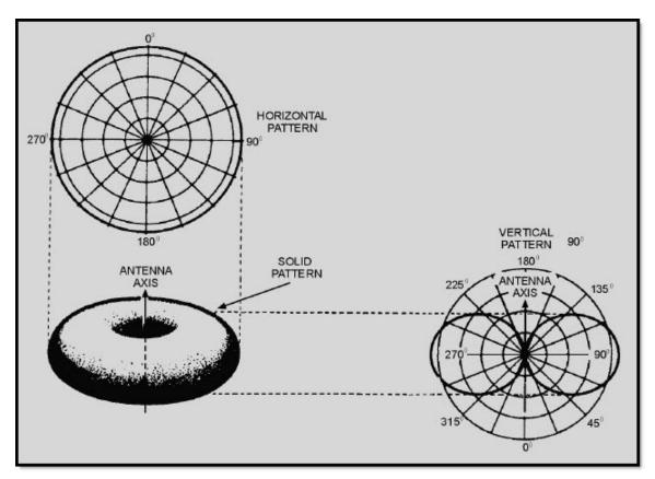
Figure 4-15 Radiation pattern of a dipole
