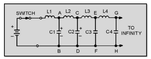
Figure 3-23 Dc applied to an equivalent transmission line
