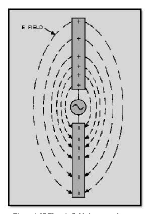
Figure 1-27 Electric fields between elements
