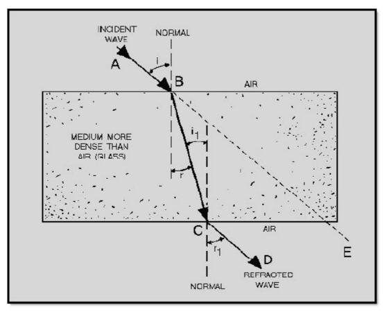
Figure 1-10 Refraction of a wave
