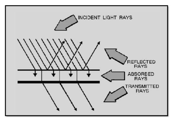
Figure 1-19 Light waves reflected, absorbed, and transmitted
