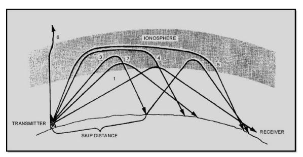
Figure 2-20 Ray paths for a fixed frequency with varying angles of incidence
