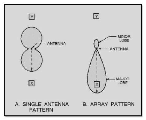
Figure 4-24 Single antenna versus array
