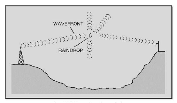
Figure 2-24 Rf energy losses from scattering
