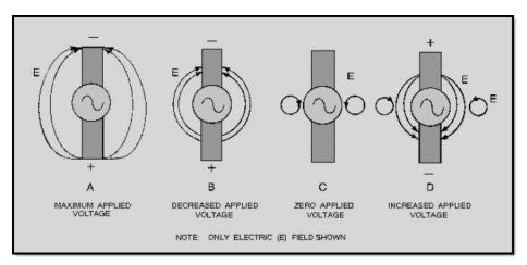
Figure 2-3 Radiation from an antenna
