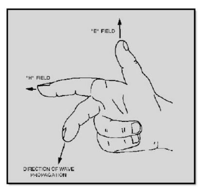
Figure 2-6 Right-hand rule for propagation
