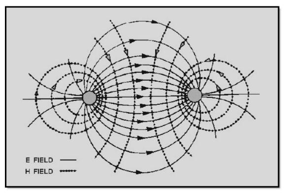
Figure 3-14 Fields between conductors
