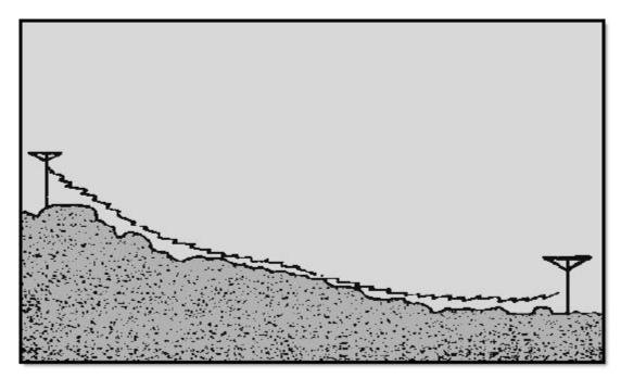
Figure 2-12 Surface wave propagation
