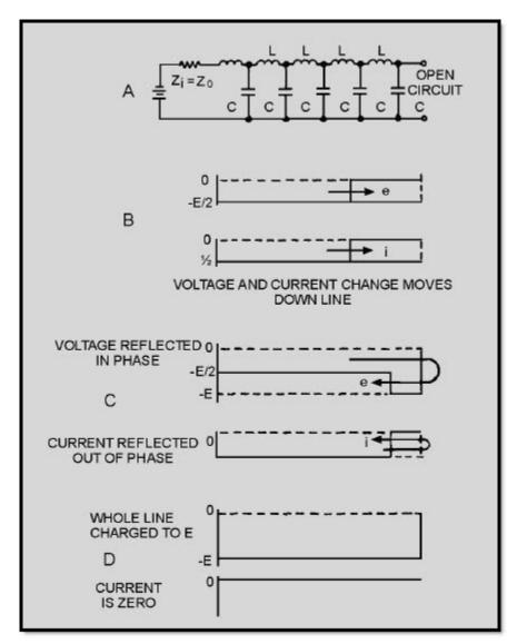
Figure 3-24 Reflection from an open-ended line
