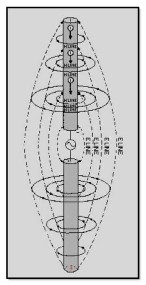
Figure 1-30 Relationship of E-lines, and current flow
