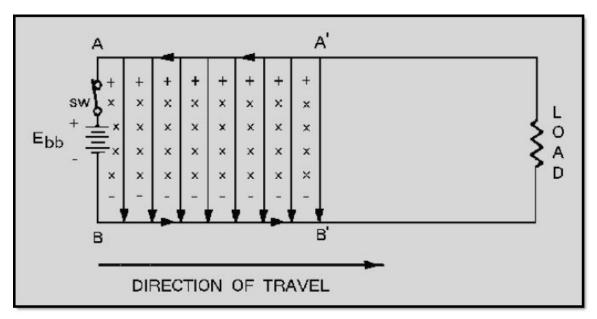
Figure 3-18 Dc voltage applied to a line
