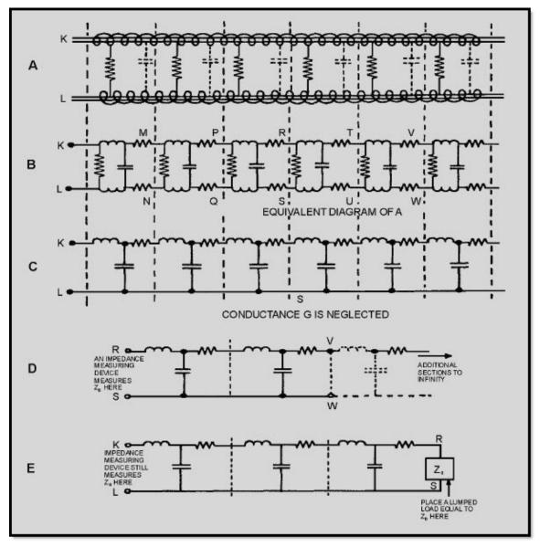
Figure 3-16 Characteristic impedance
