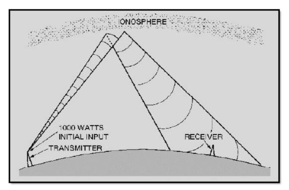
Figure 2-22 Free space loss principle
