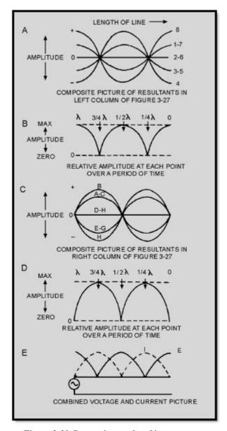
Figure 3-29 Composite results of instantaneous waves
