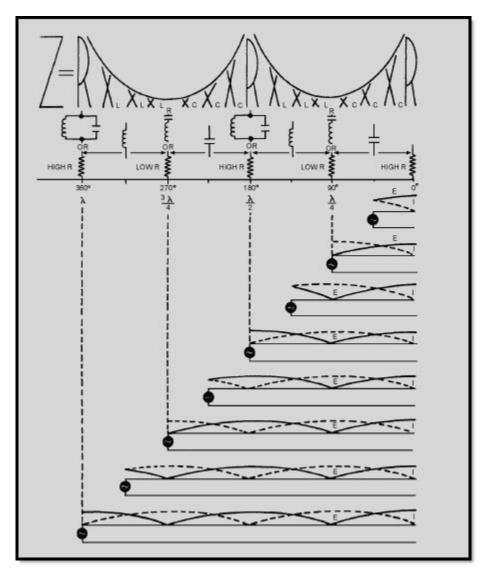
Figure 3-32 Voltage, current, and impedance on open line
