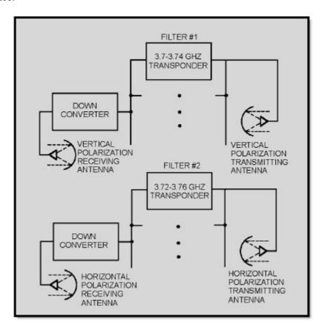
Figure 4-8 Satellite transmissions using polarized radiation
