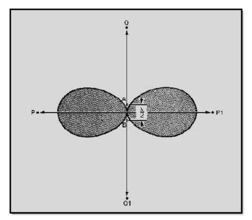
Figure 4-27 Parallel elements in phase
