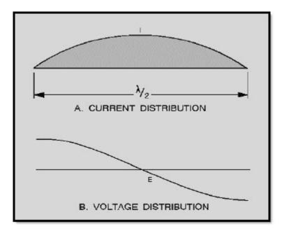
Figure 4-16 Standing waves of current and voltage
