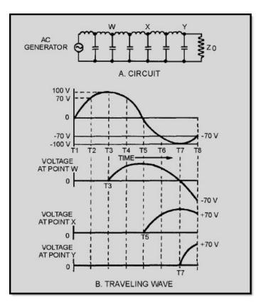
Figure 3-21 Ac applied to an equivalent transmission line
