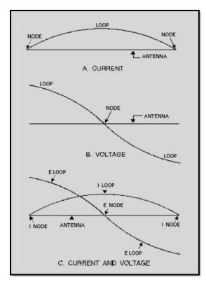
Figure 4-6 Standing waves of voltage and current on an antenna
