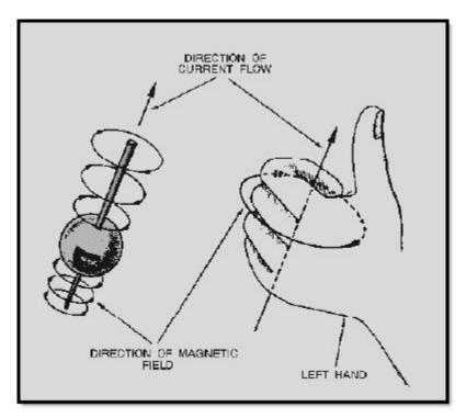
Figure 1-29 Left-hand rule for conducting elements
