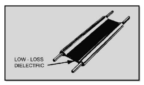
Figure 3-3 Two-wire ribbon type line
