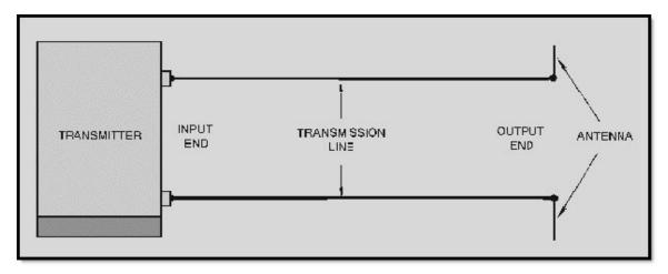
Figure 3-1 Basic transmission line
