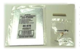
I purchased the sheet metal at the hardware store (Lowe's). It was found in the roofing area and is sold in a plastic bag as "Galvanized Step Flashing." A package of ten 5"x7" pieces cost only \$1.50, so that breaks down to fifteen cents an antenna. As a side bonus, any leftovers can be used to fix your leaky roof. I guess patching roofs and making Patch antennas is all the same thing to the sheet metal.
